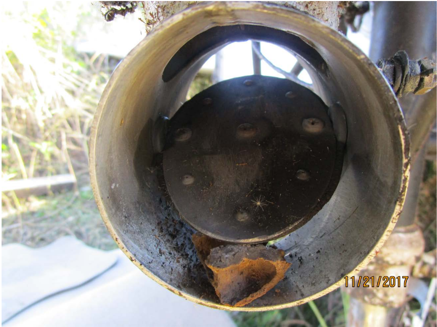
Photo 3 – Mud dauber nest in the carburetor heat intake. (Photo courtesy of the FAA)
