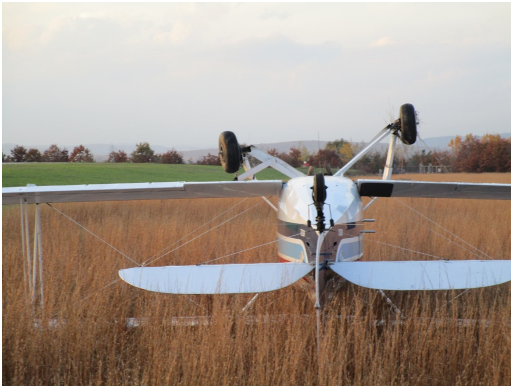
Photo 2 – FAA Digital Photograph. Rear View of the Inverted Airplane. Note the Displaced Right Main Landing Gear.
