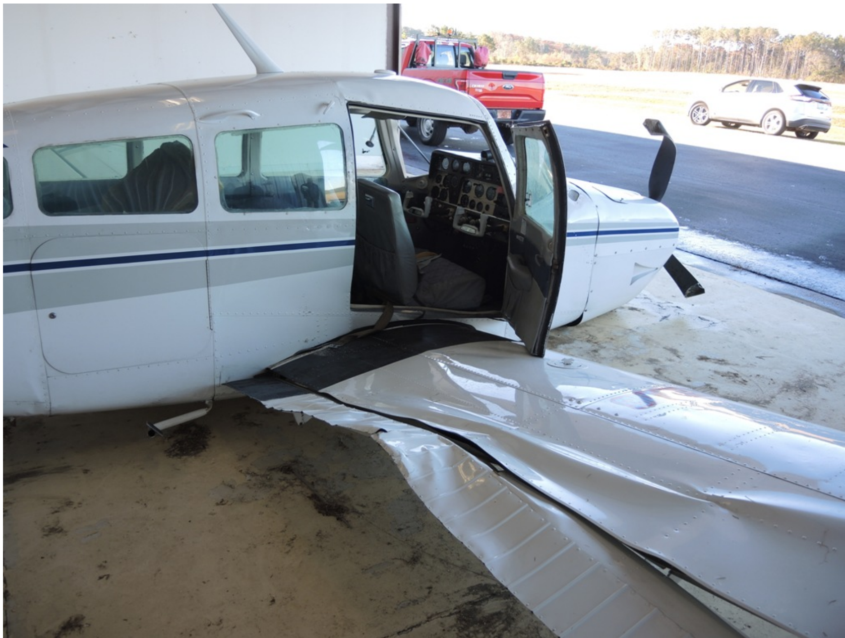
Photo 5 - Textron Aviation Photograph. Close-Up Right Rear Quartering View of the Inboard Section of Right Wing and Section of Fuselage. Note the damage to the wing.
