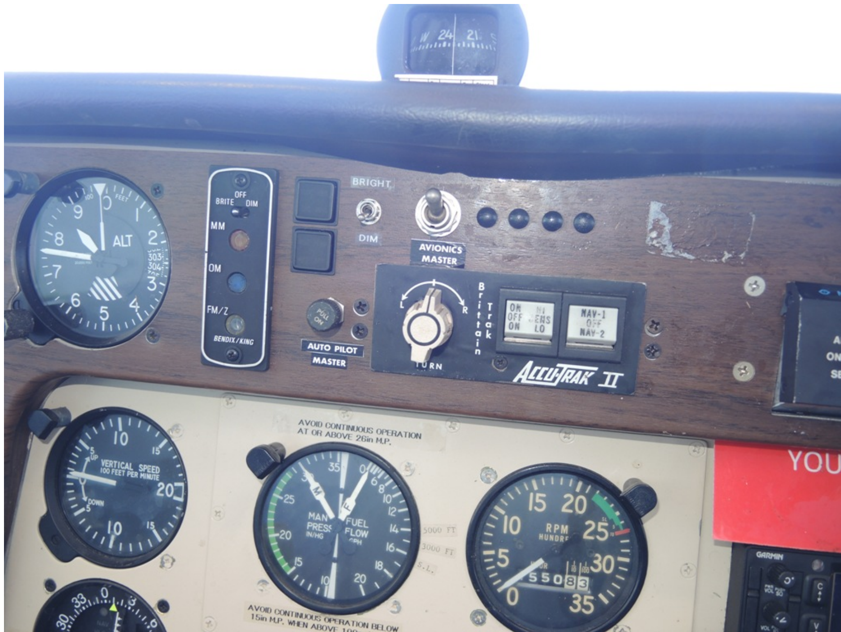
Photo 7 - Textron Aviation Photograph. View of the Instrument Panel Depicting the Avionics Master Switch.
