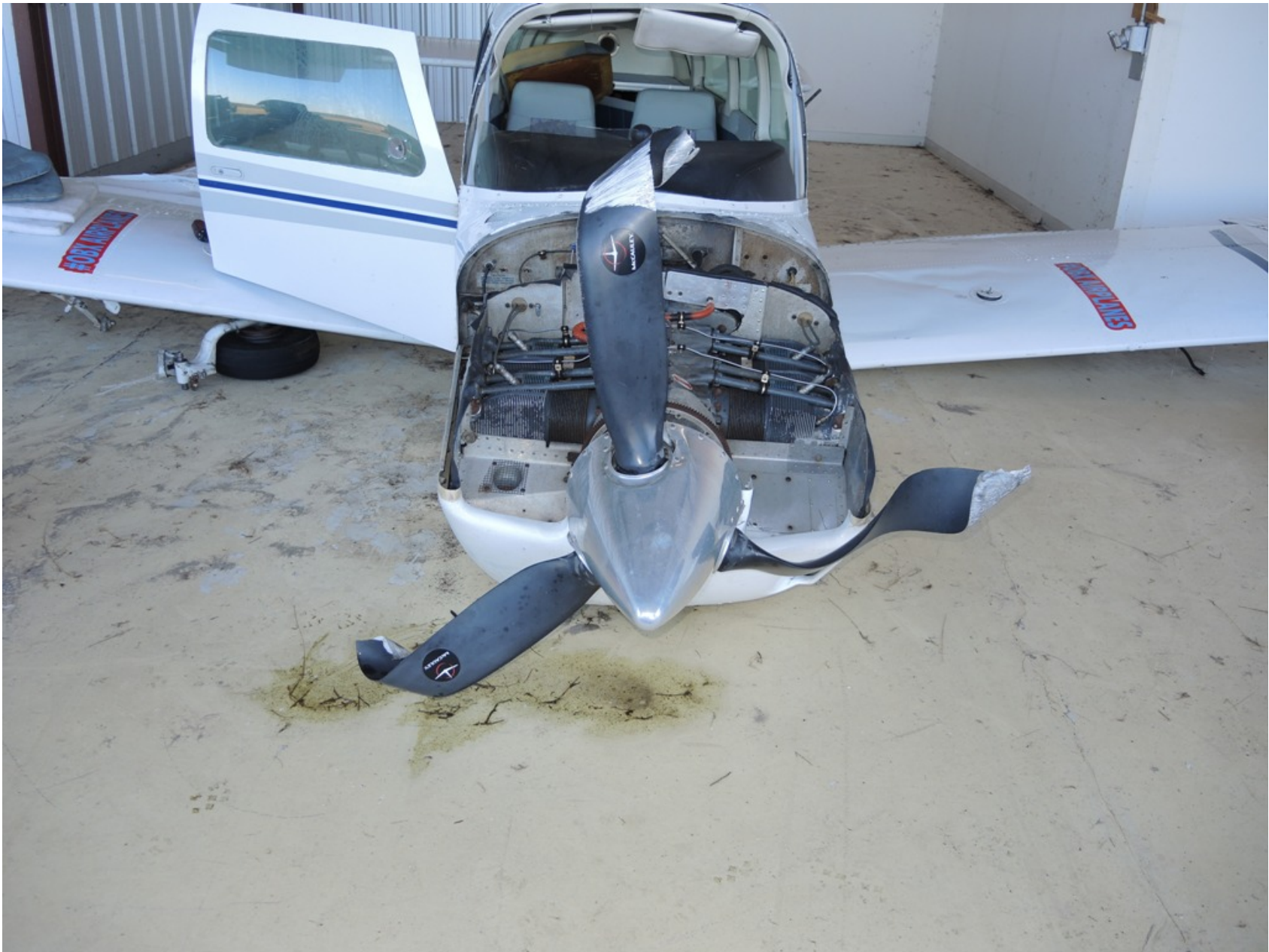
Photo 8 - Textron Aviation Photograph. Front View of the Airplane Following Recovery. Note the Propeller Blade Damage.
