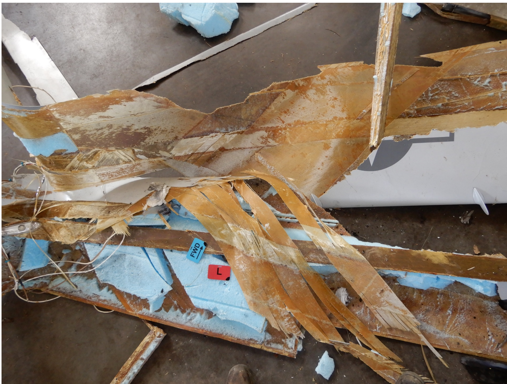
Photo 2 - Overview of Internal Left Wing Structure
