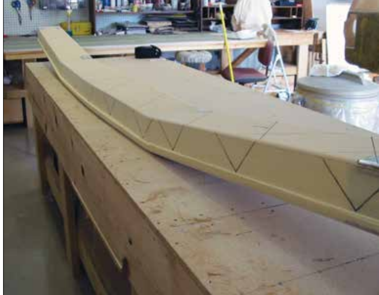
The center section spar ready for fiberglass layups. The black lines are for fiberglass weave orientation reference.
