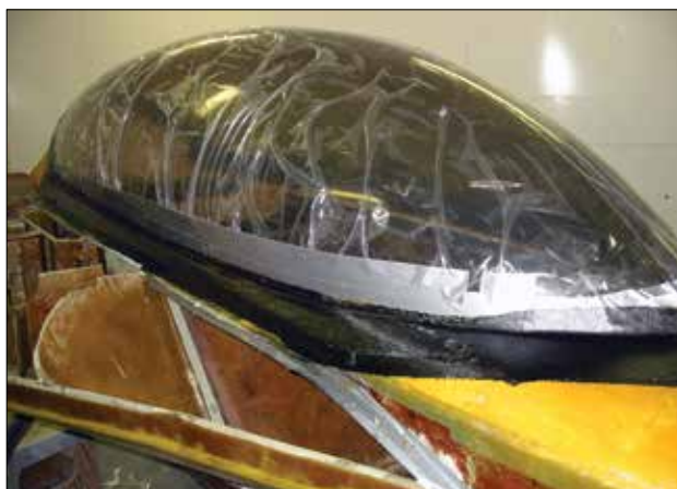
Canopy prior to being cut off. Yep, it's bedded in carbon fiber. Most of the airplane is constructed with E-Z Poxi.
