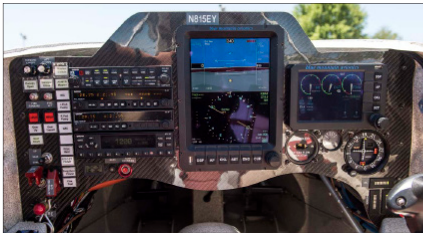
(Left) The panel includes a Blue Mountain EFIS, Garmin SL30 and SL40 radios, GTX 327 transponder, but no autopilot. (Right) Mounted in the forward cockpit in front of the rudder pedals, the fire bottle holds 10 pounds of halon for the engine compartment and is segregated into two sections. The power board includes 12- and 24-volt circuit breakers.
