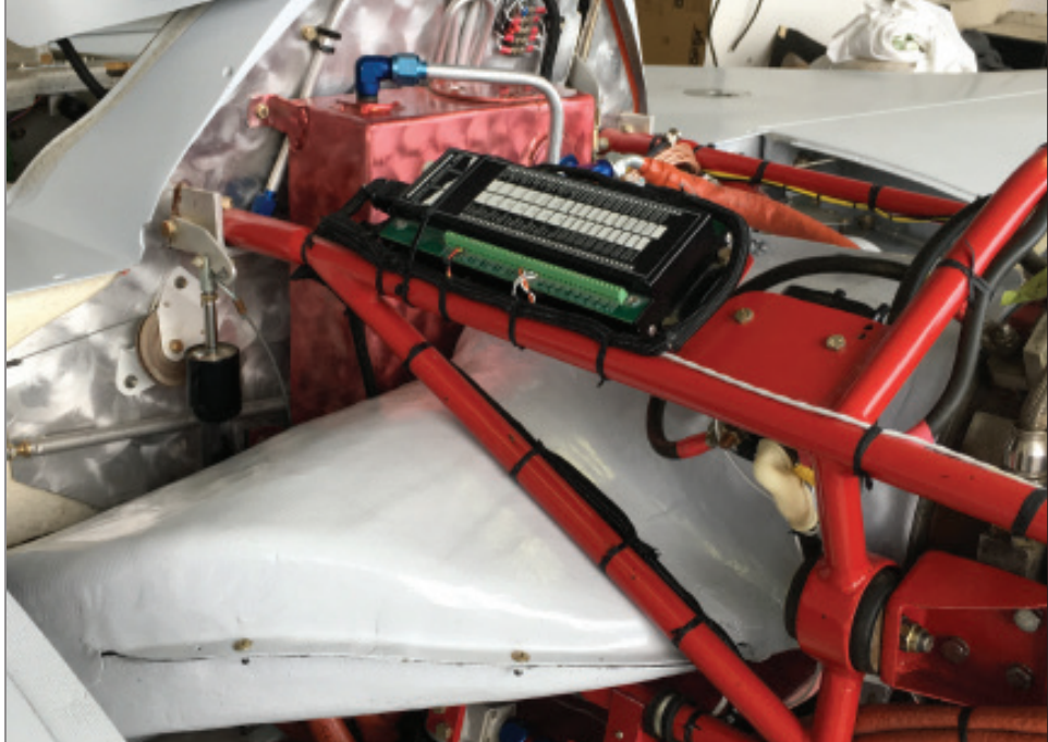
The large red tank on the firewall is the oil tank. The plenum extends from the intake scoops and bends to get air into the engine.
