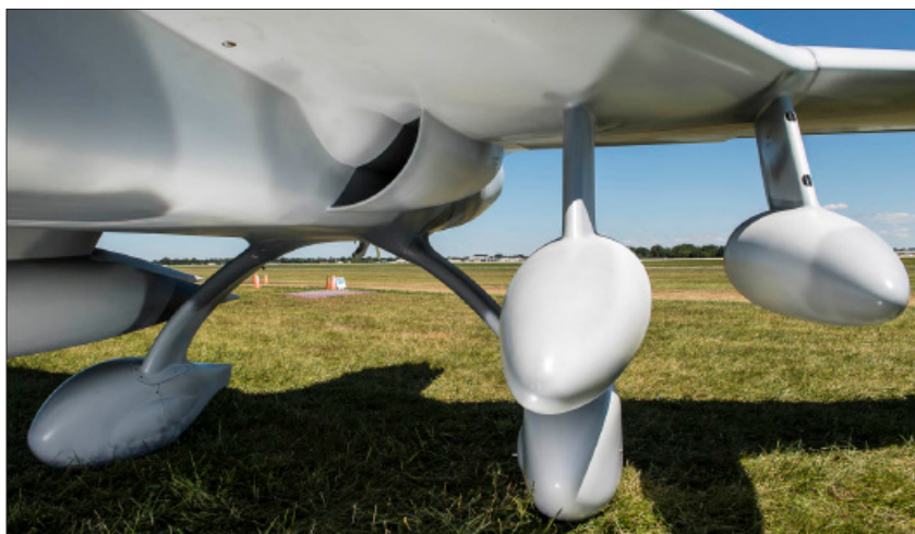
The inboard pods are for fuel, and the outboards are for baggage. Each one is 5 feet long and 1 foot in diameter. The intake scoop provides air to the engine.
