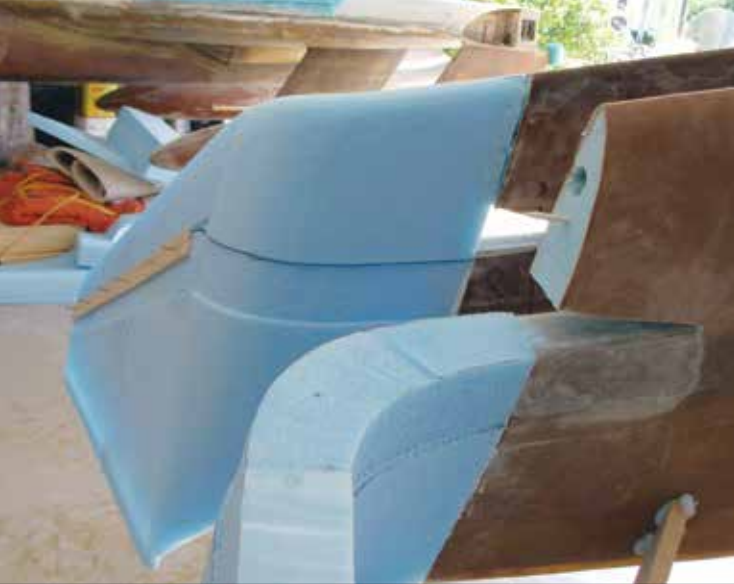
The front half of the winglet in the foreground has been cut off to allow the wing spar to be extended into the winglet.
