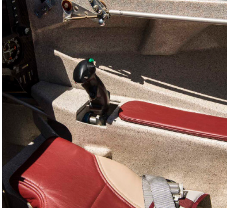
The strakes provide additional storage and a bit more elbow room in the forward cockpit.
