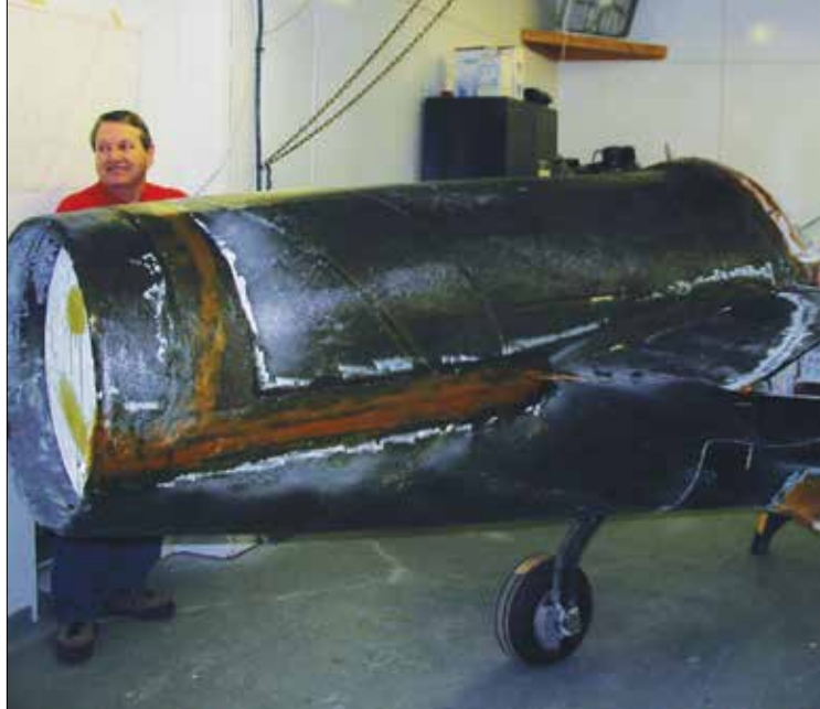
Robert standing behind the finished carbon fiber cowling—all 5 feet of it.
