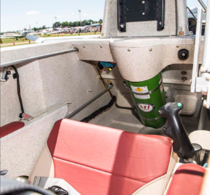
Kevlar oxygen bottle is located behind the front seat. It's good for two people for 7 hours.
