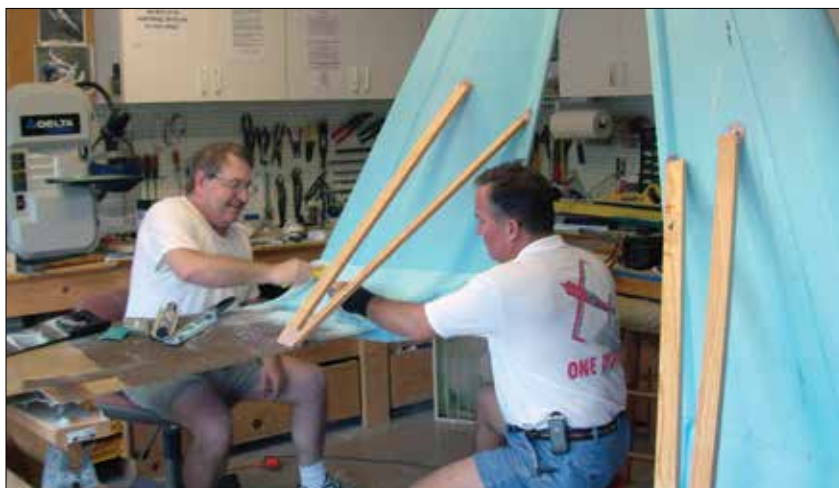
Robert (on the left) and I sanding the blend for the blended winglets. We were both much heavier back then.
