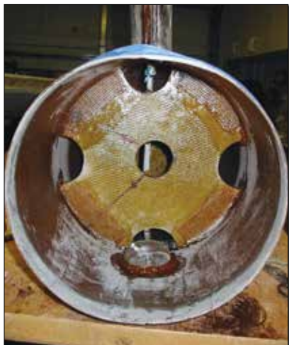
(Left) Looking forward inside one of the fuel pods prior to installing the back half. I put several baffles in to keep fuel slosh to a minimum. (Right) Near the end of primer coats. Notice the unevenness on the pods—not quite finished yet.
