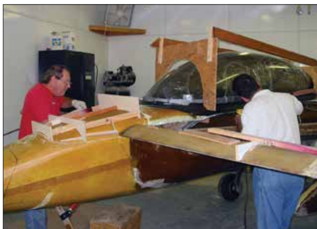
Robert (on the left) and I cutting the canard cover and canopy off to glass the inside of each.
