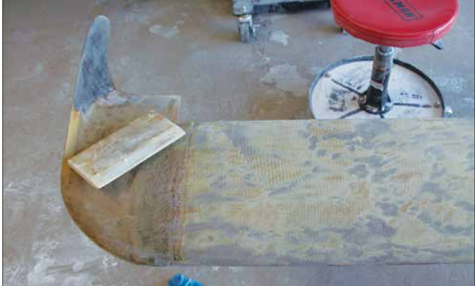
Canard tip. On a lot of the parts for the original Long-EZ, Burt Rutan says, “Sand to a pleasing shape.” Works for me...This is made out of carbon.
