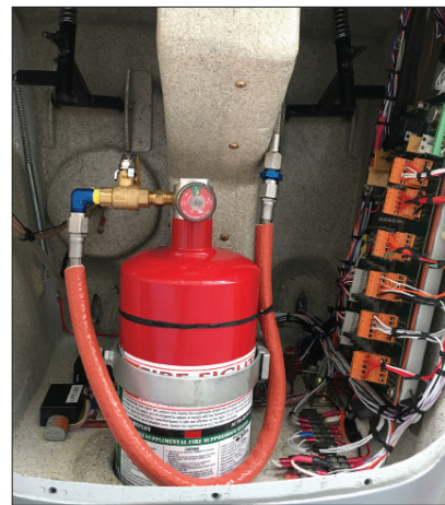
(Left) The panel includes a Blue Mountain EFIS, Garmin SL30 and SL40 radios, GTX 327 transponder, but no autopilot. (Right) Mounted in the forward cockpit in front of the rudder pedals, the fire bottle holds 10 pounds of halon for the engine compartment and is segregated into two sections. The power board includes 12- and 24-volt circuit breakers.
