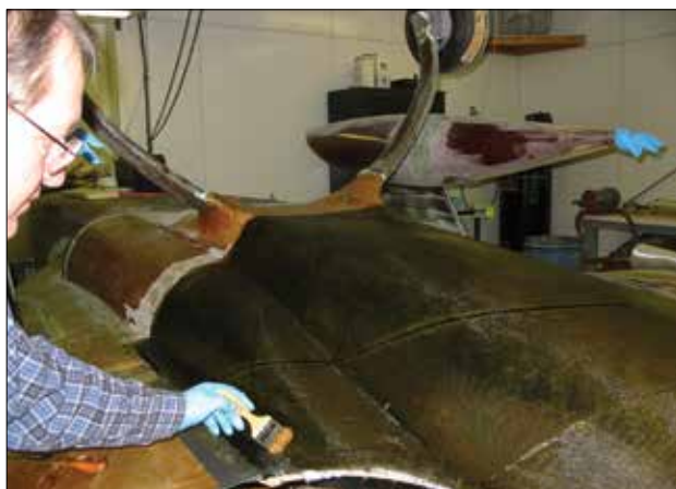
Robert doing a layup on the bottom of the Jet Eze's carbon fiber cowling.
