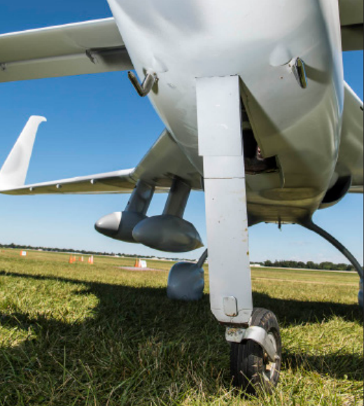
(Left) Like many Rutan canards, the main gear is fixed, but the nose wheel is retractable. (Right) Rear cockpit includes a side stick so the guy (or gal) in back can share the fun.
