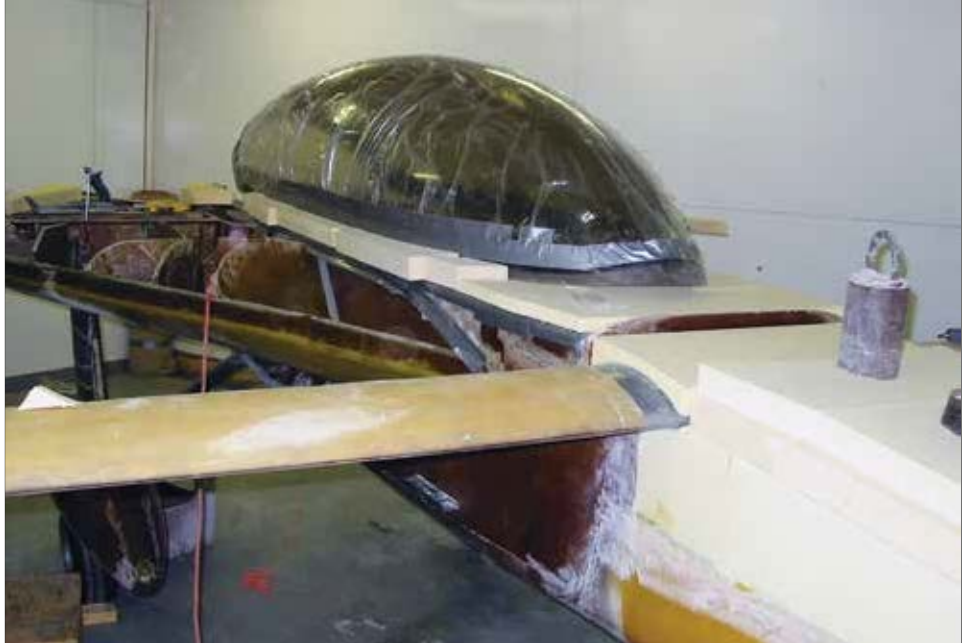
This is how the “pleasing shape” starts out...with foam blocks hot glued together, then you sand off what doesn’t look right.
