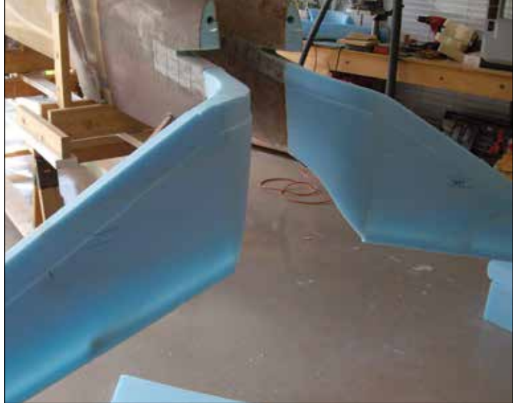
Both winglets ready for the fiberglass layups. Notice the cutouts for overlap onto the main wing spar at the end of the wing.
