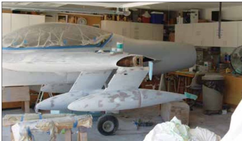
(Left) Looking forward inside one of the fuel pods prior to installing the back half. I put several baffles in to keep fuel slosh to a minimum. (Right) Near the end of primer coats. Notice the unevenness on the pods—not quite finished yet.
