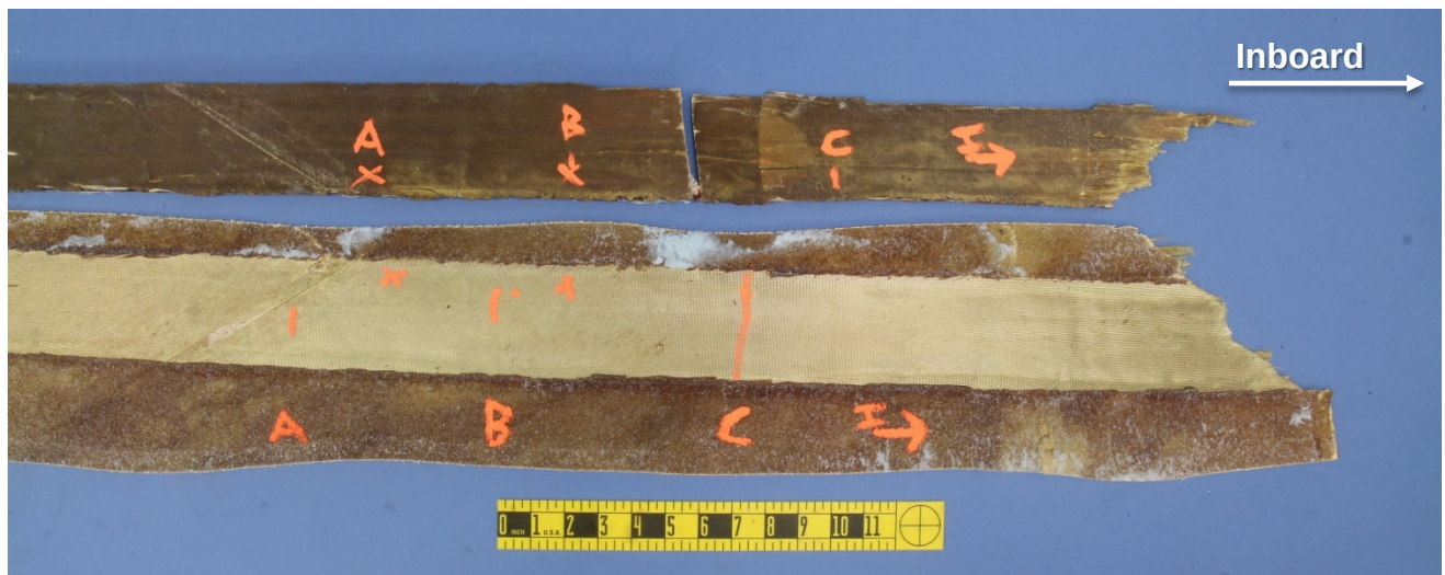
Figure 8 – View of Figure 7, with the spar cap segment removed and inverted in place.
