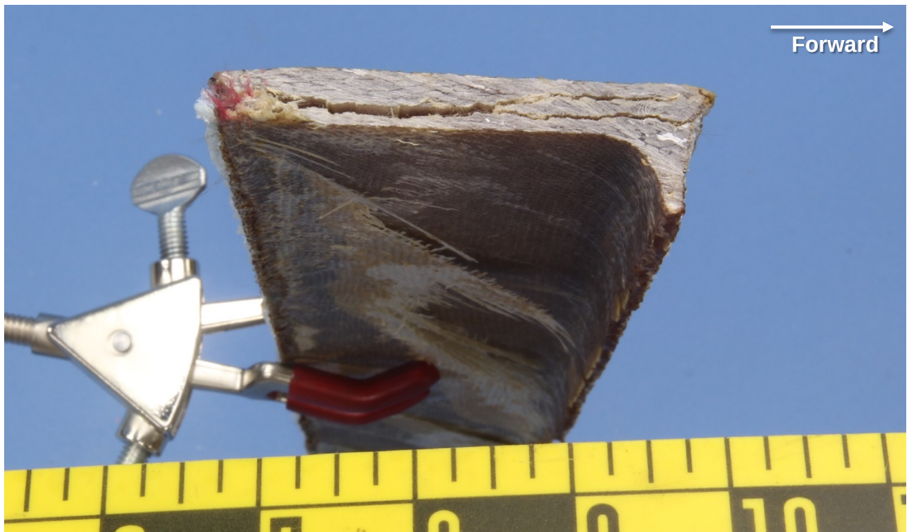
Figure 17 – The A/B section of the upper spar cap, looking outboard at the inboard section.
