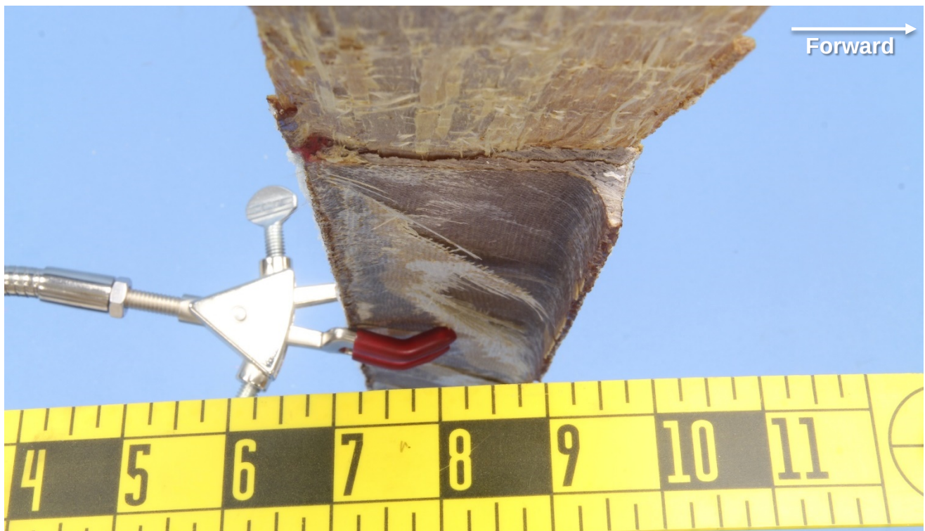
Figure 18 – The A/B section of the upper spar cap, looking outboard with the inboard C section positioned to show the locations of the internal cracks and lower fracture surface.
