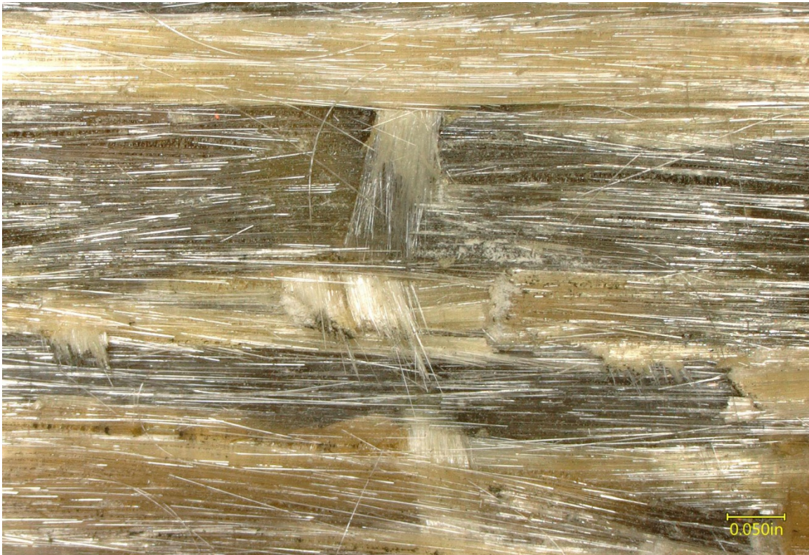
Figure 13 – Spar cap section C lower surface face, fractured fibers and resin fracture features.
