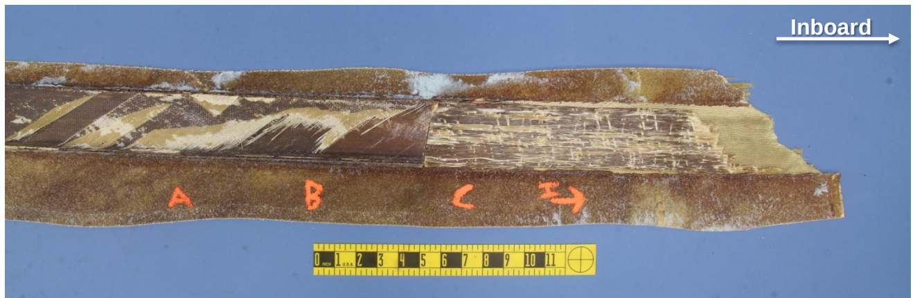
Figure 7 – The inboardmost area of the spar cap and wing skin segments, reassembled.
