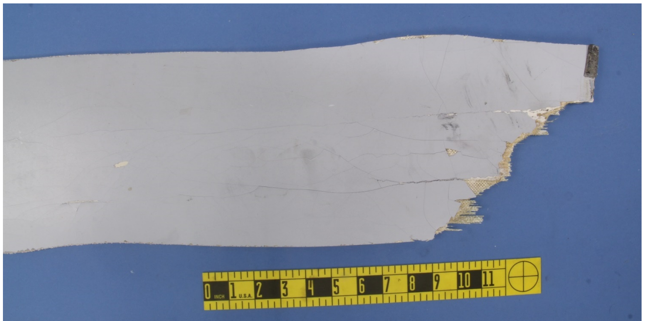
Figure 22 – Closer view of the inboard area of the wing skin section in Figure 21, showing paint cracking and absence adjacent to the fracture.
