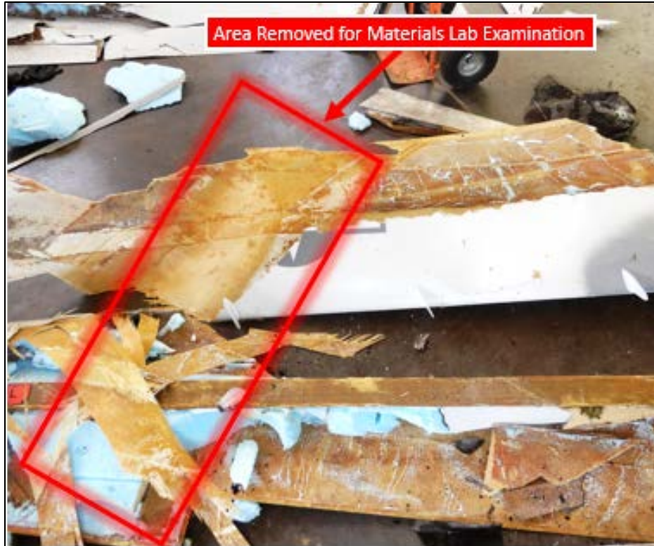
Figure 8: Area Removed for Materials Lab Examination
