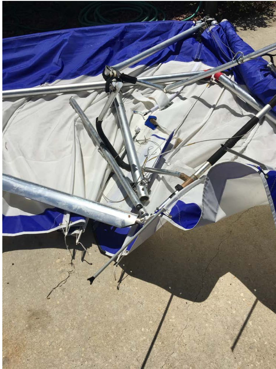
Photo 4 – Close up of damage to wing structure. Note the wing is upside down to facilitate examination. The left side of the photograph is the right wing.
