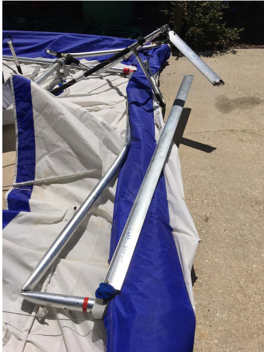
Photo 5 – View of left wing and strut damage.
