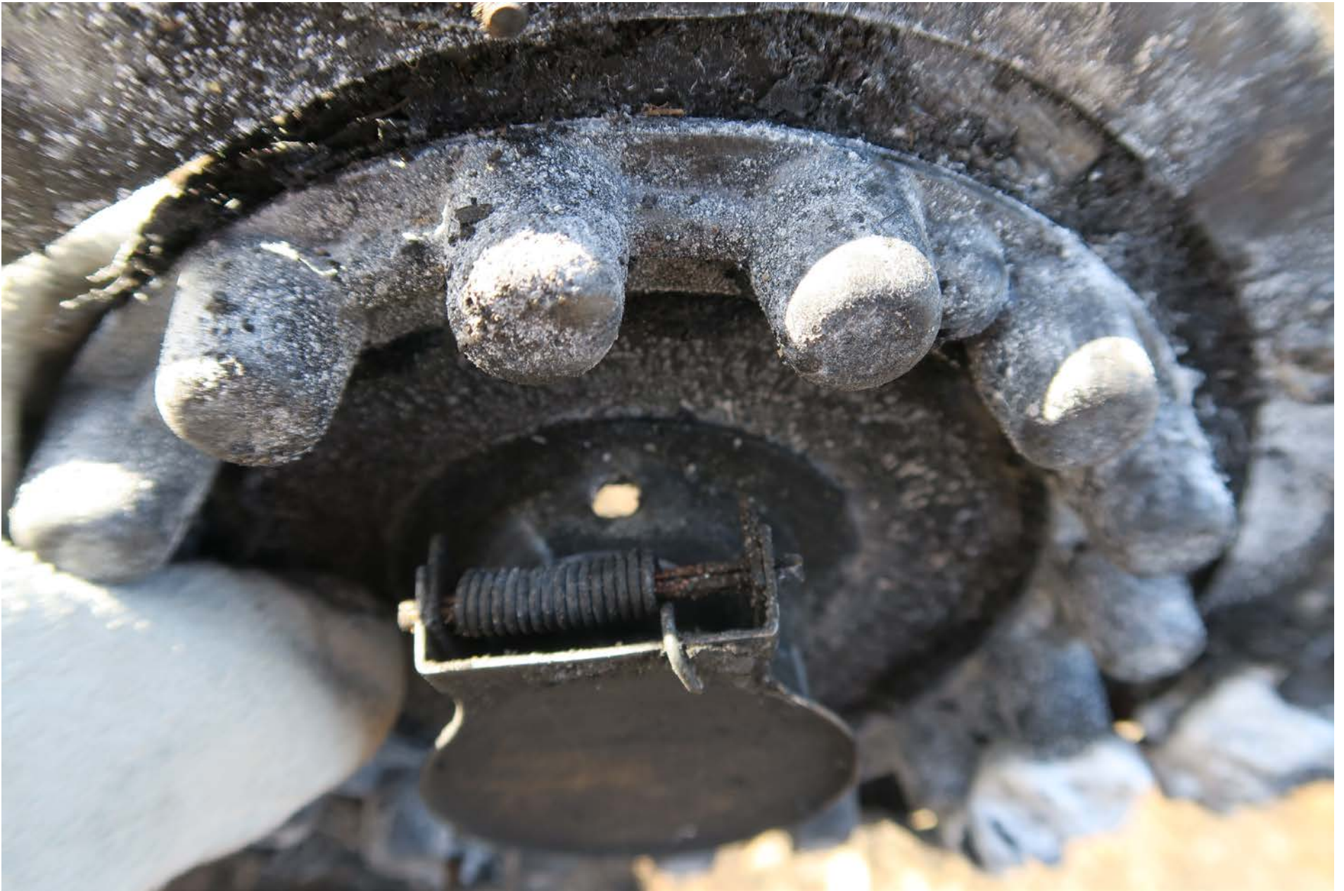
Photo 7 – Bottom view of left side fuel port showing vent hole
