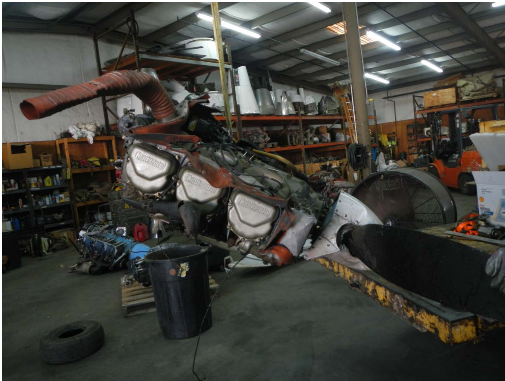
Photo 12 – View of right side of engine showing impact damage
