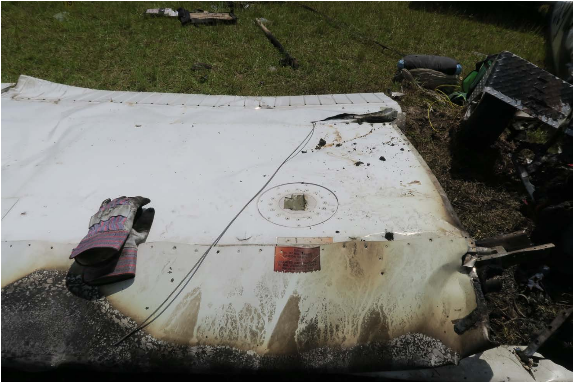
Photo 8 – View of right wing showing tape over right fuel port filler
