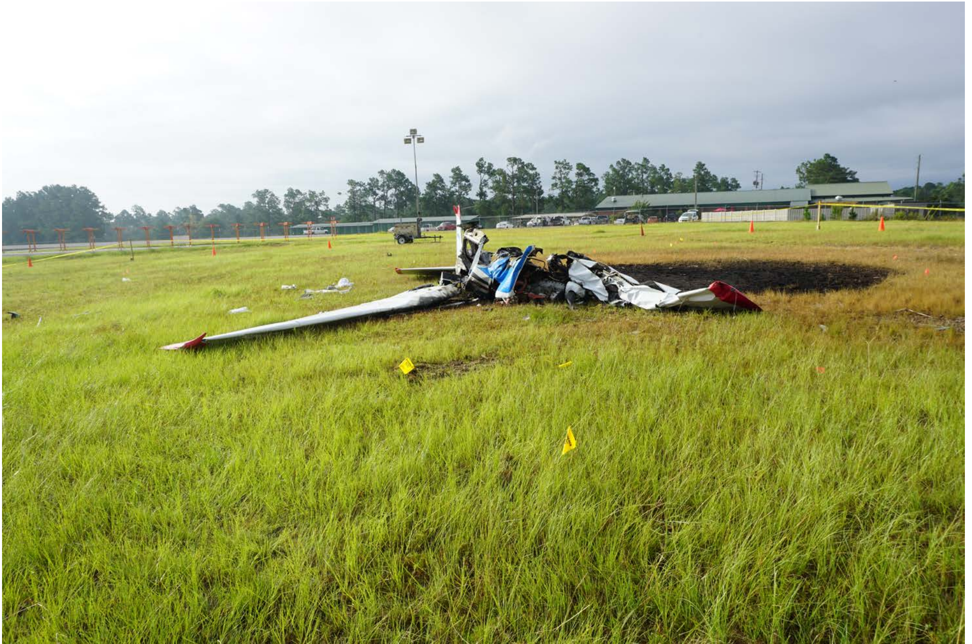
Photo 1 – Forward view of airplane wreckage showing fuselage post-crash fire damage
