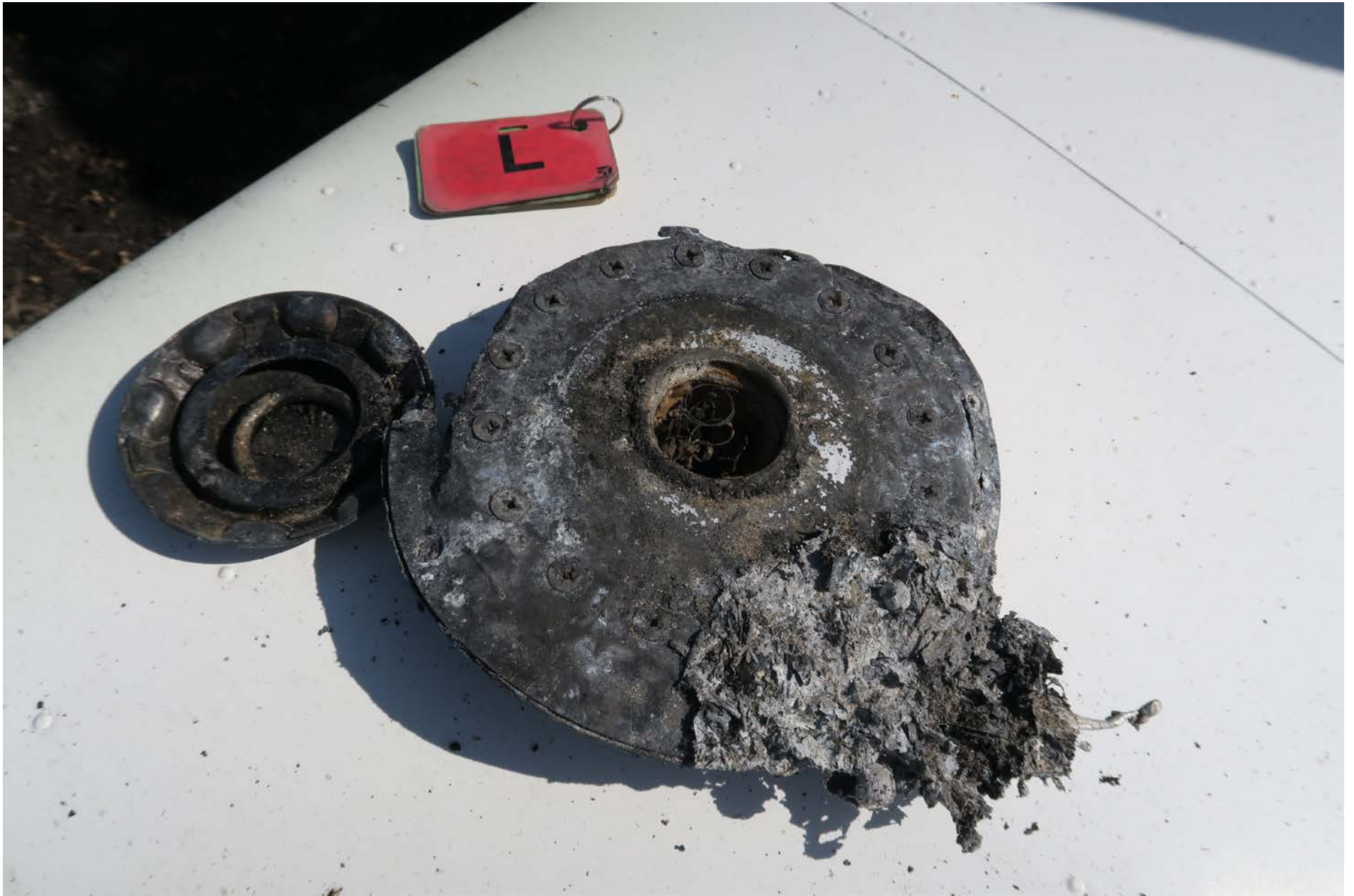
Photo 6 – View of fire damaged left wing vented fuel cap and fuel port (top view)
