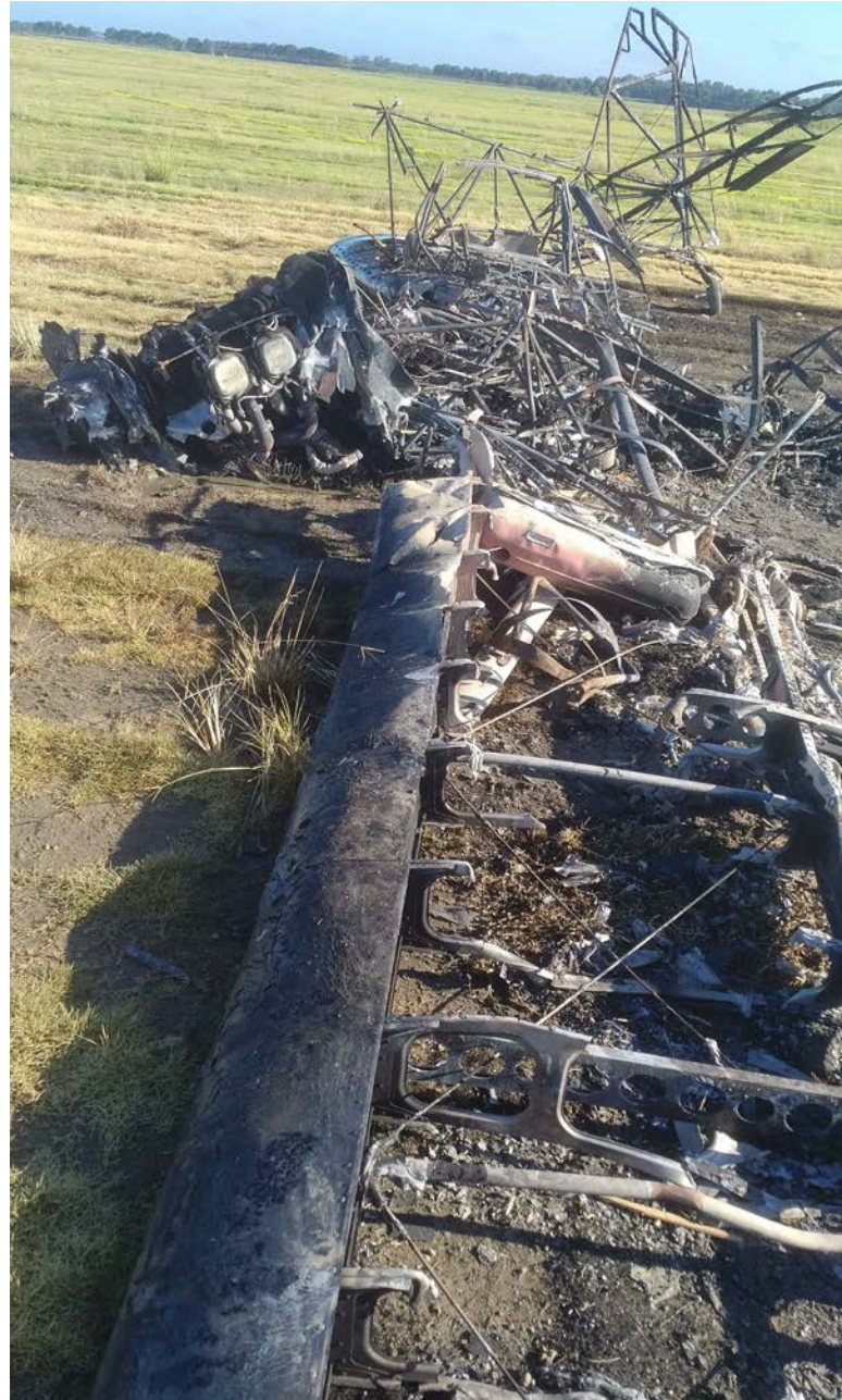
Photo 5 – Photograph of damage to left wing of airplane looking towards engine and fuselage.
