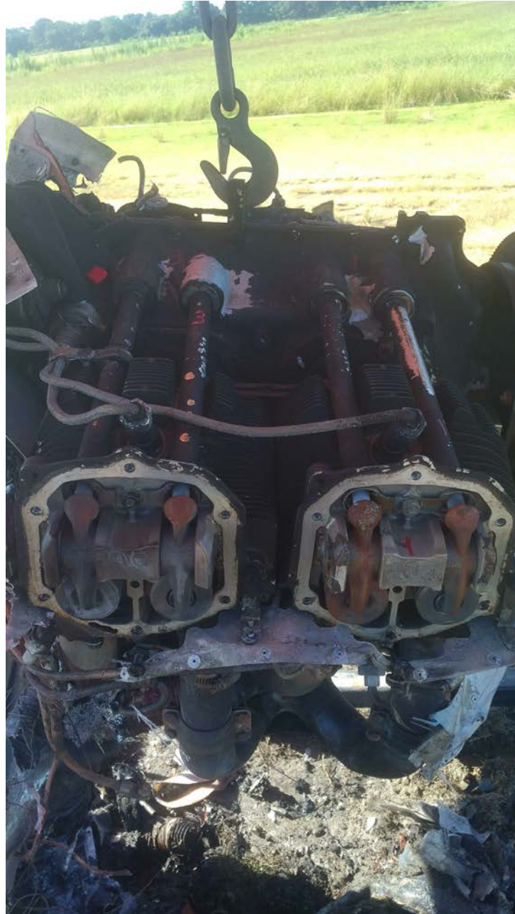
Photo 8 – Cylinders No. 1 and 3 with valve covers removed. Note post-crash fire damage to rocker arms.
