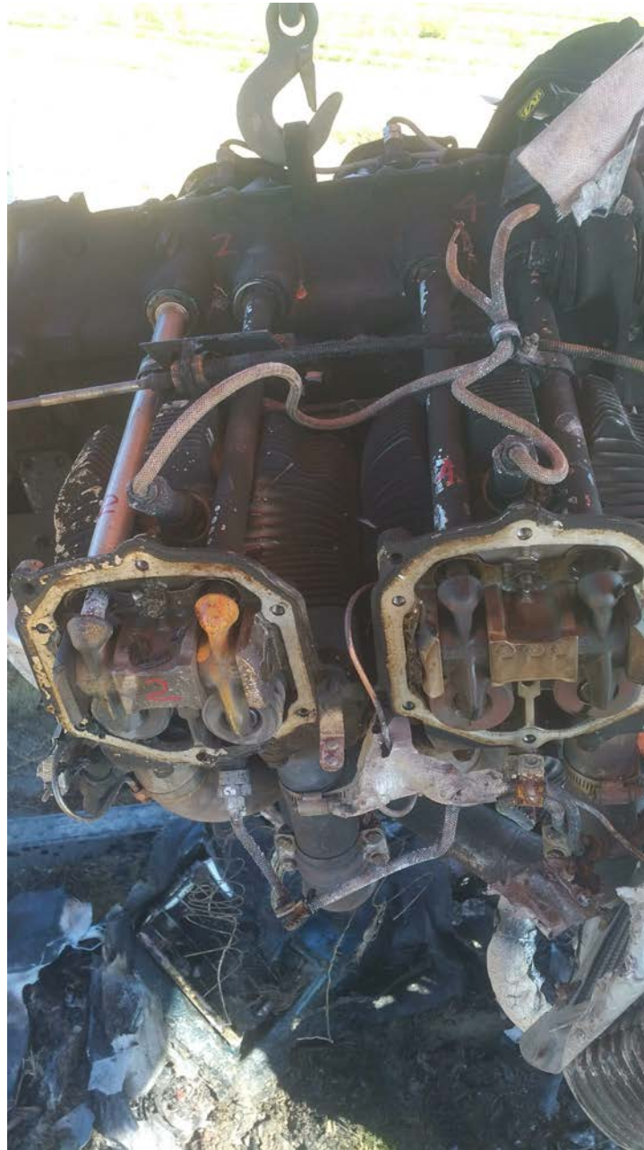
Photo 7 – Cylinders No. 2 and 4 with valve covers removed. Note post-crash fire damage to No. 2.
