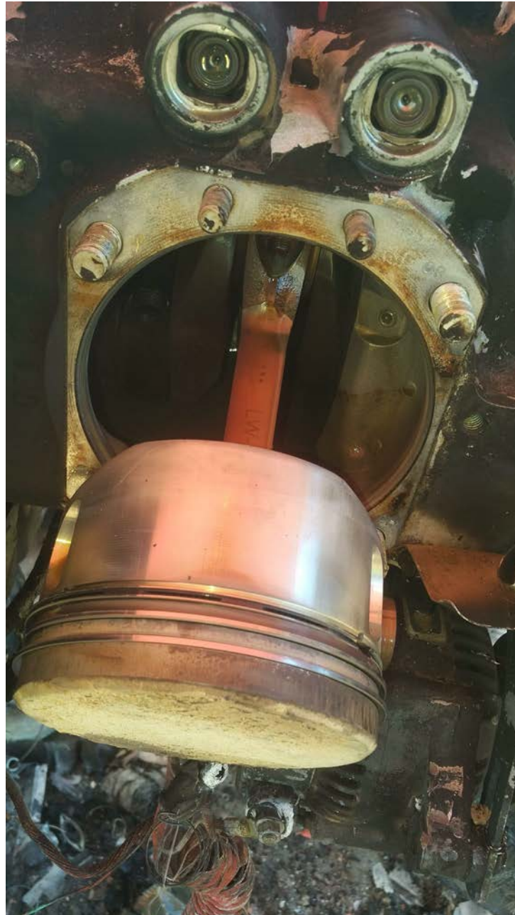
Photo 11 – Photograph of the No. 1 cylinder exhibiting normal wear and free of damage.
