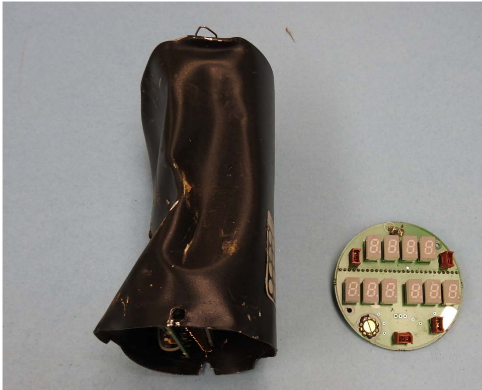
Figure 2. Damaged Shadin Fuel Flow indicator.
