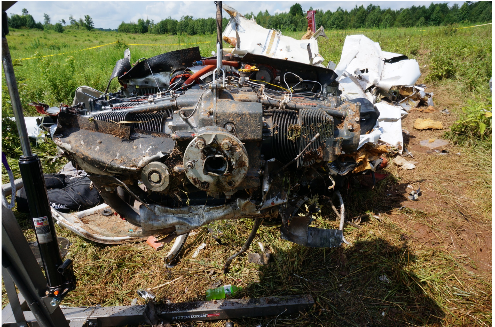
Photo 5 - The engine suspended for examination.
