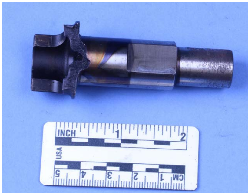
Figure 9: Oil pump drive shaft with fractured yoke.
