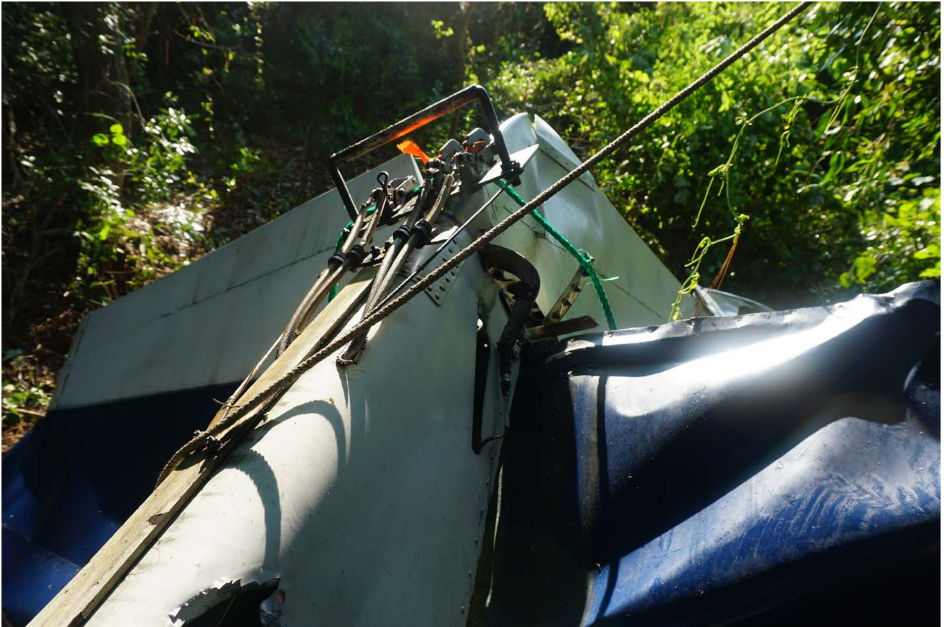
Photo 3 – View of banner tow rope entangled right horizontal stabilizer
