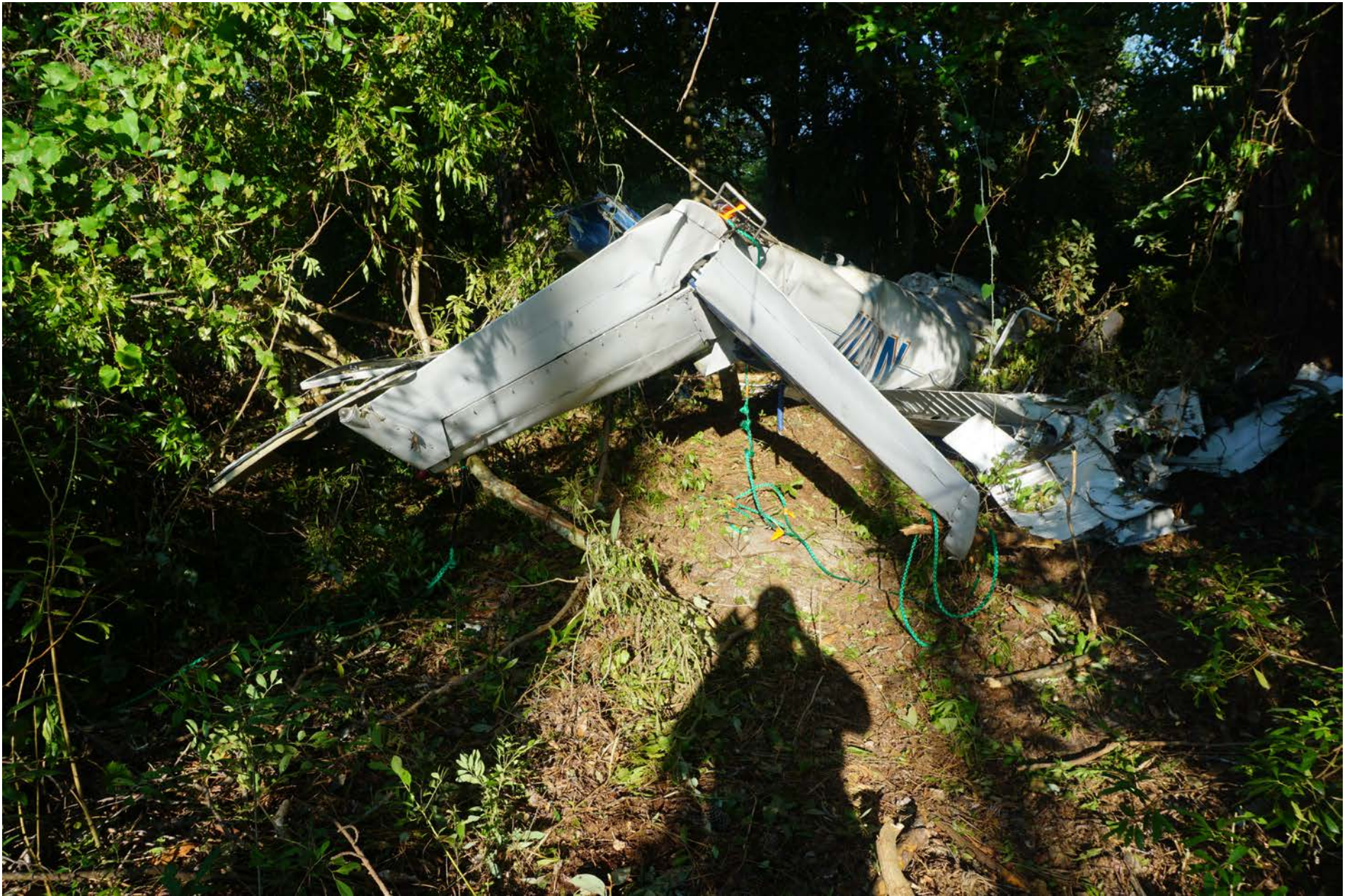
Photo 4 – View of damaged vertical and horizontal stabilizer
