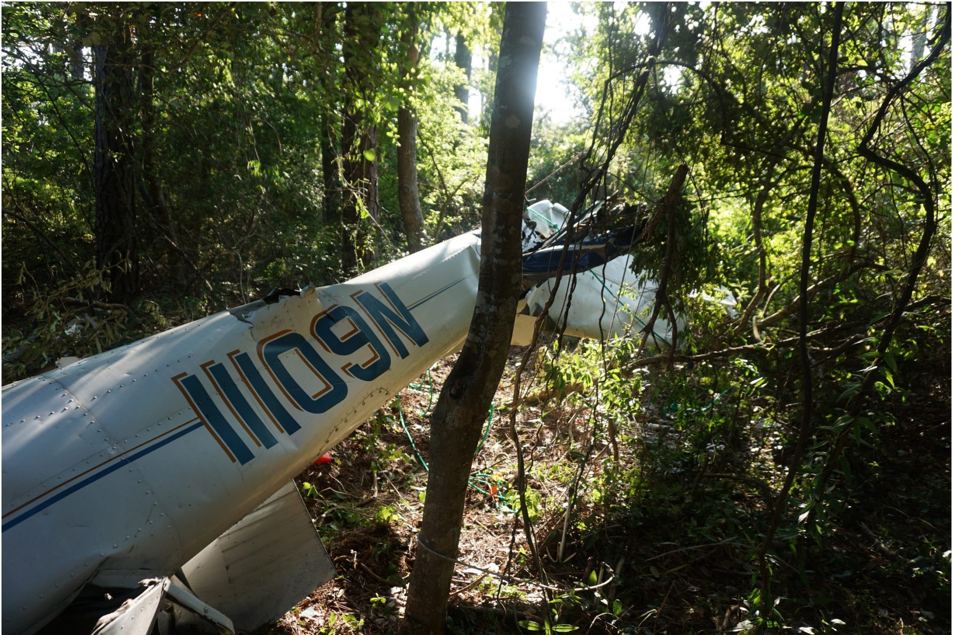
Photo 2 – View of the damaged right side of the empennage
