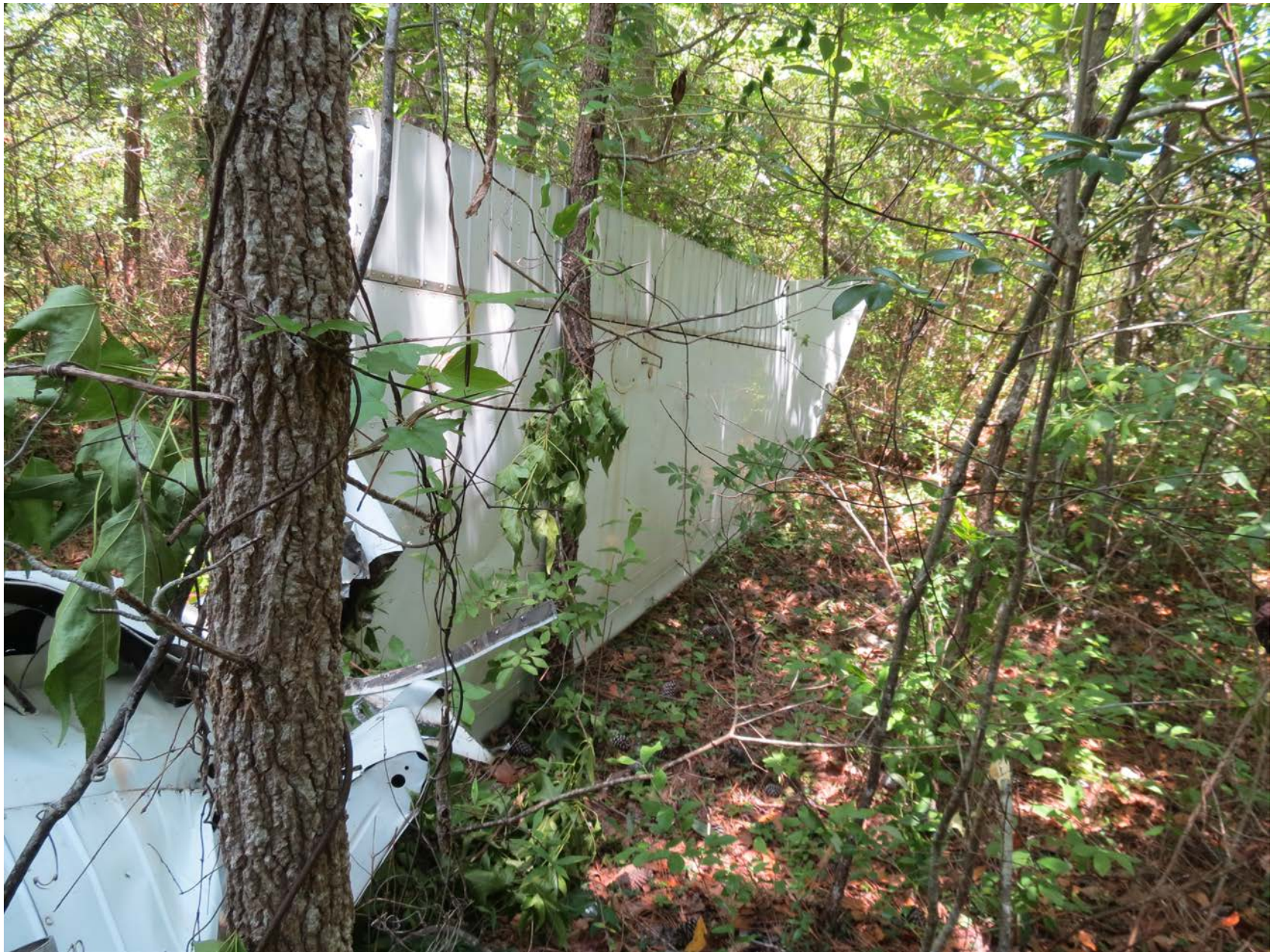
Photo 7 – View of damaged outboard right wing
