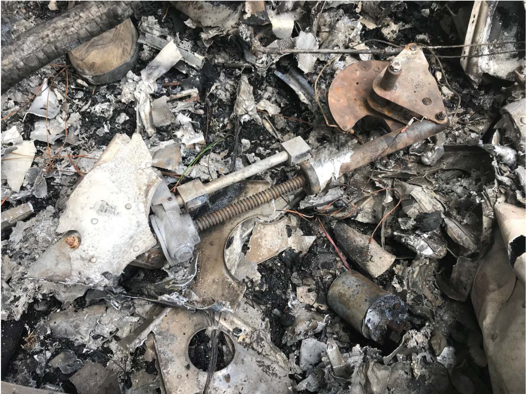
Photo 4 – View of Flap Actuator as Found (FAA)
