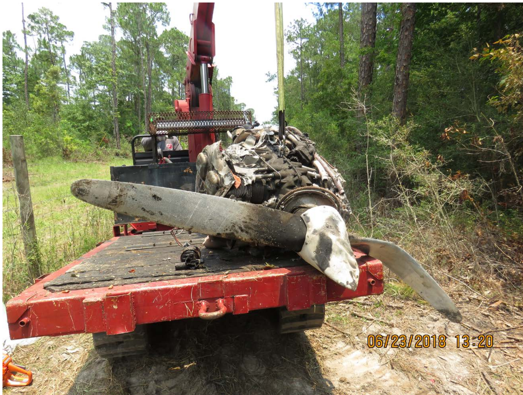
Photo 3 – View of Engine after Recovery (Lycoming)
