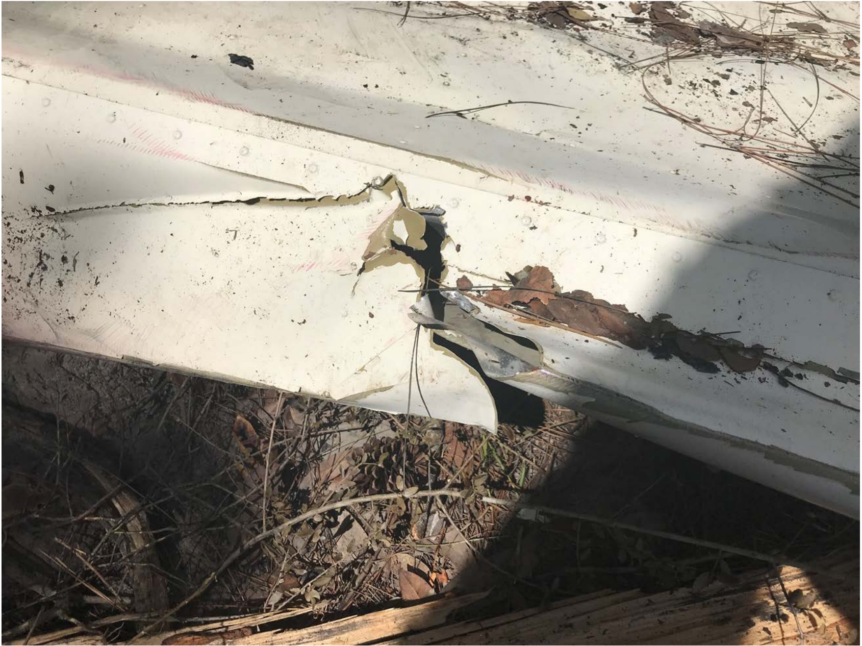
Photo 2 – View of Left Wing Leading Edge as Found (FAA)
