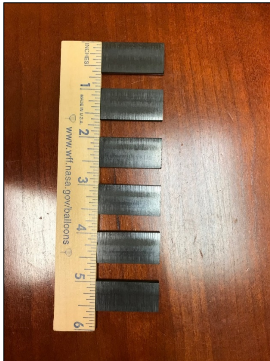
Photo 6: View of vanes removed from vacuum pump
