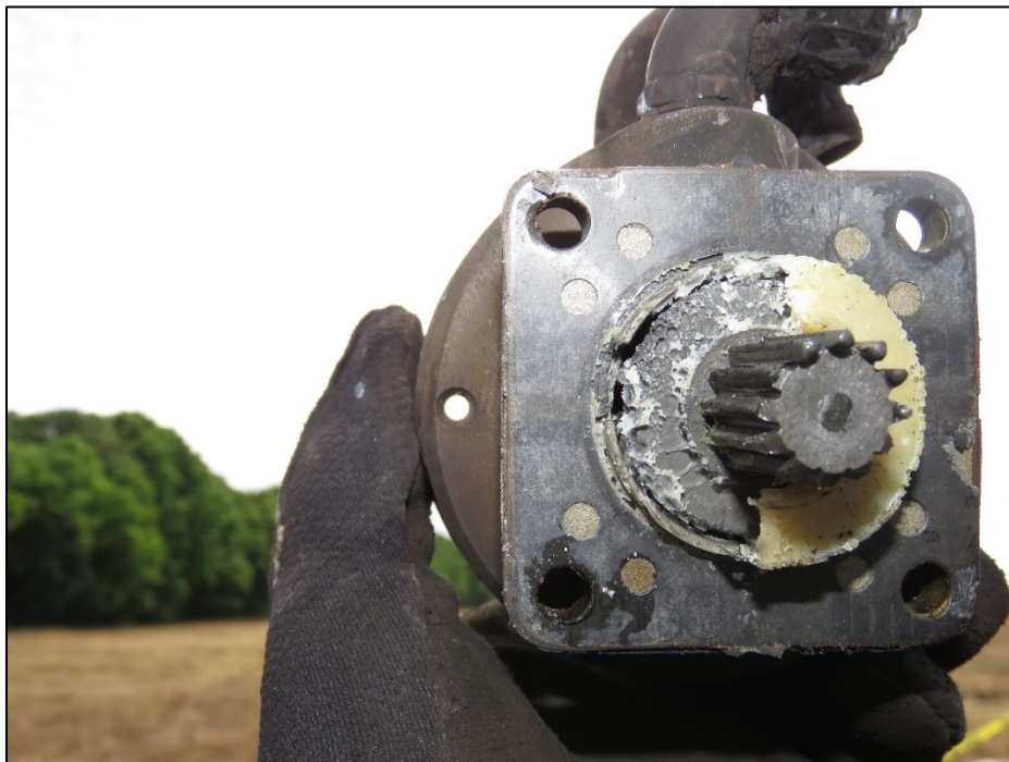
Photo 4: Vacuum Pump Gear Drive.
