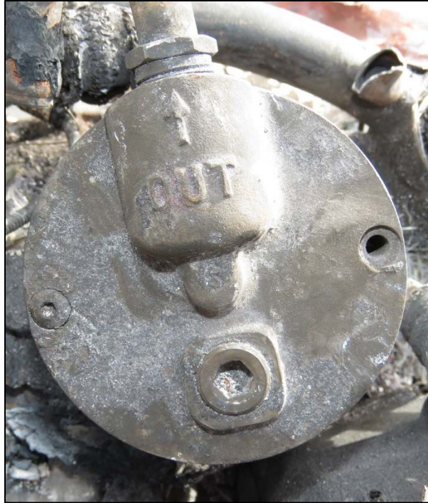
Photo 3: Vacuum Pump attached to the engine. Note the right casing screw was found missing.
