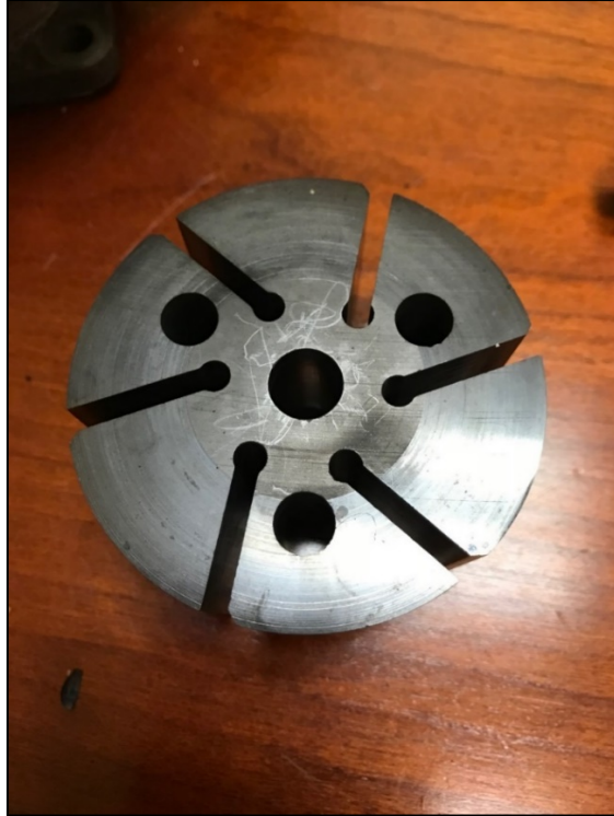
Photo 5: View of Stator from Vacuum Pump
