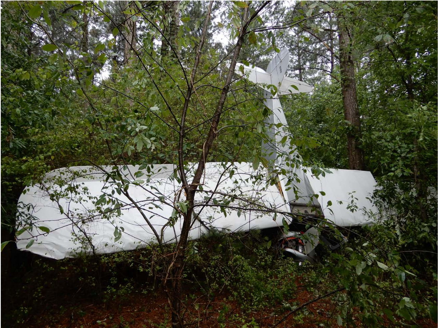
Photo 1 – View of the top of the airplane as it came to rest in a nose low position.
