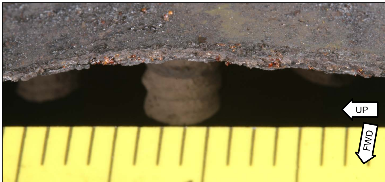
Figure 4. Fracture surface near the middle of the crack in the muffler wall as viewed looking aft.
