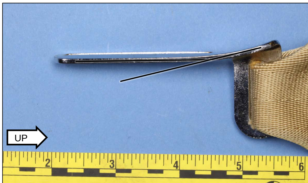
Figure 5. Buckle attachment fitting on the front left shoulder harness strap. The lines indicate the angle of bending.
