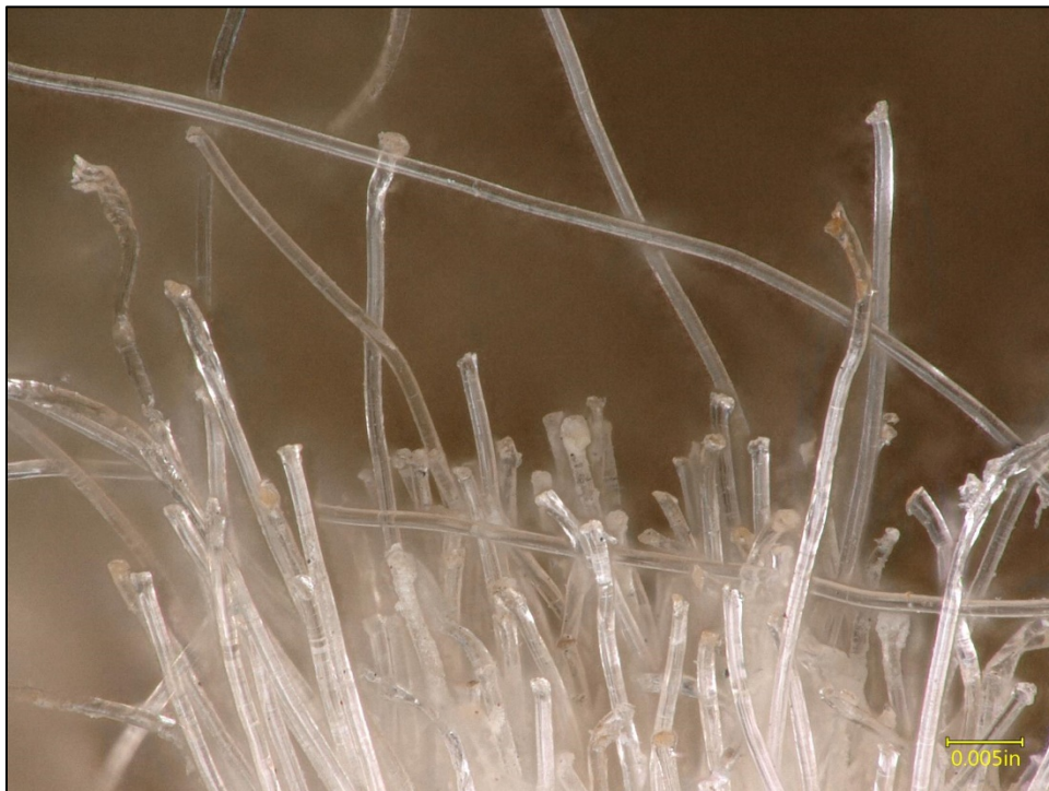
Figure 7. Optical images of typical fractured fibers for the front left lap belt fractures shown in figure 6.
