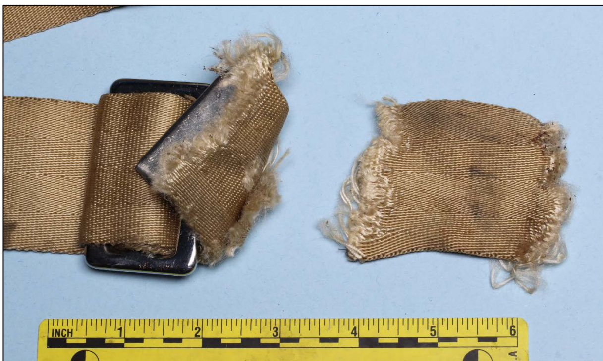
Figure 6. Closer view of fractures at the anchor point for the front left lap belt.
