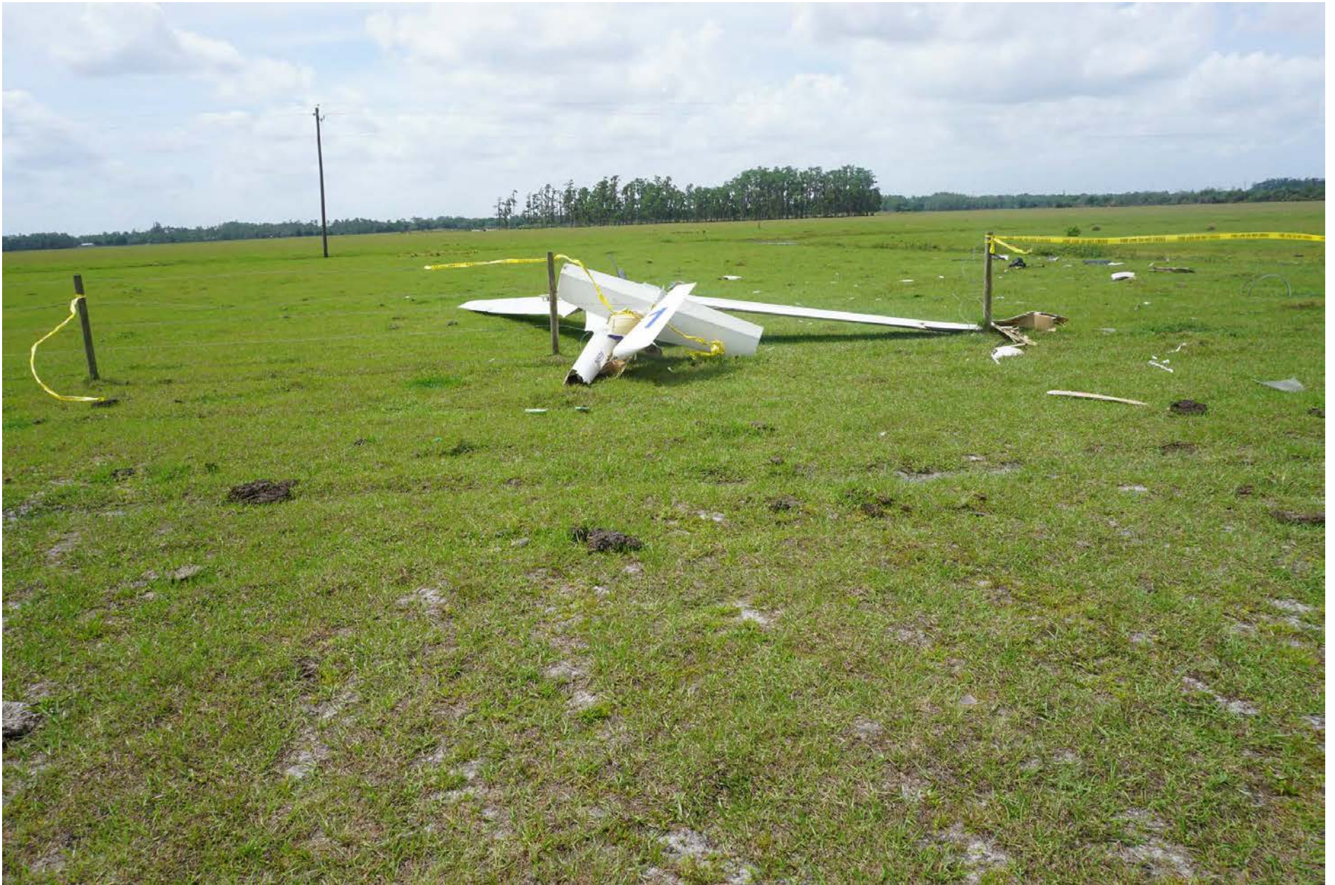
Photo 1 – Aft view of wreckage showing damaged vertical and horizontal stabilizers
