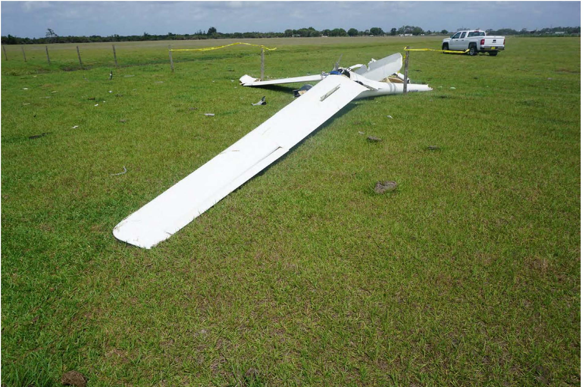
Photo 3 – Left-side view of wreckage showing damaged left wing
