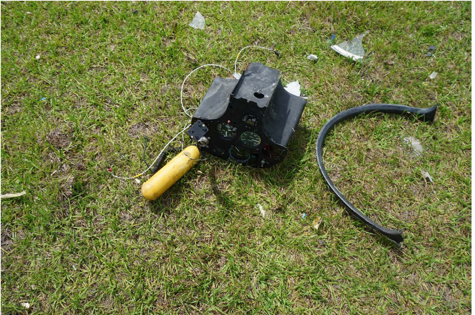
Photo 6 – View of damaged instrument panel within the debris path
