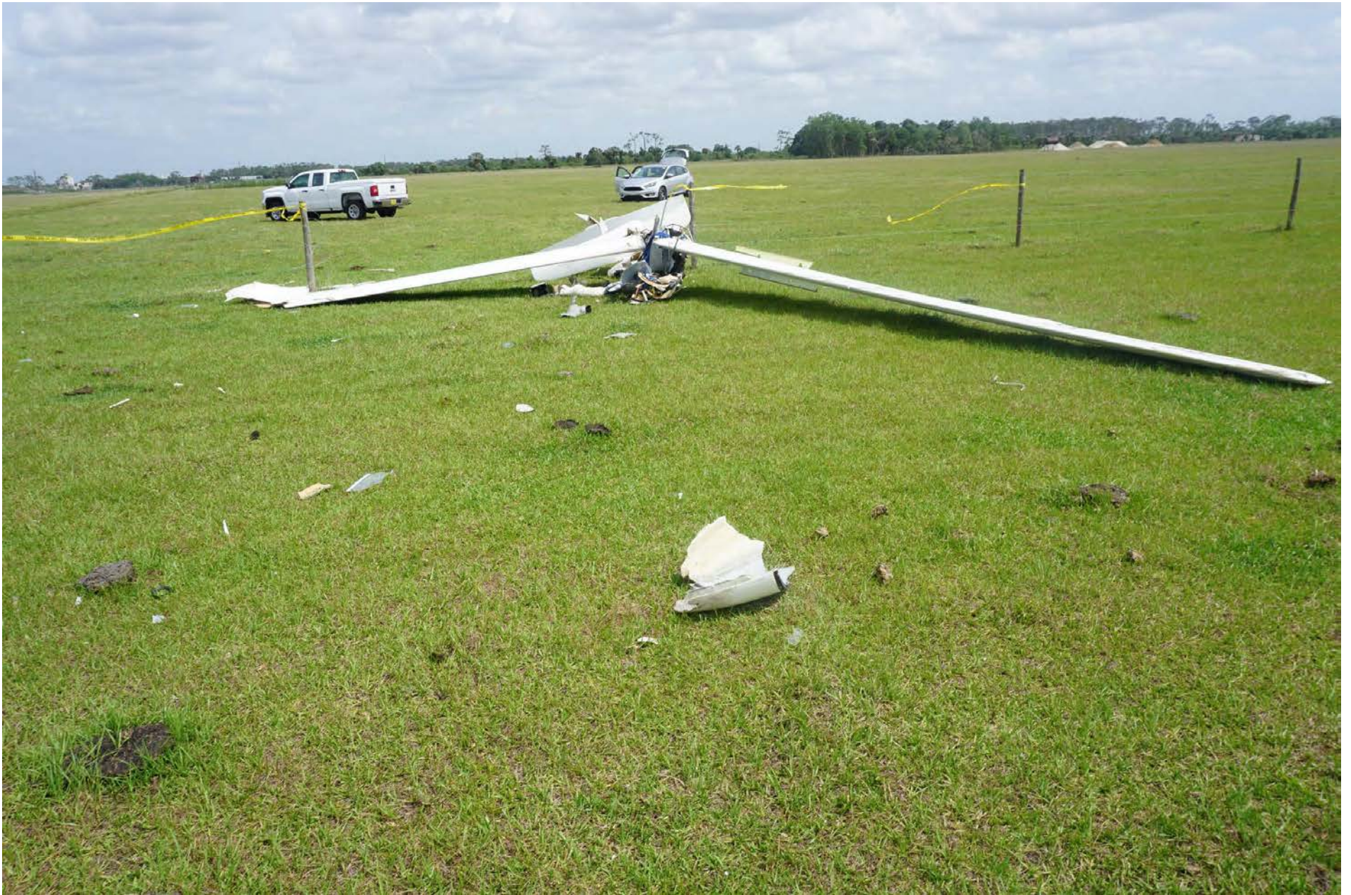
Photo 4 – Front view of wreckage showing the crushed cockpit
