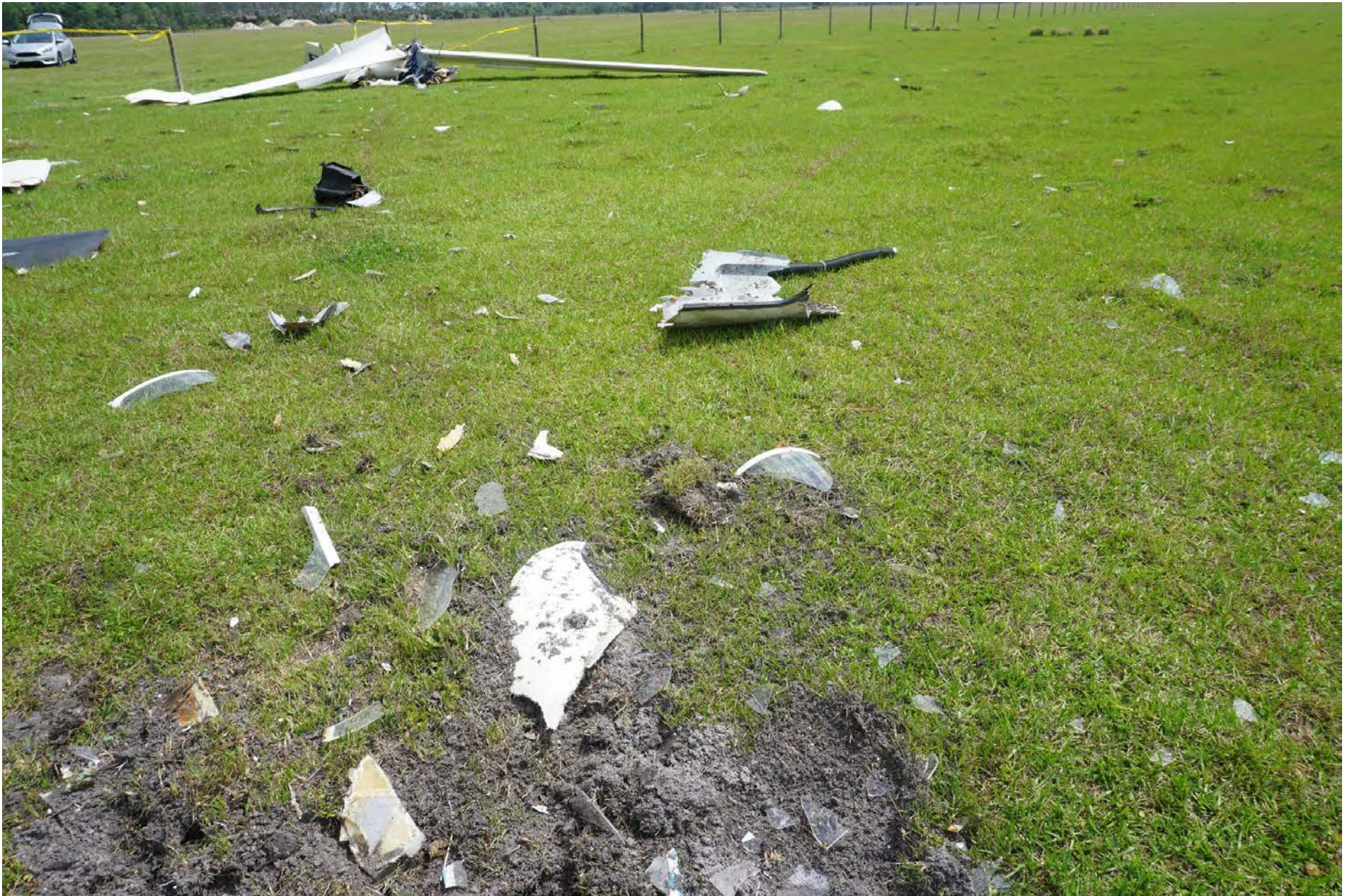
Photo 5 – Forward view of wreckage showing fragmented cockpit parts and instrument panel
