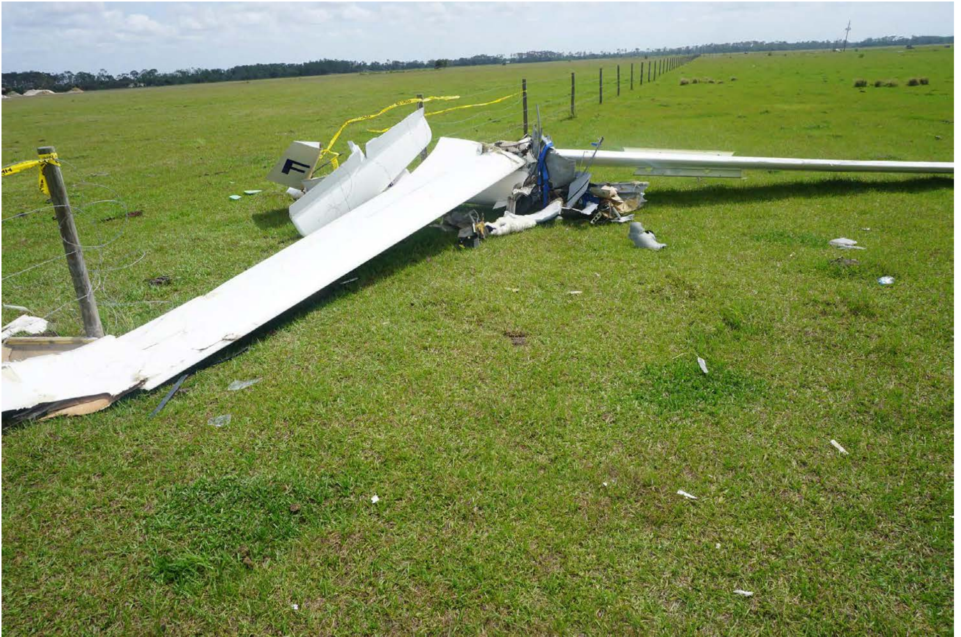
Photo 2 – Right-side view of wreckage showing damaged right wing and crushed cockpit
