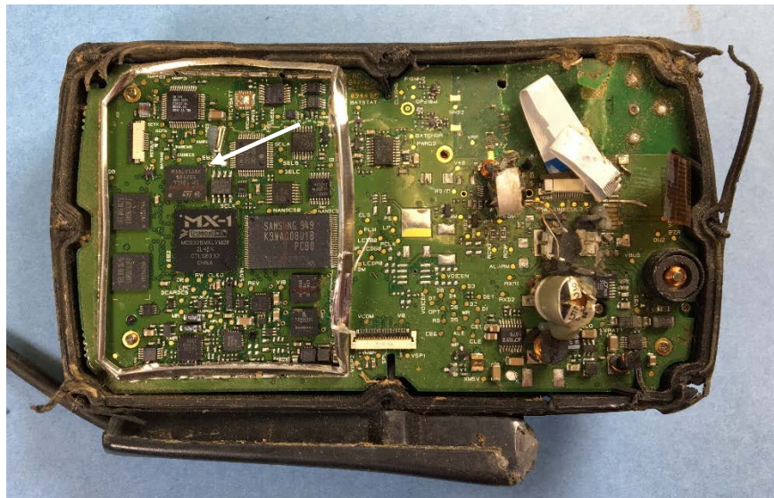
Figure 3. GPS memory chip indicated by white arrow.
