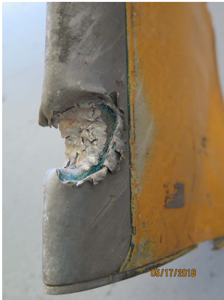
Photo 9 – View of ‘Blue’ Rotor Blade Leading Edge Damage (Boeing)
