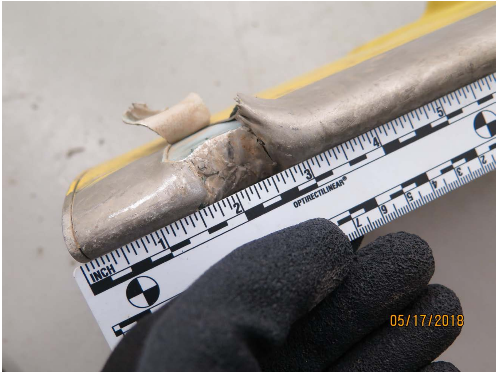
Photo 10 - View of 'Blue' Rotor Blade Leading Edge Damage (Boeing)
