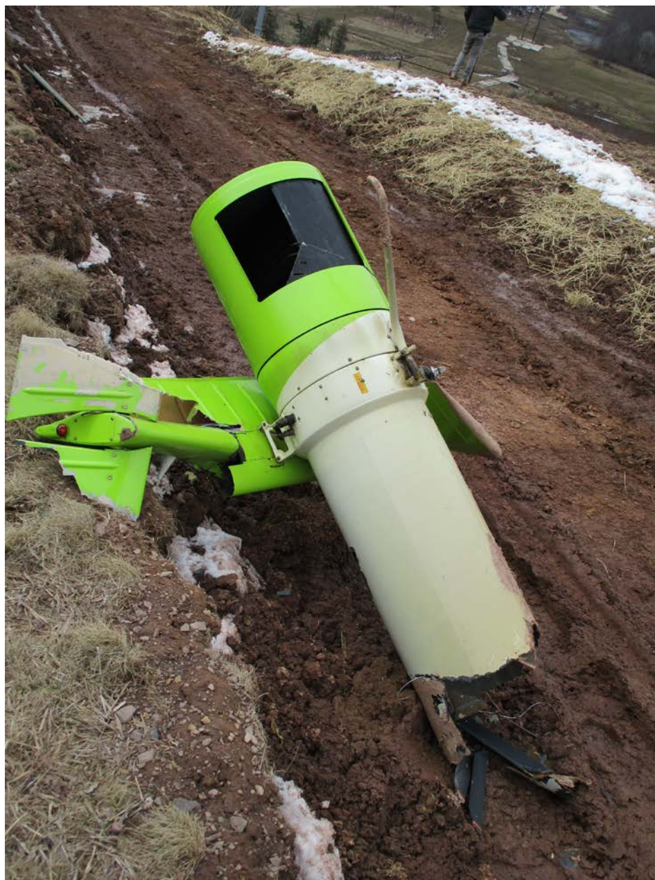
Photo 4 – View of Fractured Tailboom as Found (FAA)
