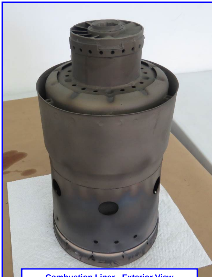
Combustion Liner - Exterior View
