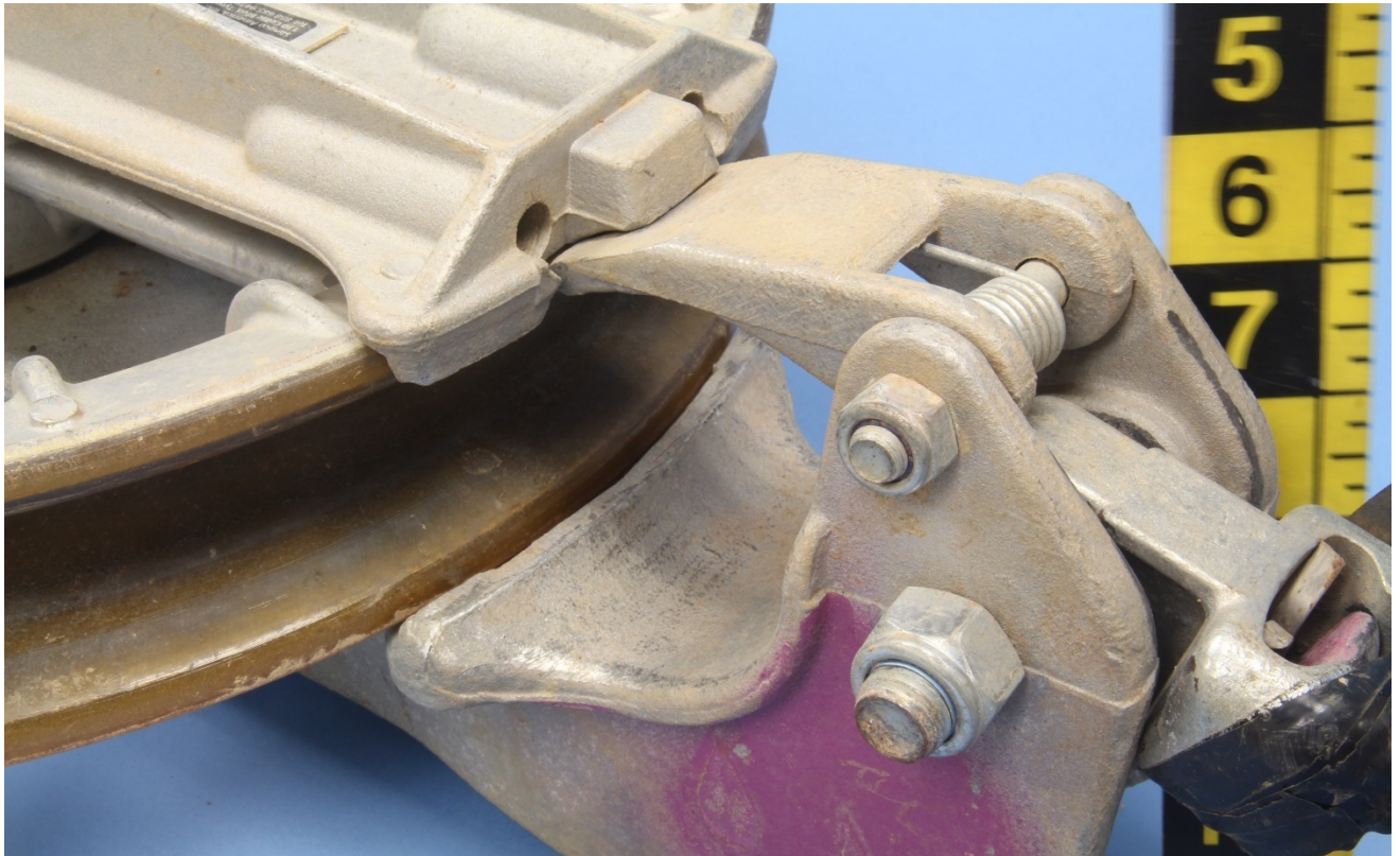
Figure 3 – The locking gate from Figure 2, shown from the side in the latch closed position.
