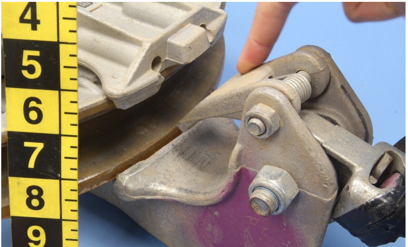
Figure 4 – The locking gate from Figure 2, shown from the side in the latch open position.
