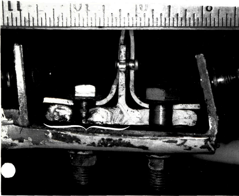
Figure 2. Inboard (left) and outboard (right) views of the lower spar cap fracture with the fatigue zones denoted by white brackets. Left view also shows fuselage carry through and attachment fasteners.
