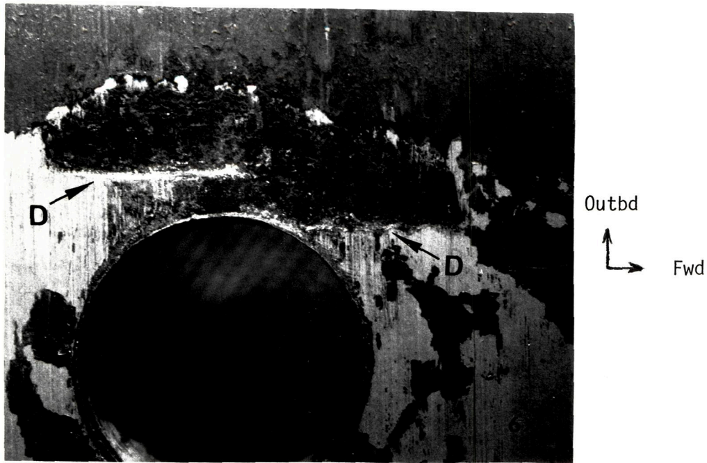
Figure 3. A view looking at the upper surface of the carry through at the forward outboard bolt hole (forward at right, outboard at top) showing the fretting demarkation lines which correspond to the spar fatigue planes.
