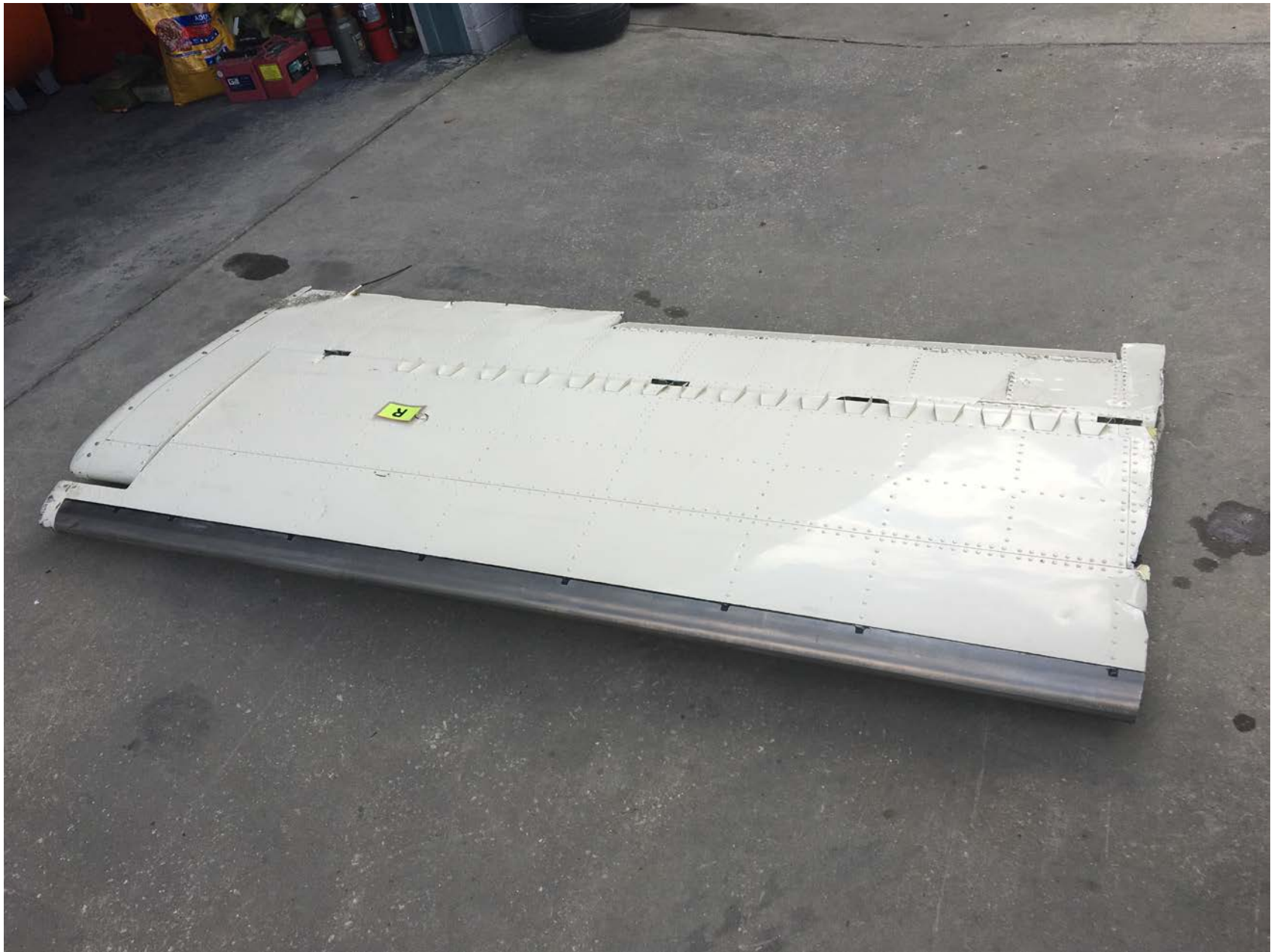
Photo 5 – Right Elevator (cut by recovery personnel)
