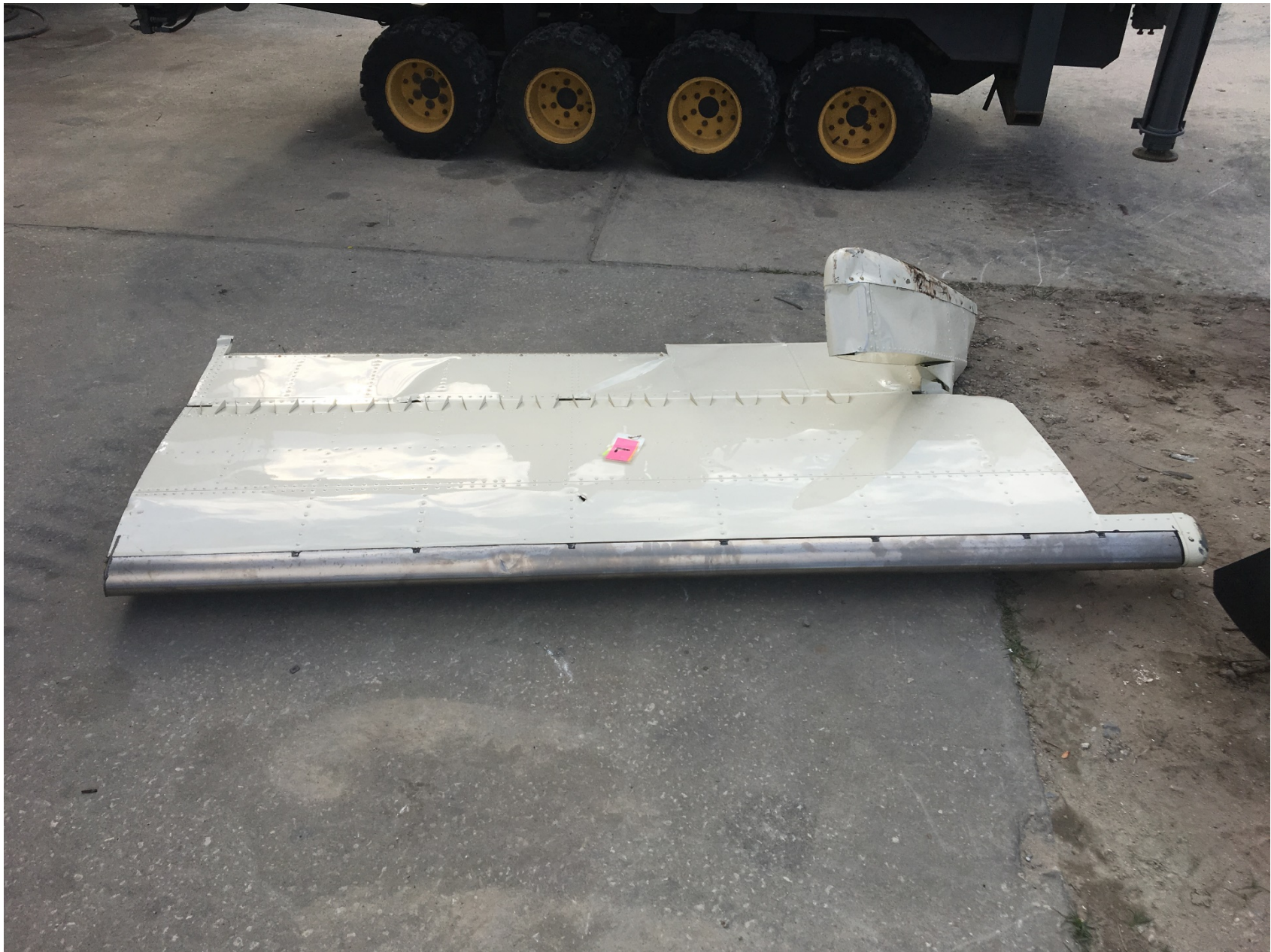
Photo 4 – Left Elevator (cut by recovery personnel)
