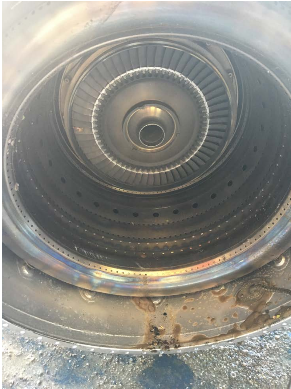
Photo 9 – View of debris in engine and rotational scoring on fir trees.
