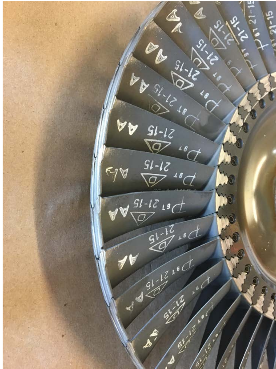
Photo 10 – View of rotational scoring on power turbine blades.
