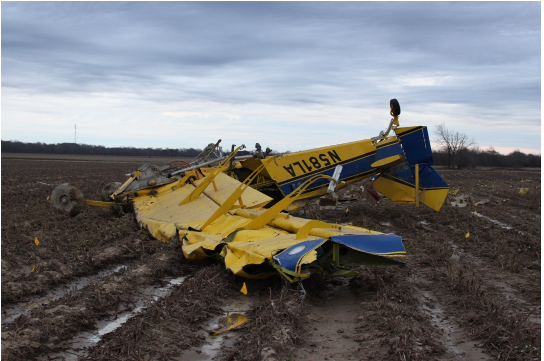
Photo 3 - NTSB Digital Photograph. Close-Up View of the Right Wing and Right Side of the Inverted Airplane at the Accident Site. Note the Damage to the Leading Edge of the Right Wing.
