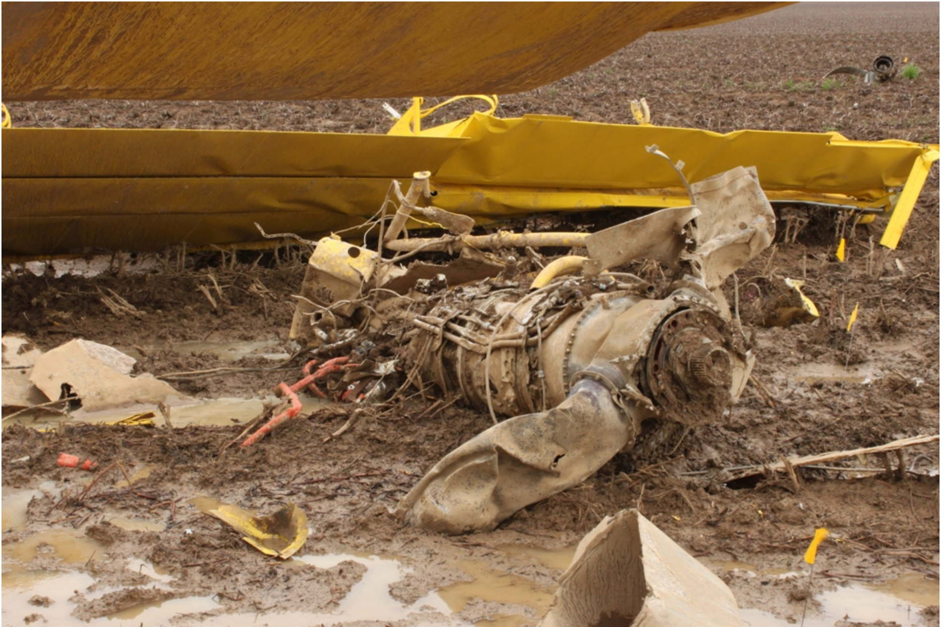
Photo 4 - NTSB Digital Photograph. Close-Up View of the Separated Engine Assembly behind Left Wing of Inverted Airplane at the Accident Site.
