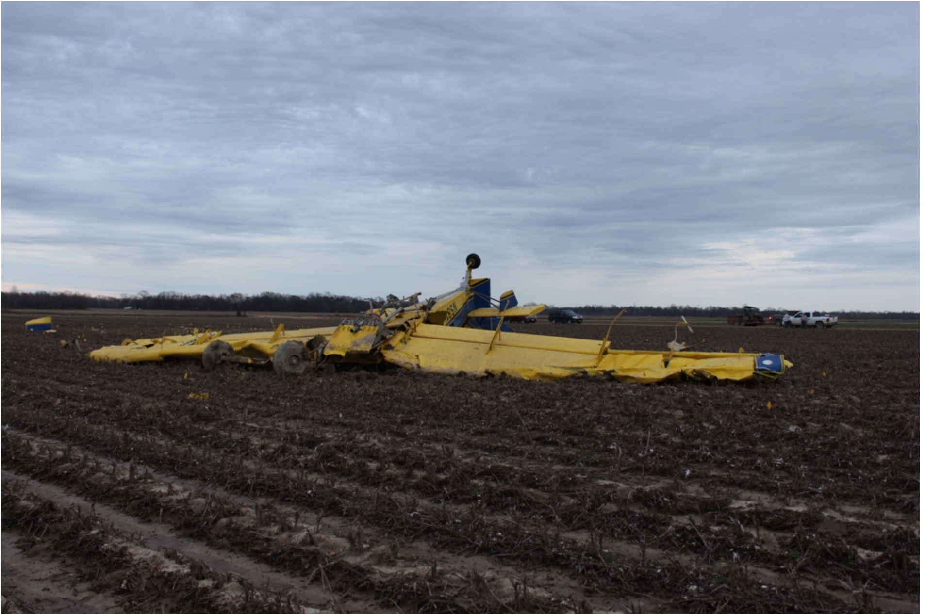
Photo 2 – NTSB Digital Photograph. Forward View of the Inverted Airplane at the Accident Site. Note the damage to the Leading Edge's of Both Wings.
