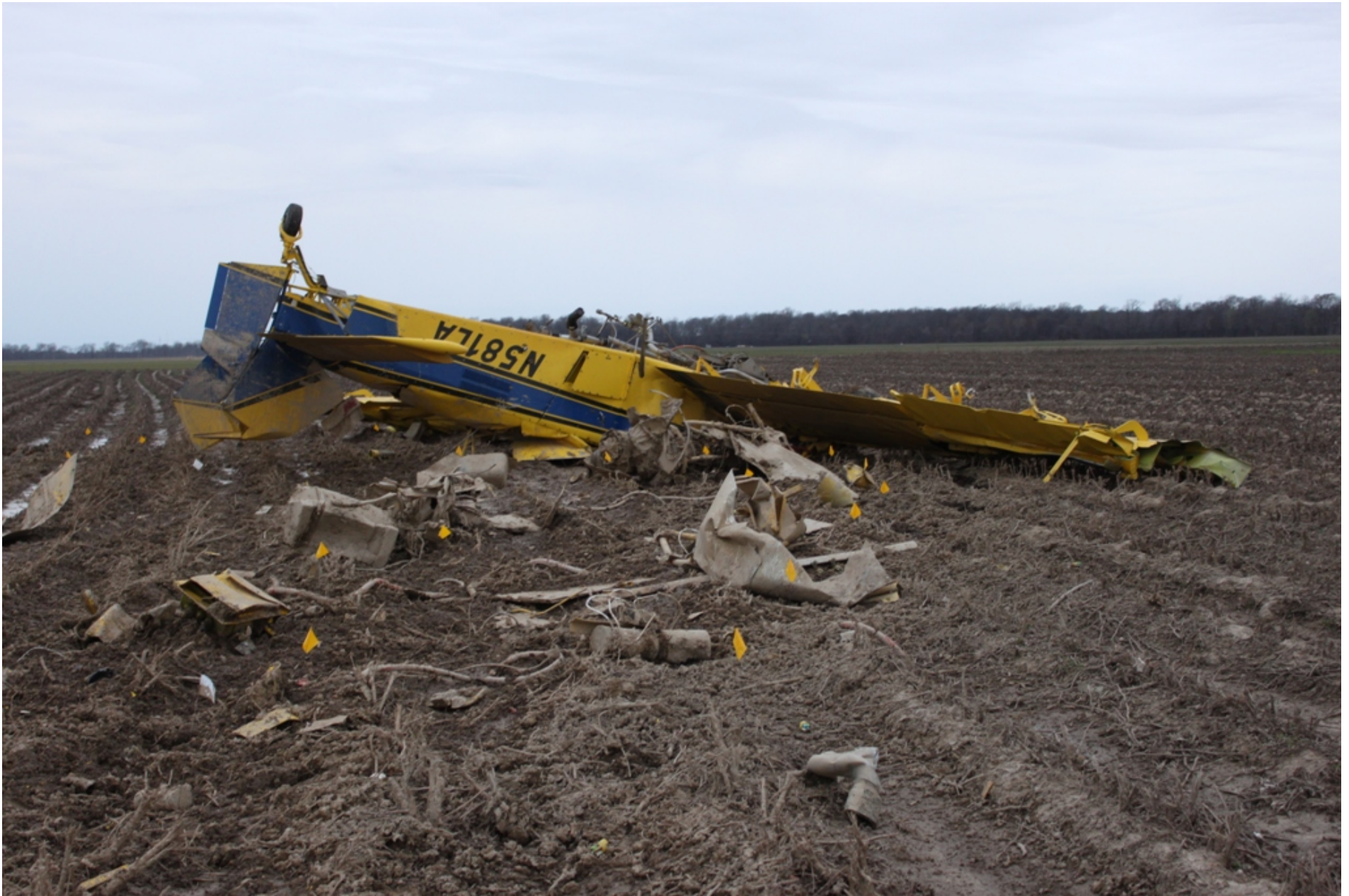
Photo 1 – NTSB Digital Photograph. Left Side View of the Inverted Airplane at the Accident Site.
