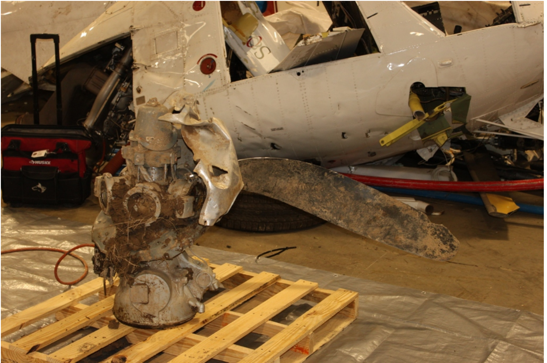
Photo 9 - NTSB Digital Photograph. View of the Propeller Assembly and Reduction Gearbox. Only 1 Propeller Blade remained Secured.
