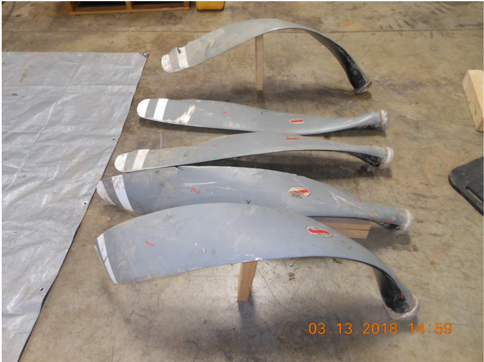
Photo 10 – Hartzell Digital Photograph. View of the Propeller Blades After Cleaning. Note the Varying Amount of Bending.
