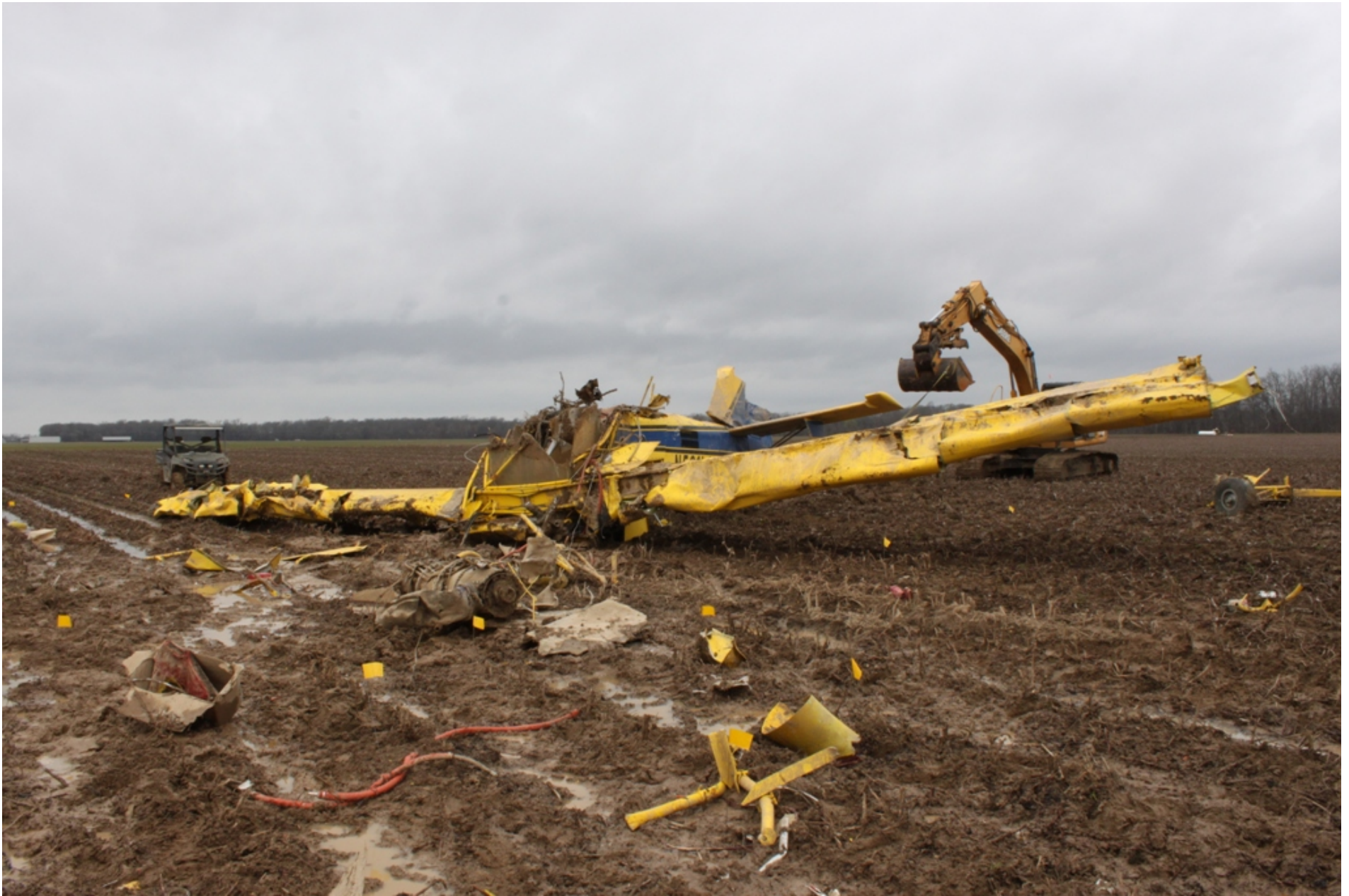
Photo 5 - NTSB Digital Photograph. View of the Airplane at the Accident Site Following Being Uprighted. Note the damage to the Leading Edge's of Both Wings.
