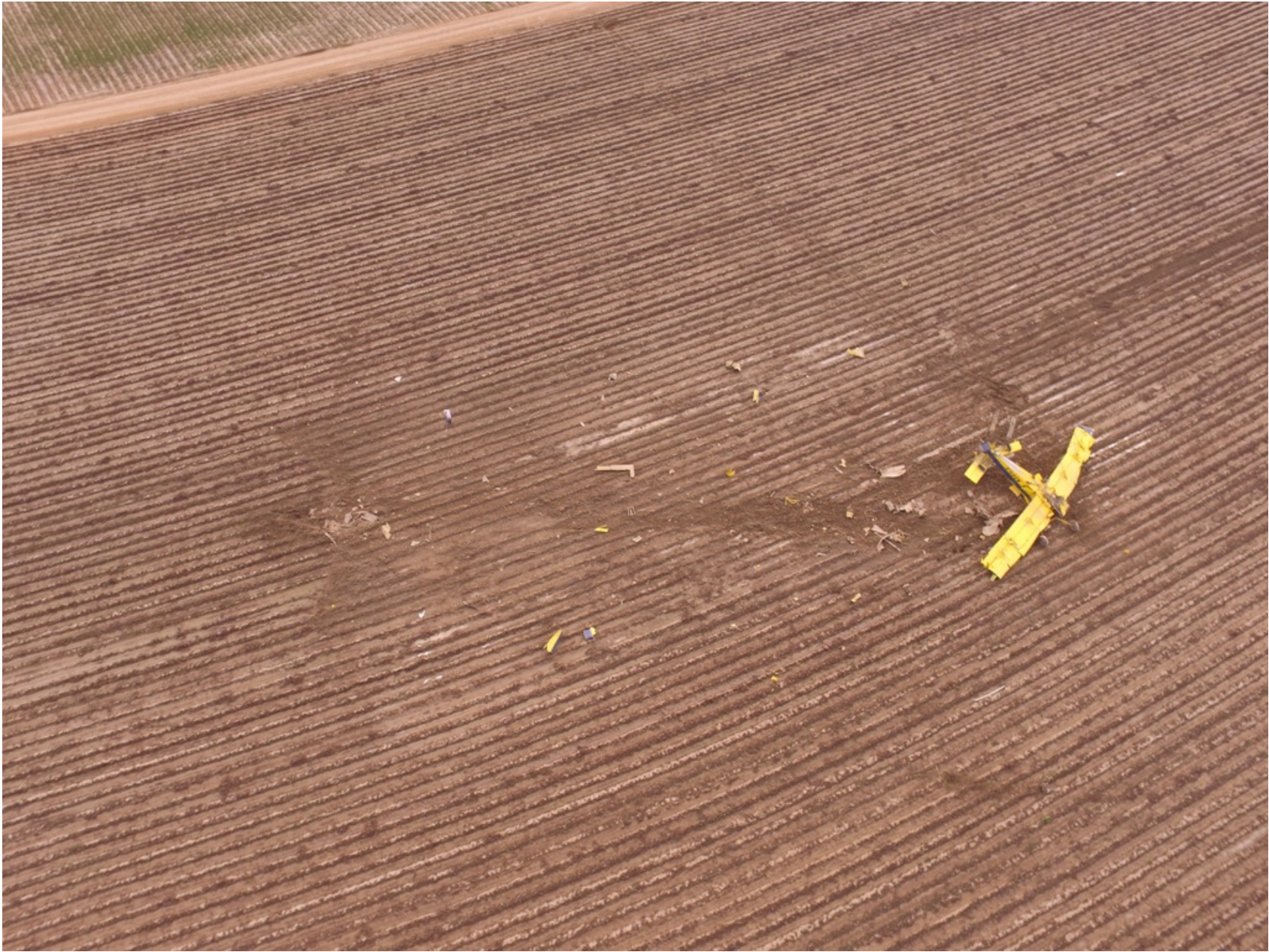
Photo 8 - Drone Image Provided by Doug Clark. View Depicting the Initial Impact Crater, Ground Scar, and Inverted Airplane at the Accident Site.
