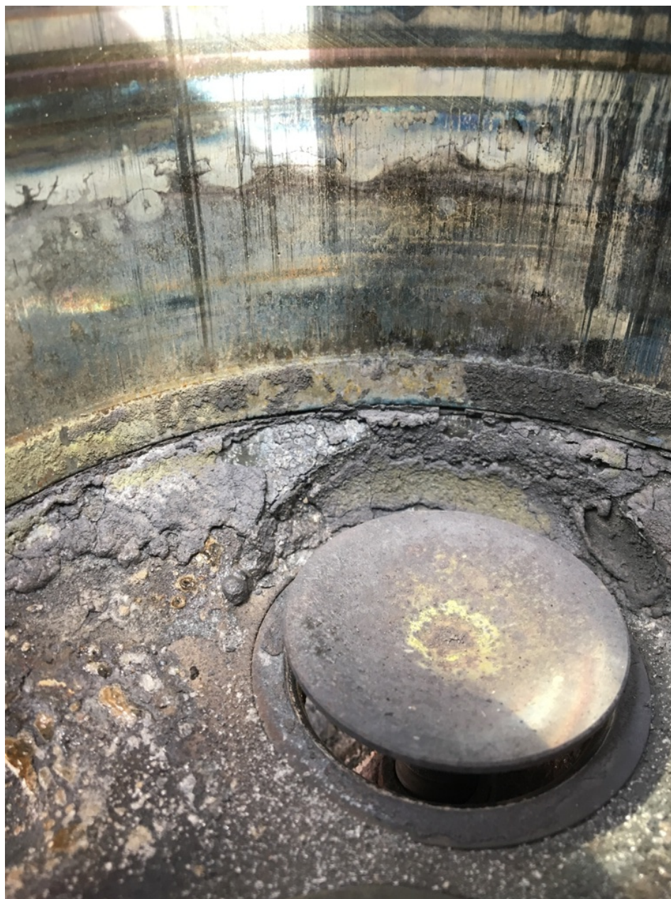
Photo 7 - No. 4 Cylinder/ Stuck Valve
