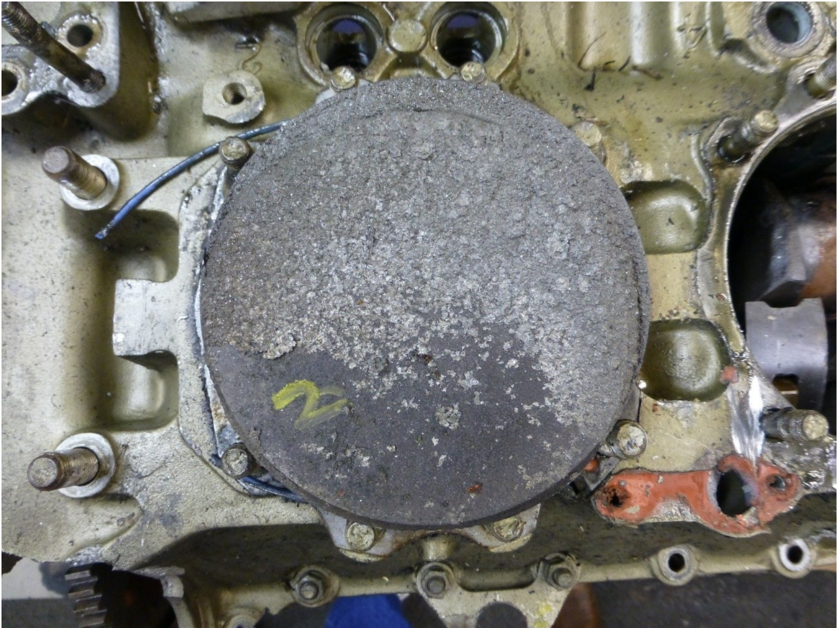
Photo 4 – Detonation damage to the crown of the piston.
