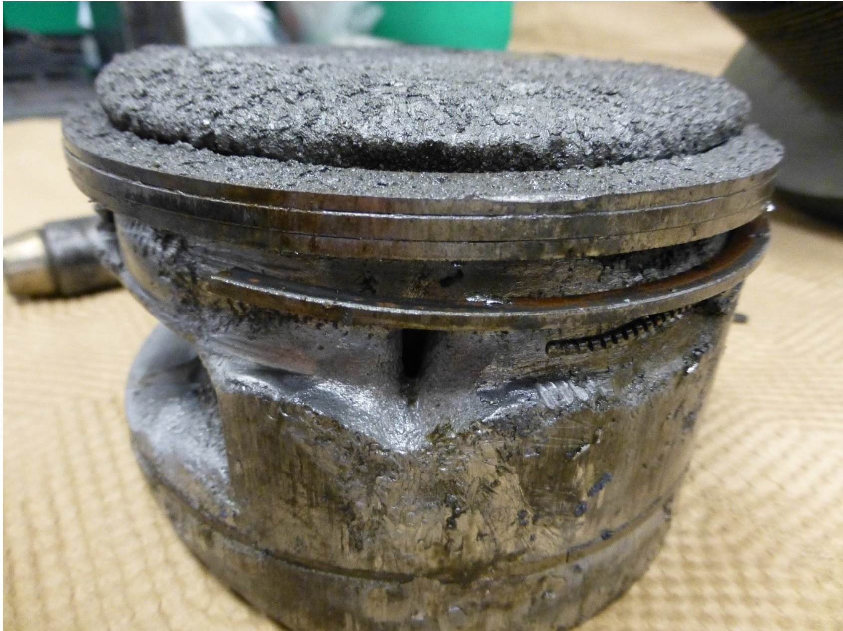
Photo 5 – Side view of the piston, damage to the oil control ring grooves.
