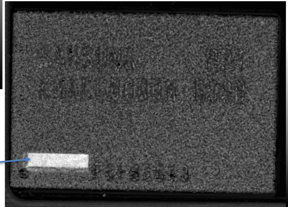
C-SAM image from within the mold compound.
