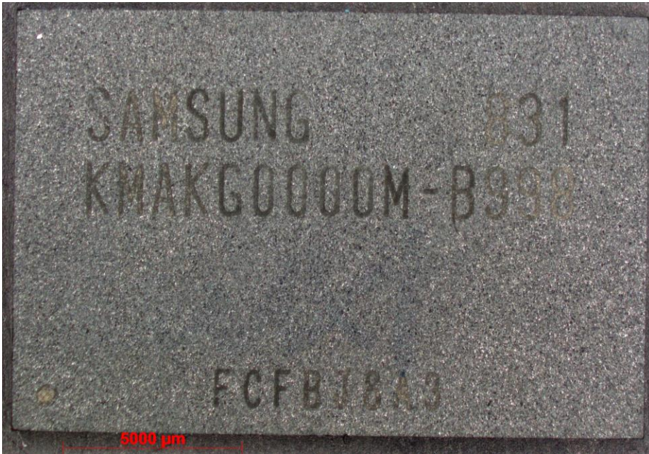
Front, mold side of the memory module
