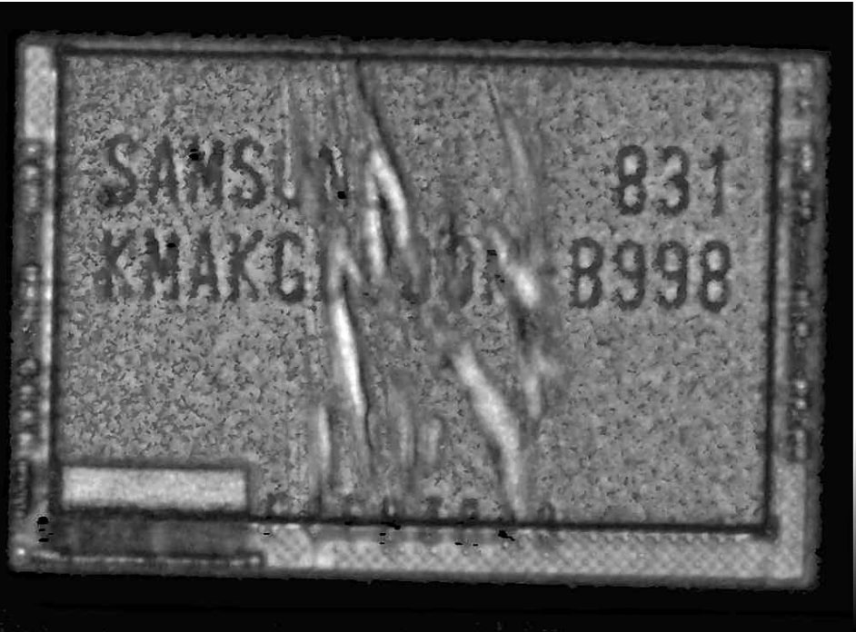
C-SAM image showing the laminated substrate. No cracks are seen in the substrate.
