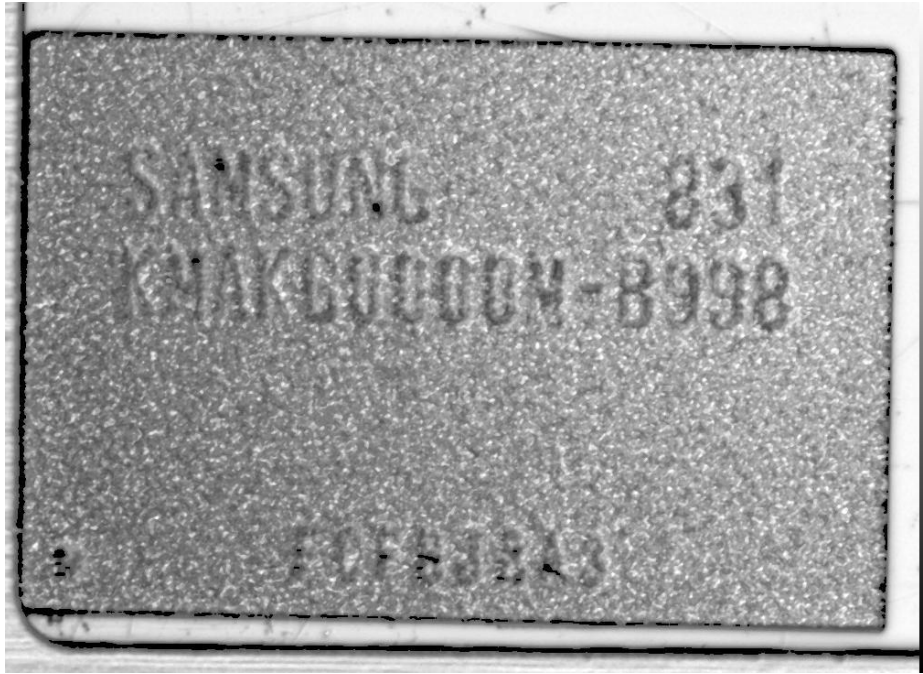
C-SAM image of the top surface of the package
