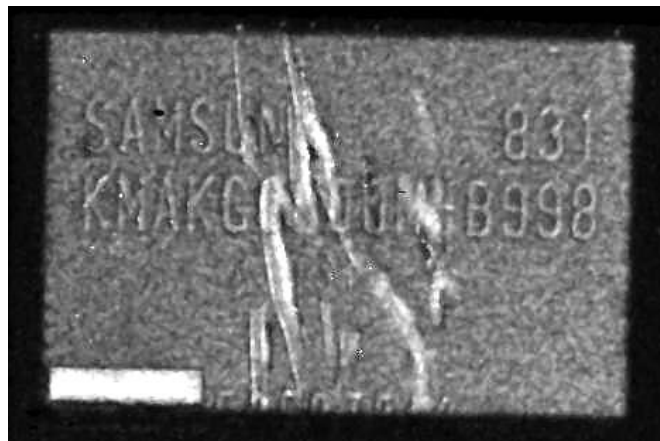
Figure 4. C-SAM image revealing damage to the die in the GPSMAP 696 NVM chip.
