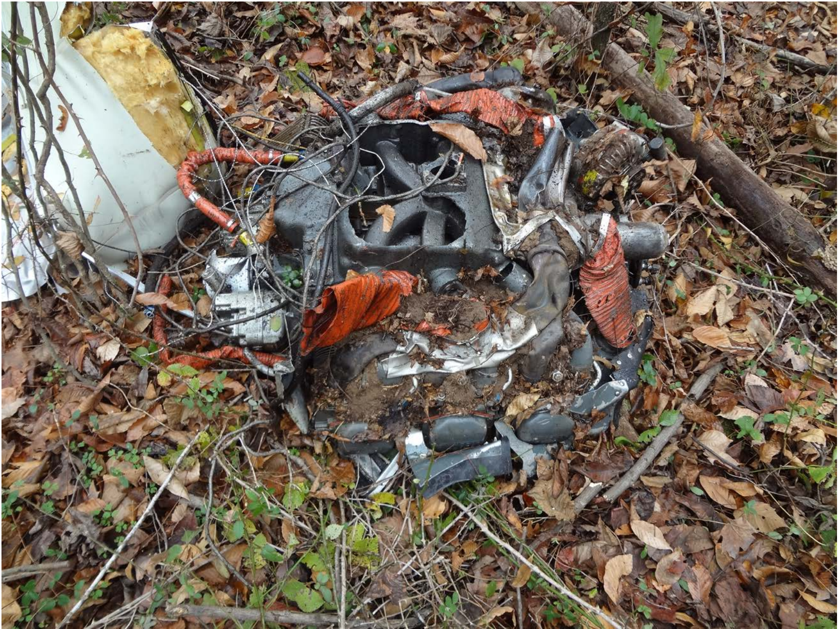
Photo 2 – View of Engine as Found (Lycoming)
