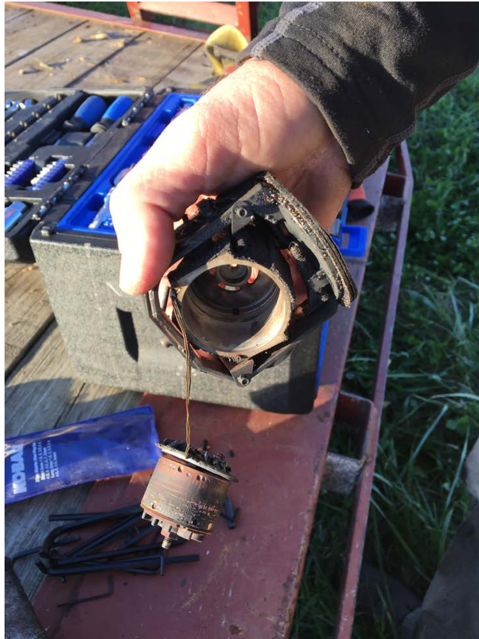
Photo 7 – View of Disassembled Gyro
