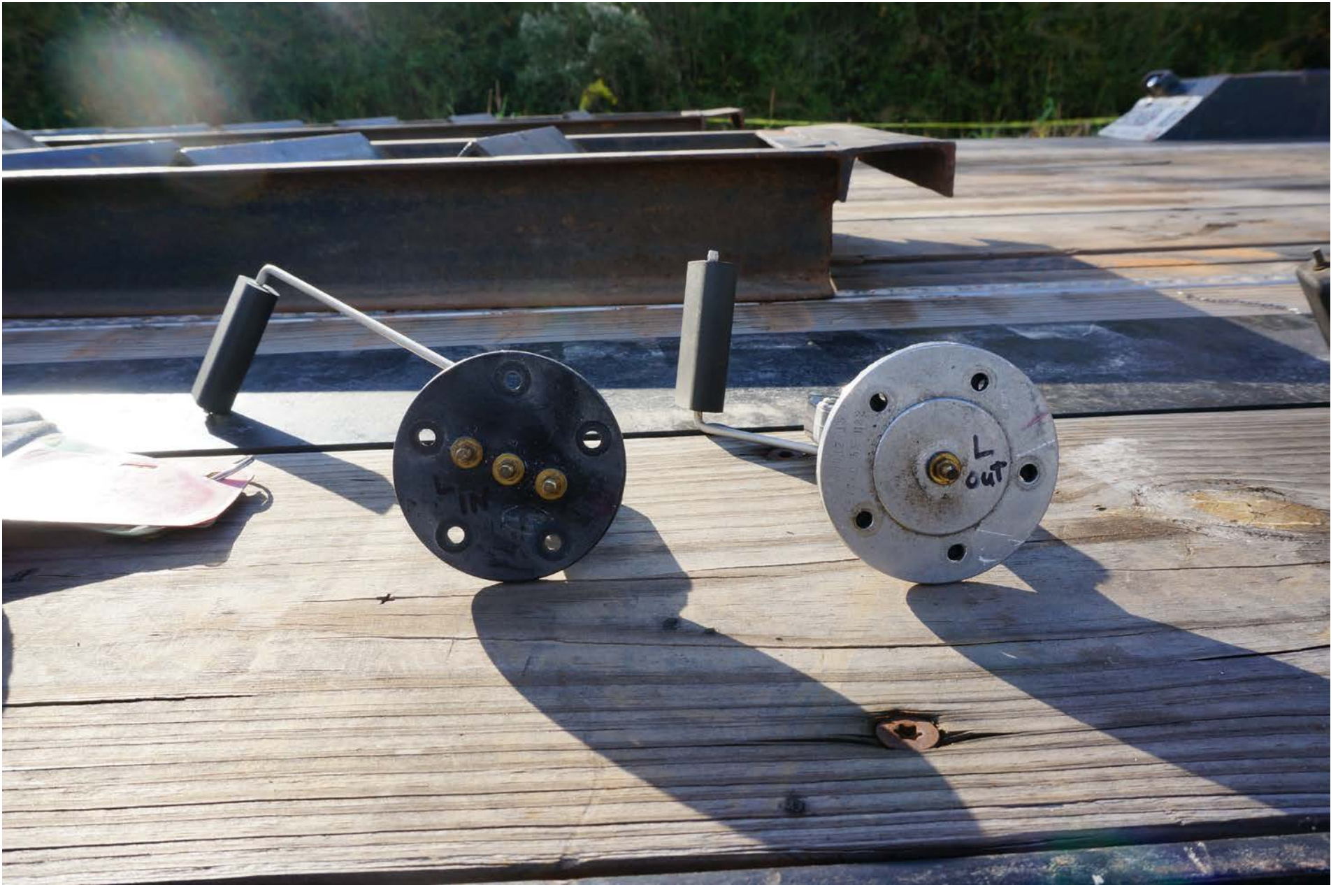
Photo 18 – Left Fuel Tank Inboard and Outboard Transmitters (After Removal)
