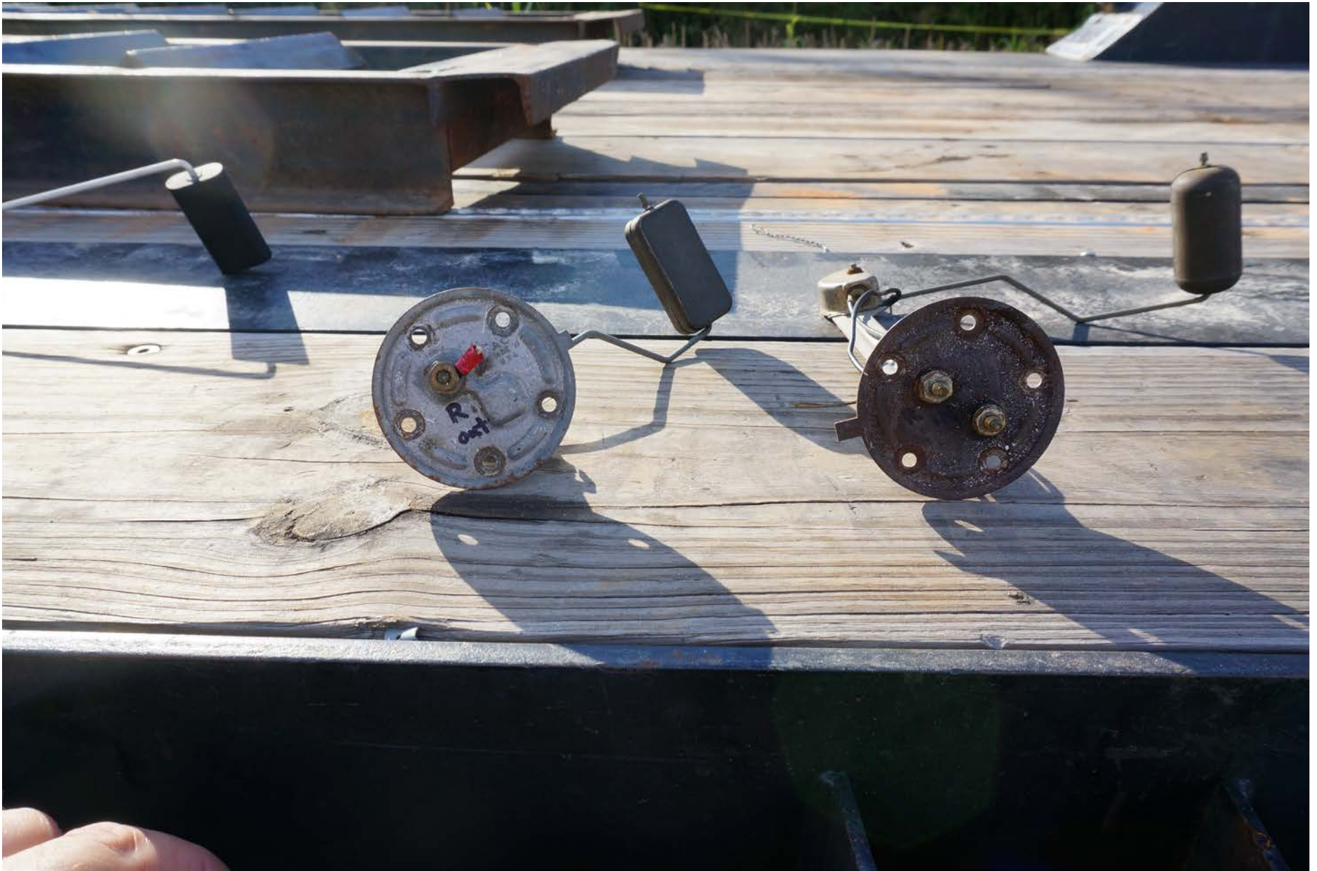
Photo 17 – Right Fuel Tank Inboard and Outboard Transmitters (After Removal)
