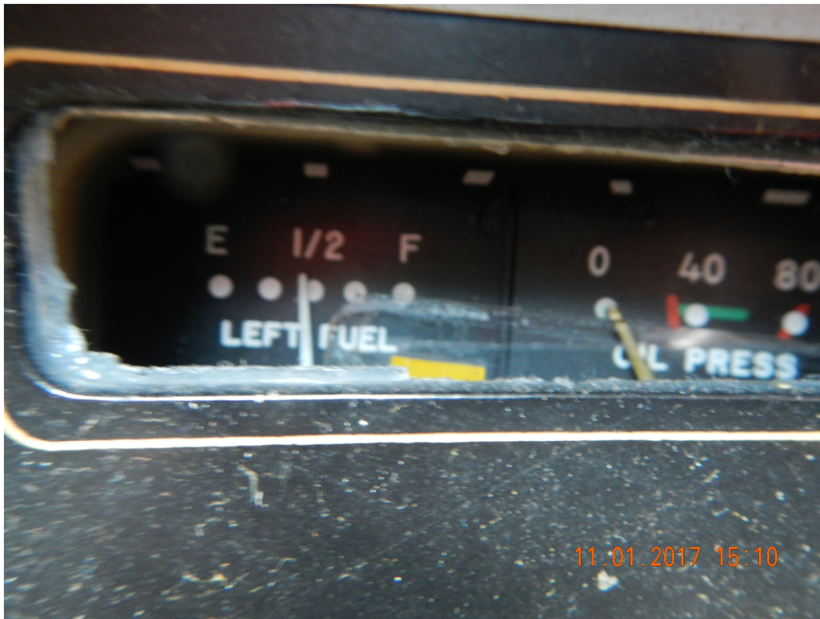
Photo 16 – Left Fuel Tank Gauge (Power On) – Courtesy of CMI
