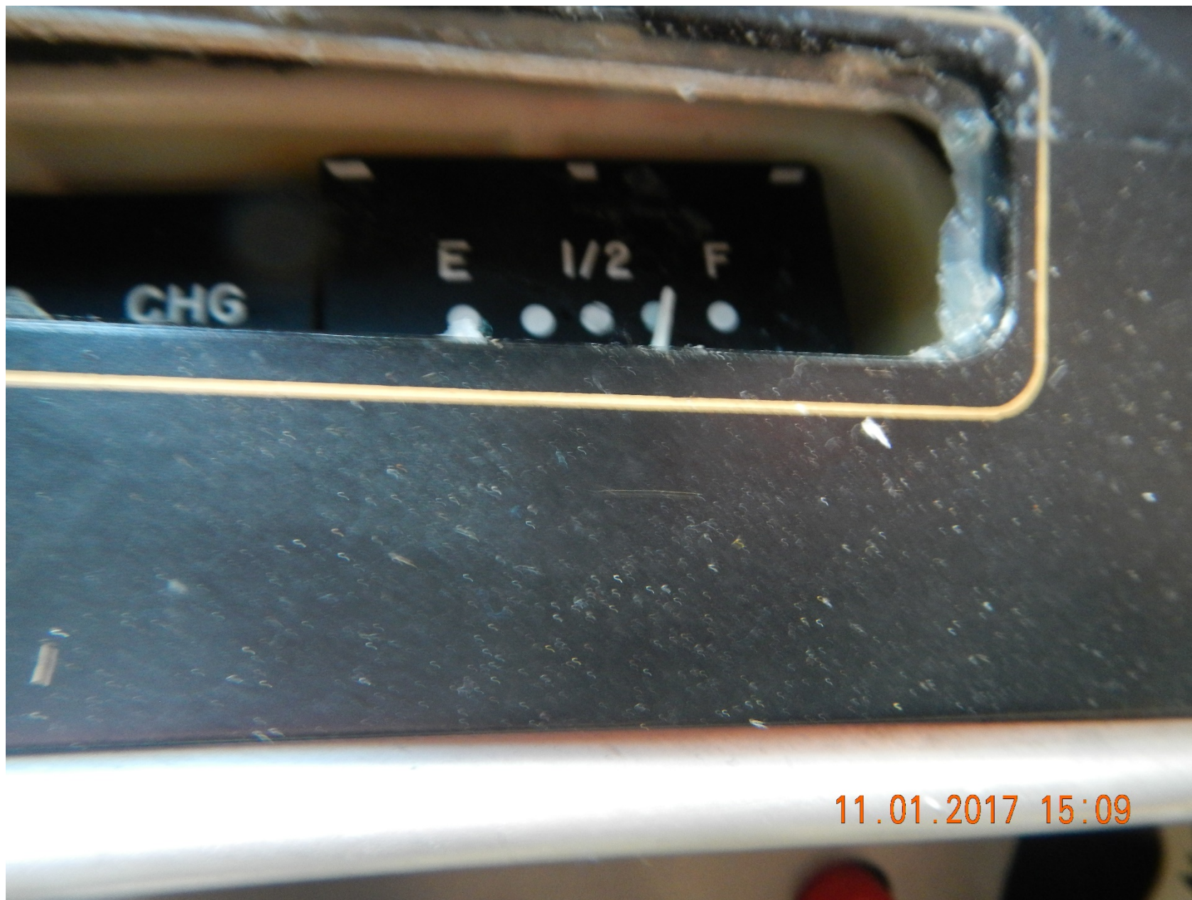
Photo 15 – Right Fuel Tank Gauge (Power On) – Courtesy of CMI
