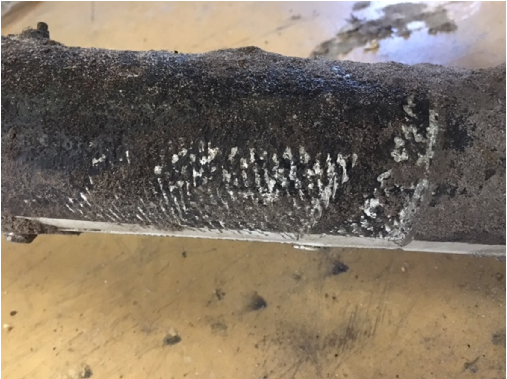
Photo 5 – Right Rear Skid Tube (Marion County Sheriff Photo)
