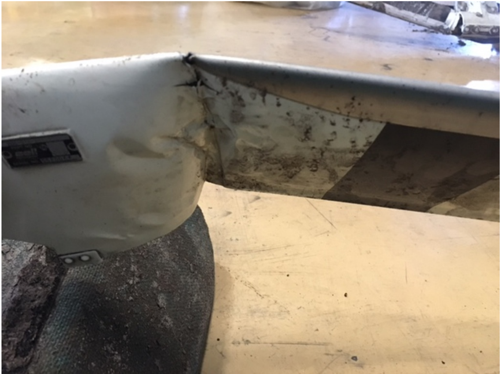
Photo 3 - Tail Rotor Blade Damage (Marion County Sheriff Photo)
