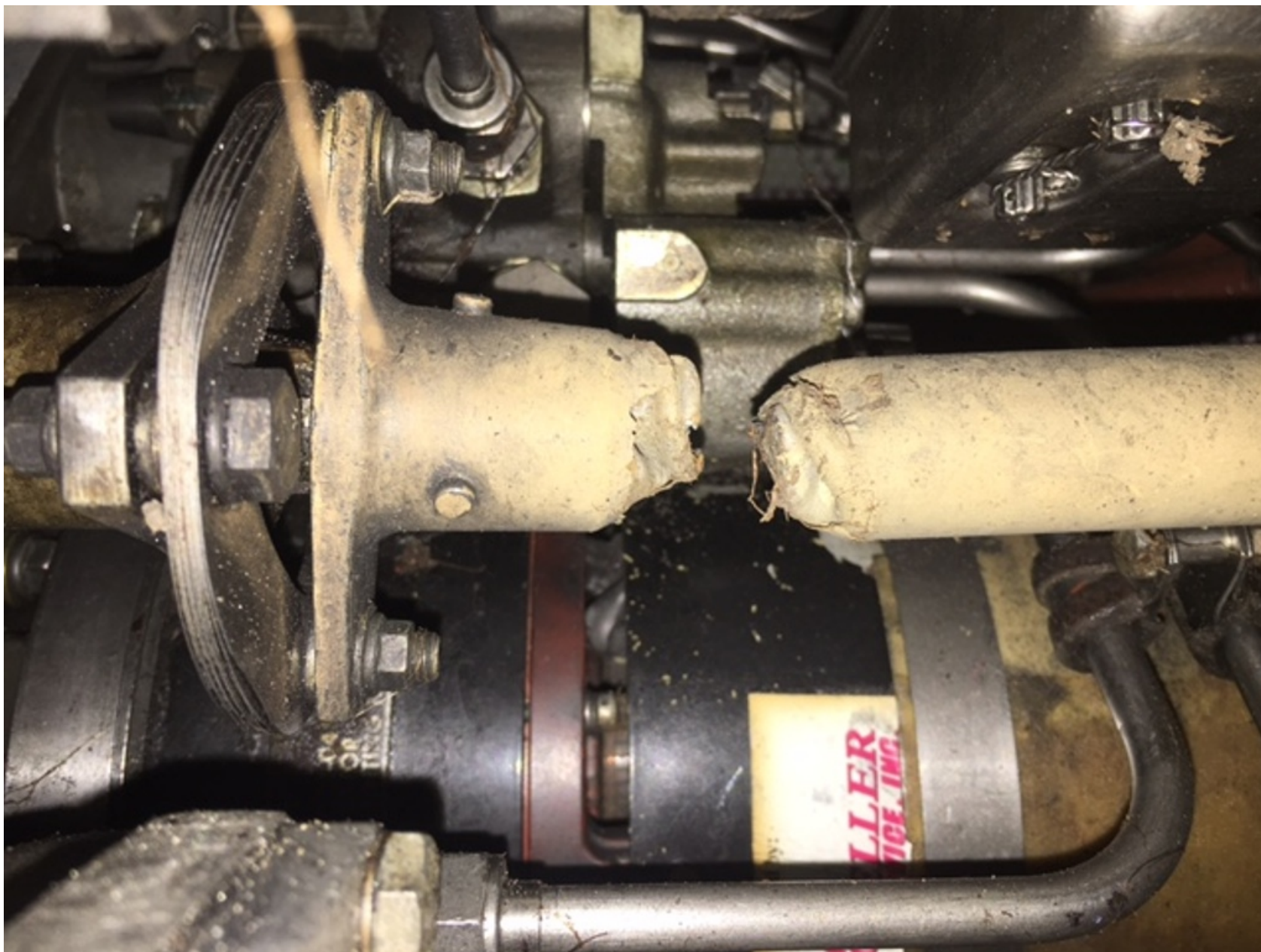
Photo 4 - Tail Rotor Short Shaft Fracture (Marion County Sheriff Photo)
