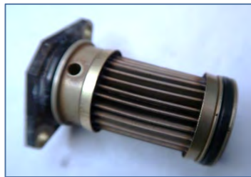
Fuel filter (HP) clean
