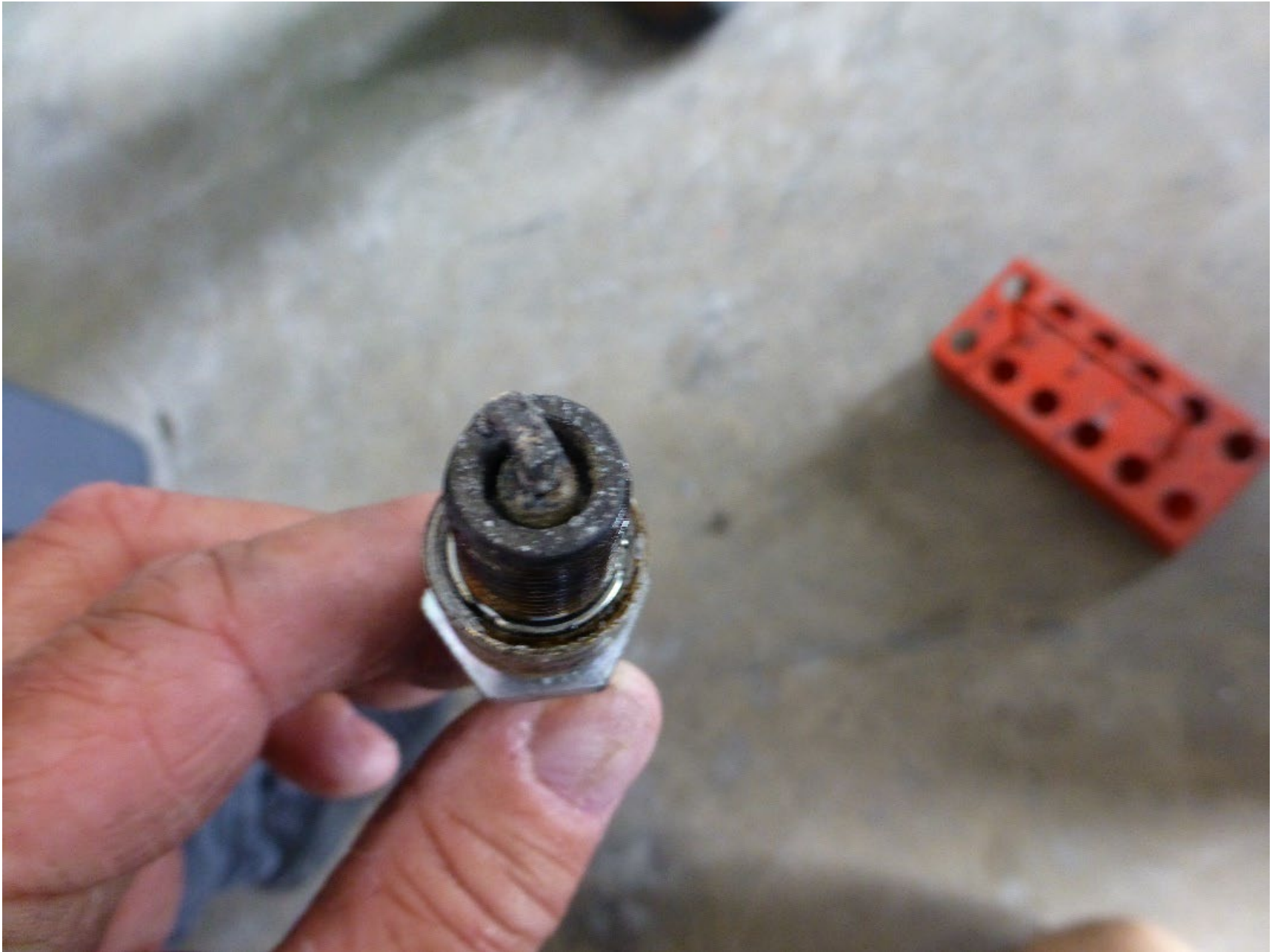
Photo 13 – Spark Plug from No.1 Cylinder Displaying Spatter
