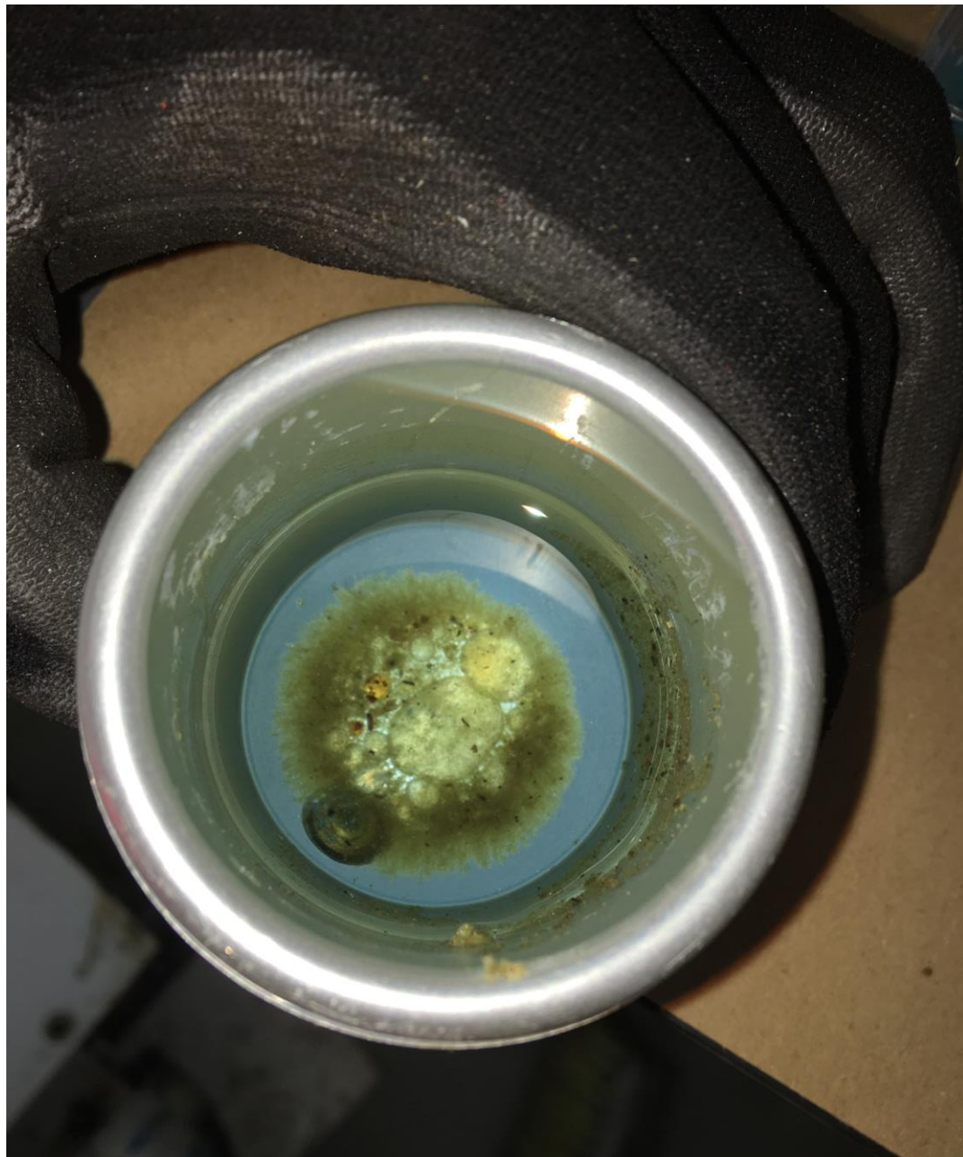
Photo 3 – View of fluid in gascolator.
