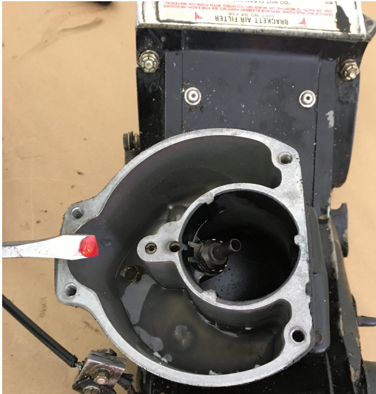
Photo 4 – View of fluid in carburetor with water finding paste.
