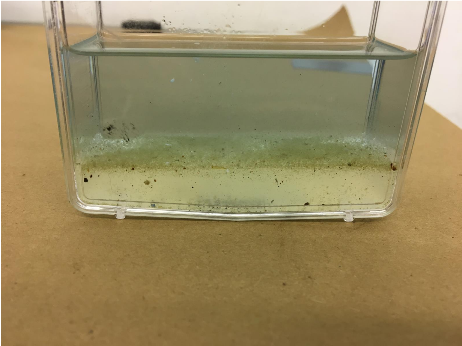
Photo 5 – View of contaminated fuel extracted from fuel system.
