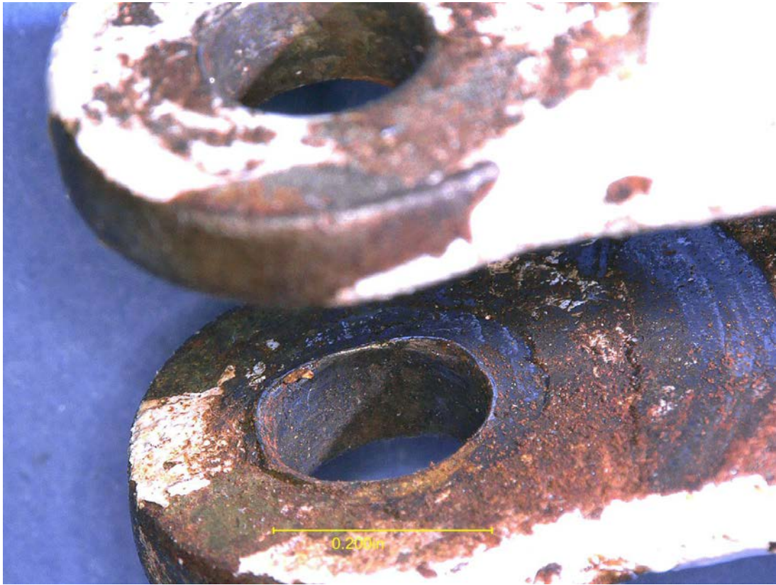
Figure 4: Deformed yoke bolt hole exhibiting a raised burr.
