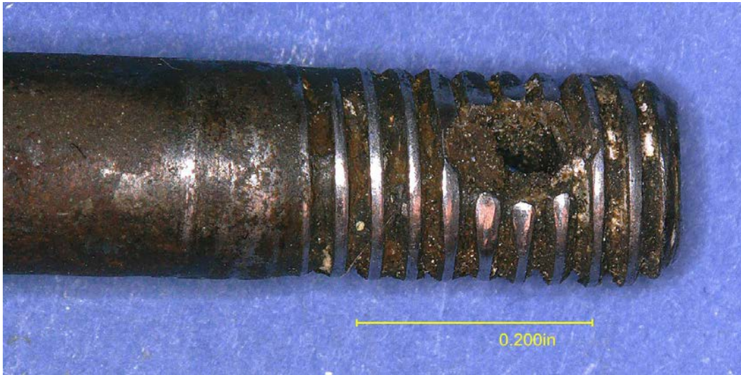
Figure 6: Flattened and polished bolt threads.
