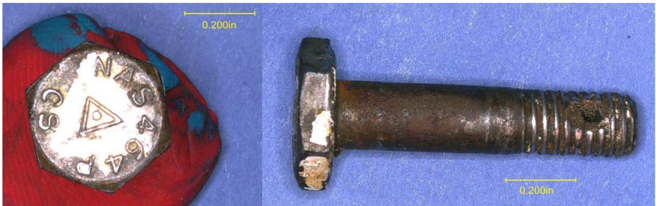
Figure 5: Bolt consistent with NAS464P3-8.
