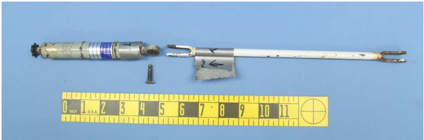
Figure 1: Trim tab actuator, push-pull rod and cross drilled bolt as received.
