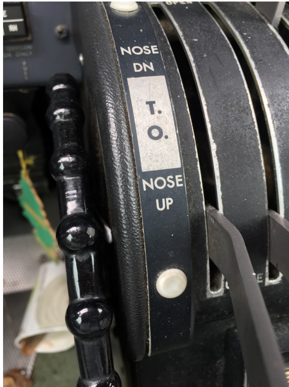
Photo 12 - Digital Photograph From FAA. Close-Up View of a Portion of the Elevator Trim Wheel and Pitch Trim Indicator. Note the Indicator was at the Nose-Up Stop.
