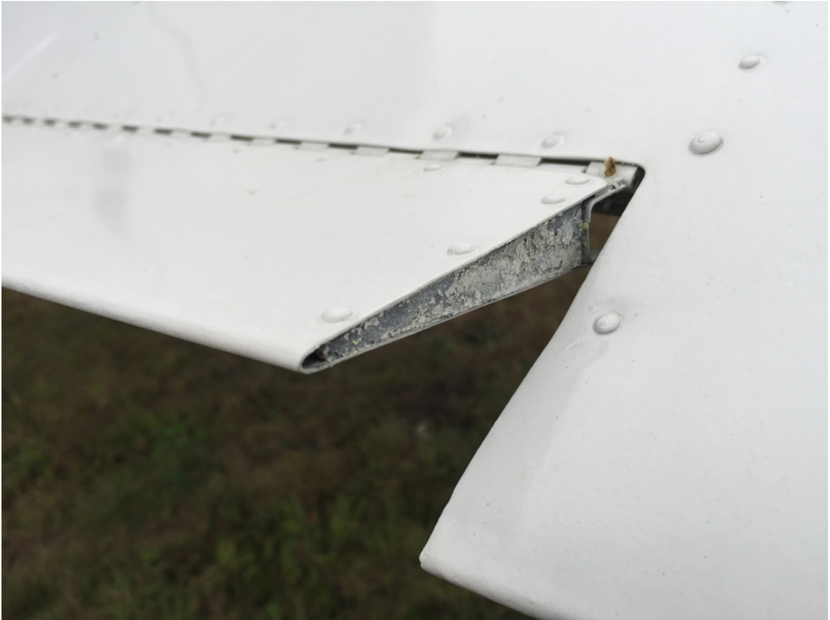
Photo 7 - Digital Photograph From FAA. Close-Up View Depicting the Outboard Portions of the Elevator Trim Tab and Adjacent Right Elevator Depicting the Tab Trailing Edge Up Position (Airplane Nose-Down).
