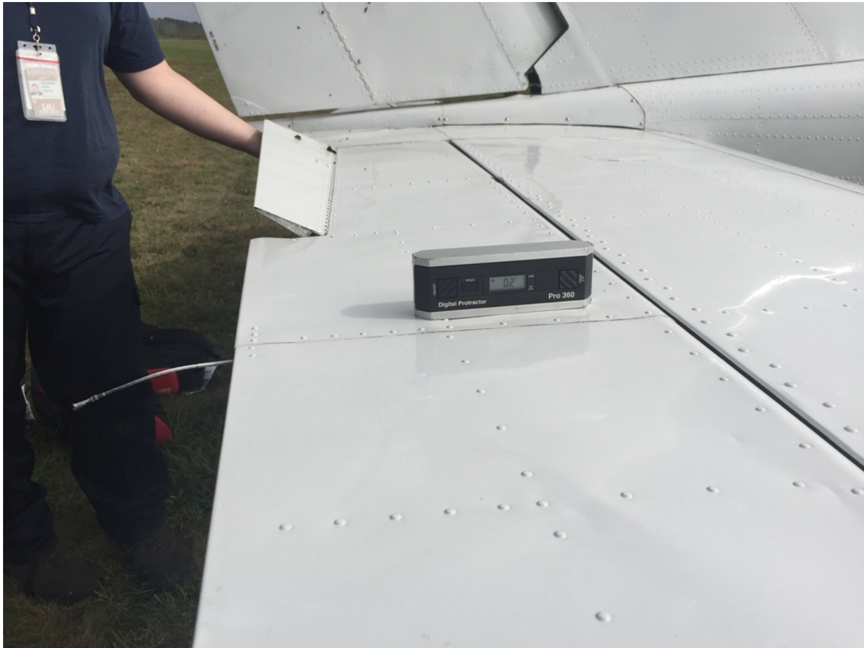
Photo 8 - Digital Photograph From FAA. View Depicting the Right Elevator in a Neutral Position and the Elevator Trim Tab in a Trailing Edge Up Position (Airplane Nose-Down).
