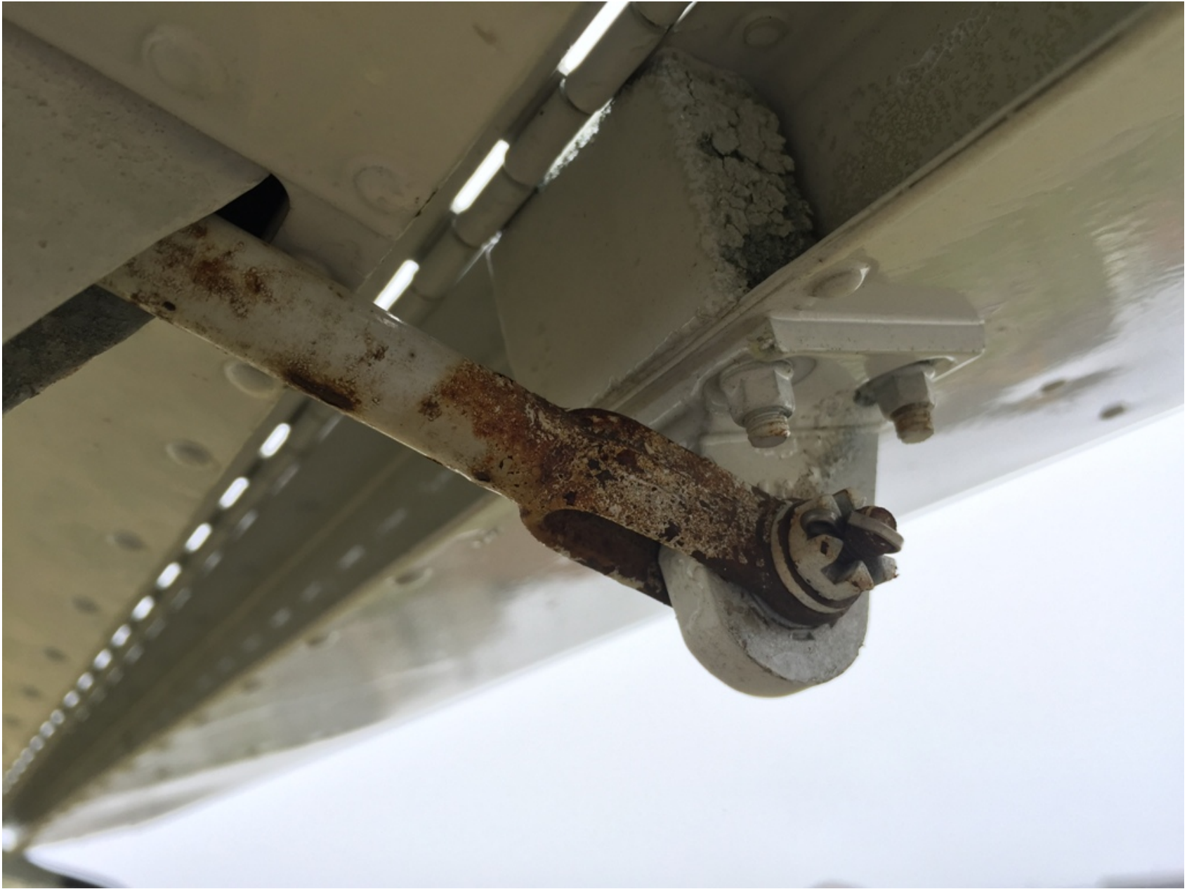
Photo 5 - Digital Photograph From FAA. View of the Elevator Trim Push Rod Assembly Connected at the Elevator Trim Tab.
