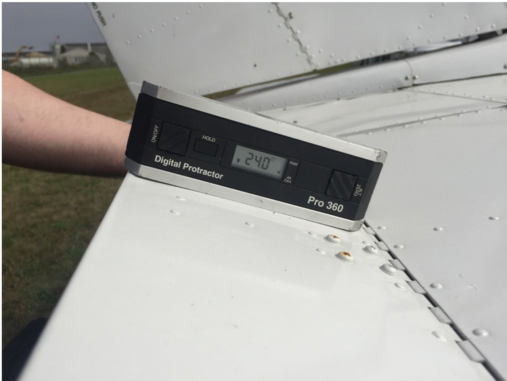
Photo 9 - Digital Photograph From FAA. View Depicting the Right Elevator in a Neutral Position and the Elevator Trim Tab in a 24 Degrees Trailing Edge Up Position (Airplane Nose-Down).
