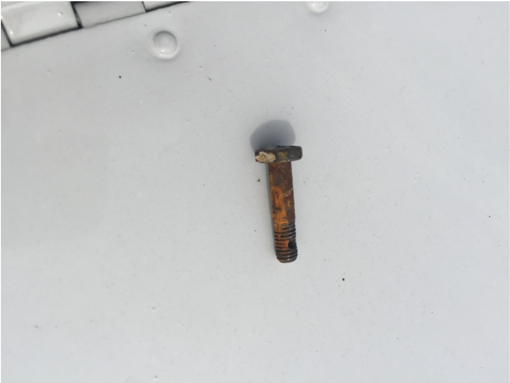
Photo 11 - Digital Photograph From FAA. View of the Bolt Recovered From Inside the Right Elevator. It was retained for Examination by NTSB.
