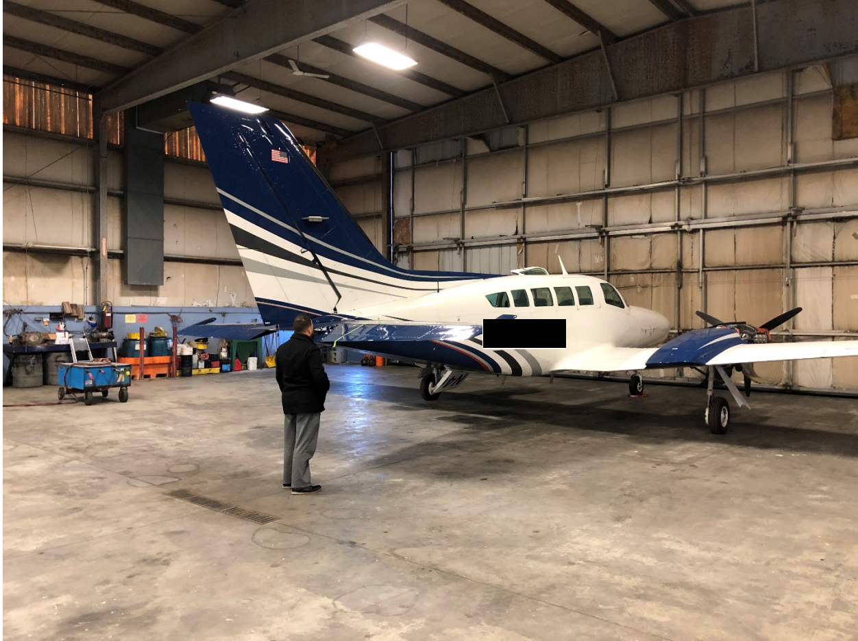
Figure 3: FAA Photograph of a Cessna 402C from same Orientation as Owner Provided Photo. Tape on Elevator depicts the location of the elevator trim tab actuator location.
