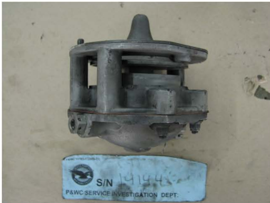
Photo No. 50 Bleed off valve
