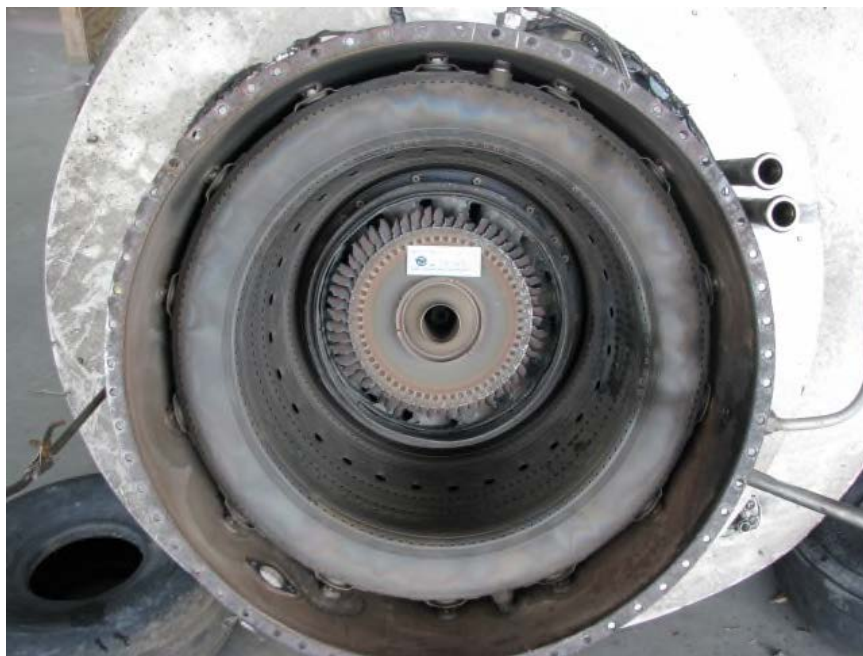
Photo No. 28 Compressor turbine in-situ
