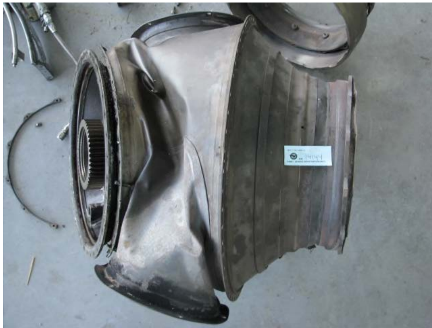
Photo No. 4 Exhaust duct impact damage
