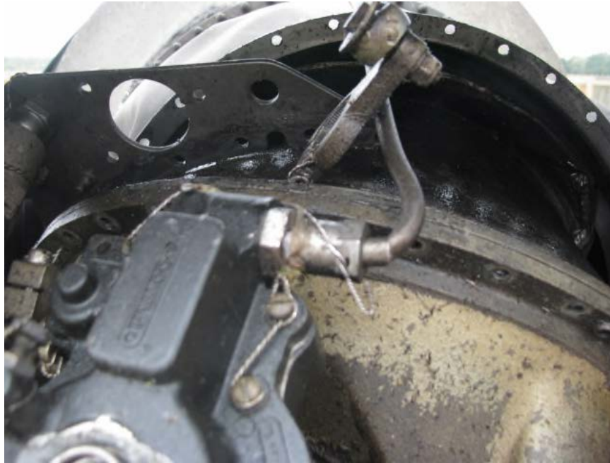
Photo No. 3 Reduction gearbox separated at the "B" flange
