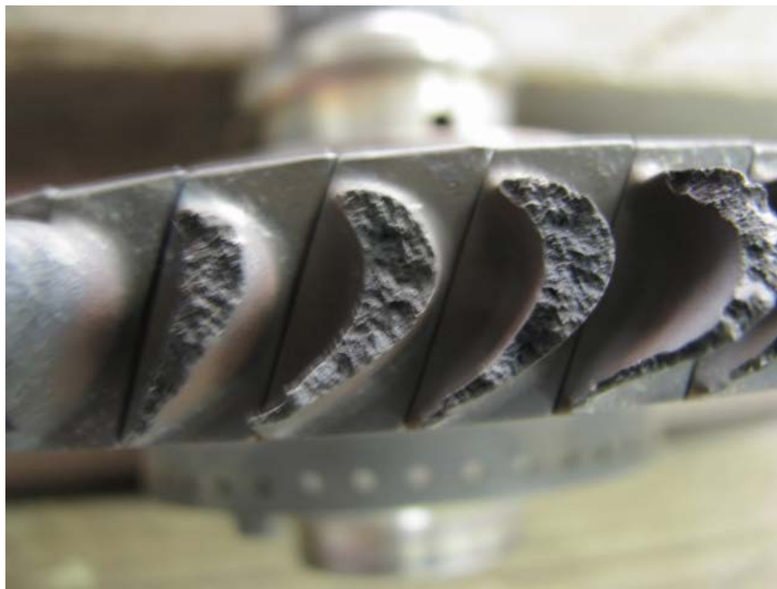
Photo No. 30 View of typical fracture surfaces observed on the compressor turbine blades
