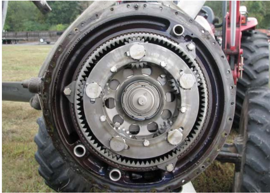
Photo No. 9 Second stage planet gear carrier assembly
