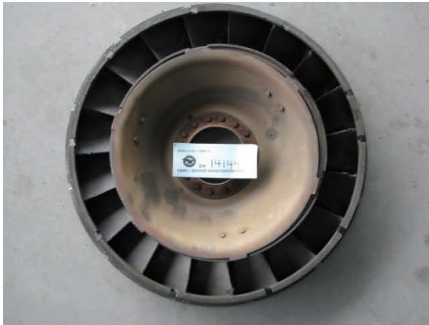
Photo No. 37 Upstream view of the power turbine stator
