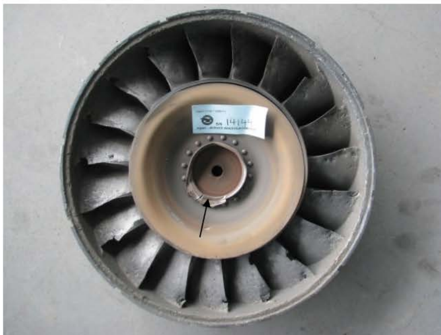
Photo No. 38 Downstream view of the power turbine stator
