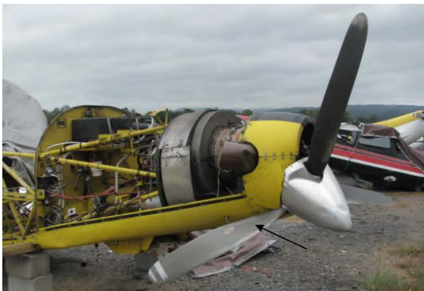
Photo No. 2 Bent Propeller and right exhaust stack
