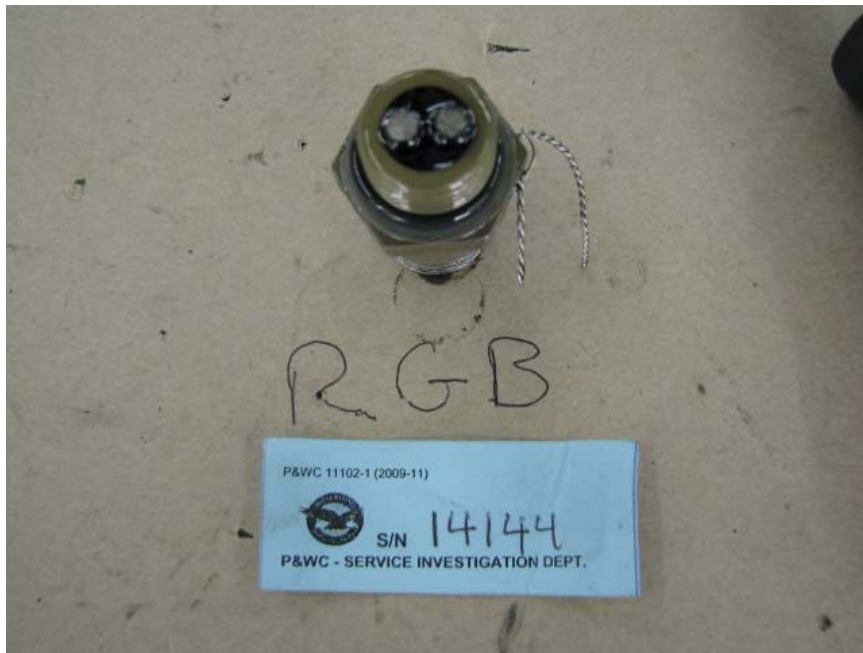
Photo No. 18 Reduction gearbox magnetic chip detector
