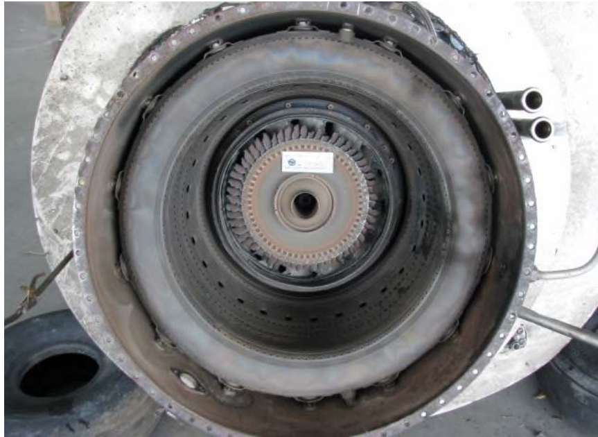
Photo No. 20 Outer combustion liner
