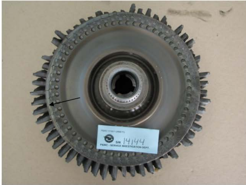
Photo No. 31 Leading edge view of compressor turbine disc
