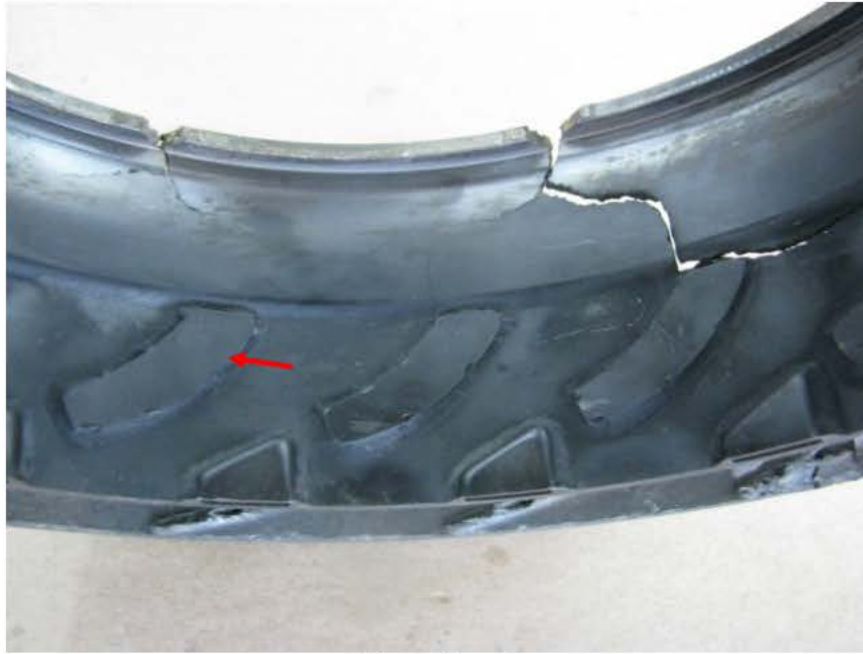
Photo No. 23 Compressor turbine inner shroud side welds
