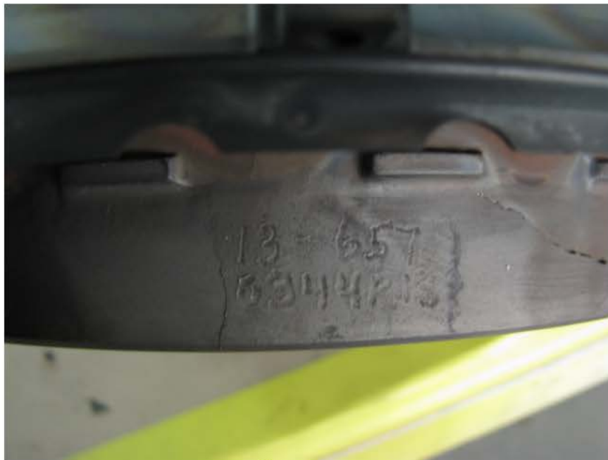
Photo No. 26 CT stator markings
