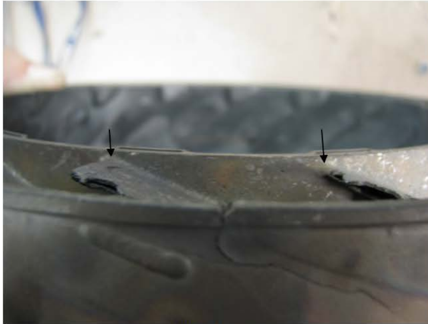
Photo No. 25 Trailing edge vane locations
