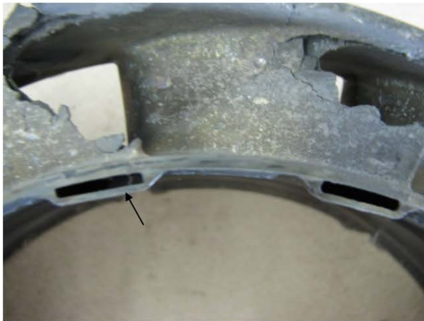
Photo No. 24 Compressor turbine stator air slots
