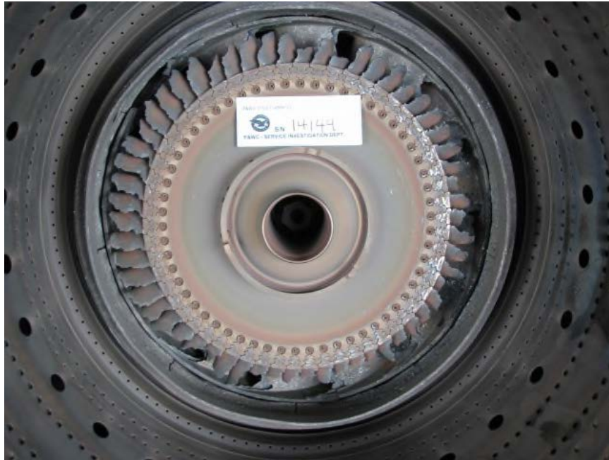
Photo No. 29 Closer view of compressor turbine blades damages
