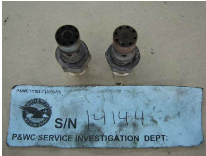
Photo No. 47 Intact ignitor plugs
