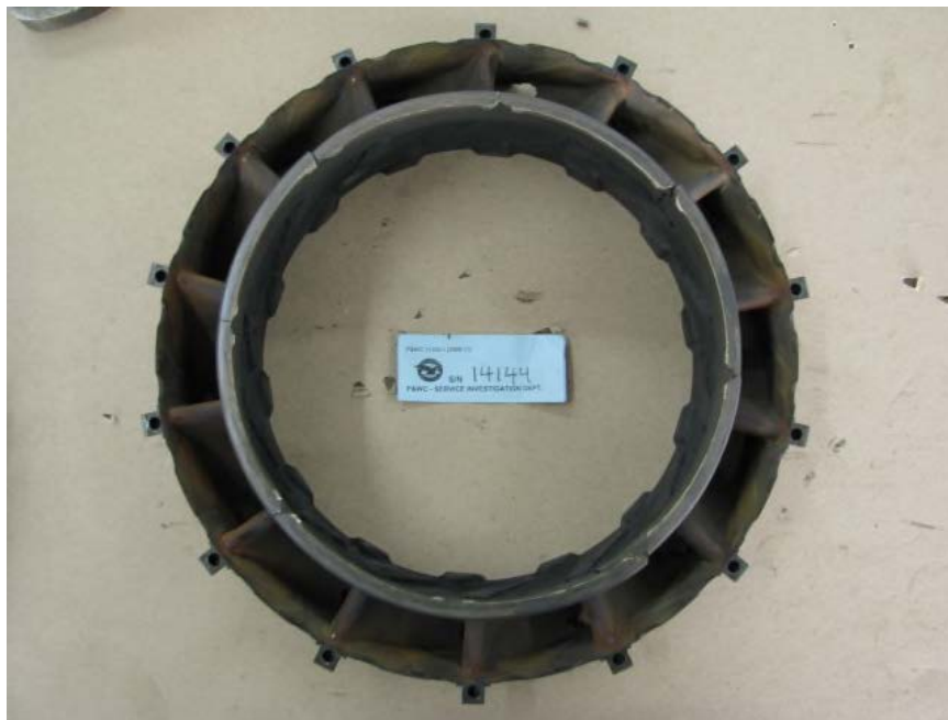
Photo No. 22 Compressor turbine stator upstream view
