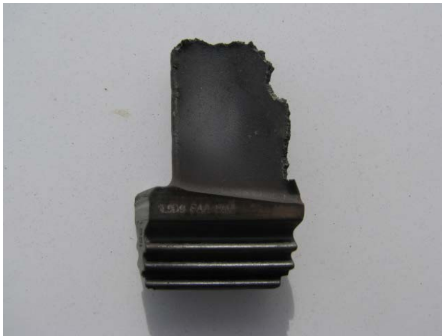
Photo No. 34 The removed compressor turbine blade showing P/N
