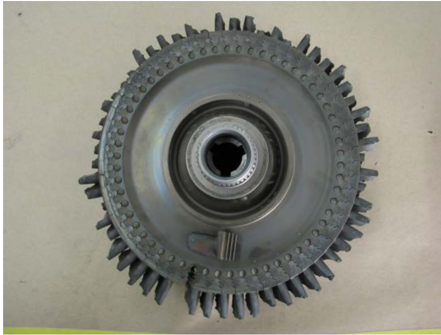
Photo No. 33 One compressor turbine blade removed from the disc
