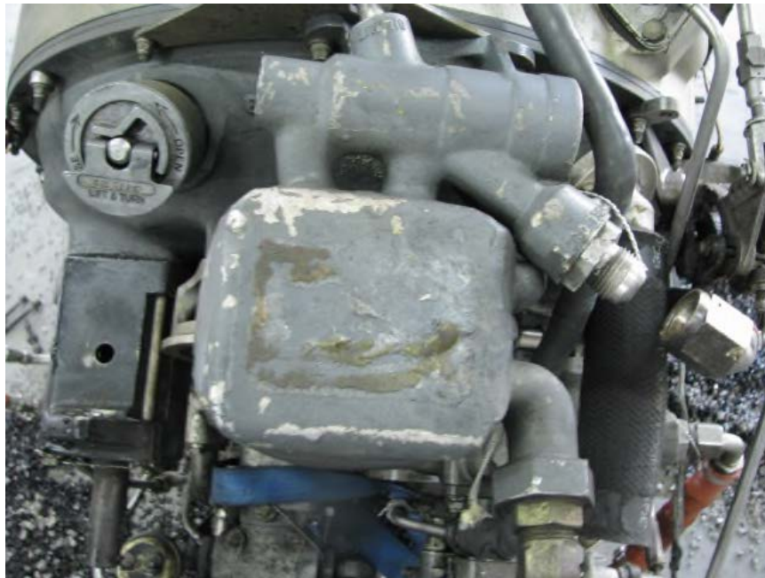
Photo No. 48 Fuel heater
