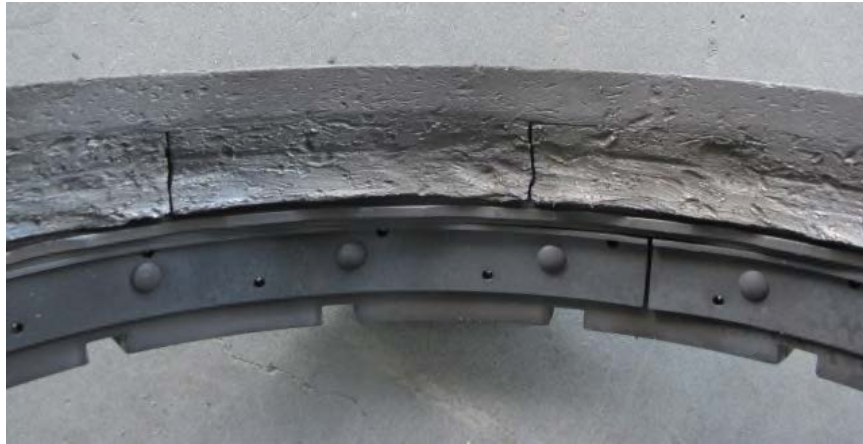
Photo No. 27 Compressor turbine shroud segments
