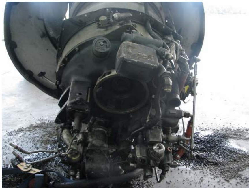
Photo No. 10 Accessories gearbox
