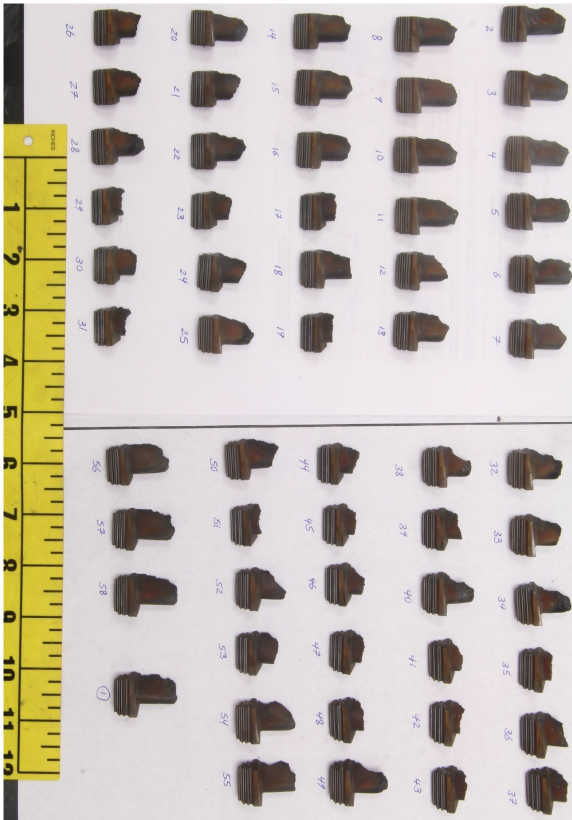
Figure 7 – The blades removed from the turbine wheel, labeled 2 through 58, along with Blade 1, viewed from the convex sides.
