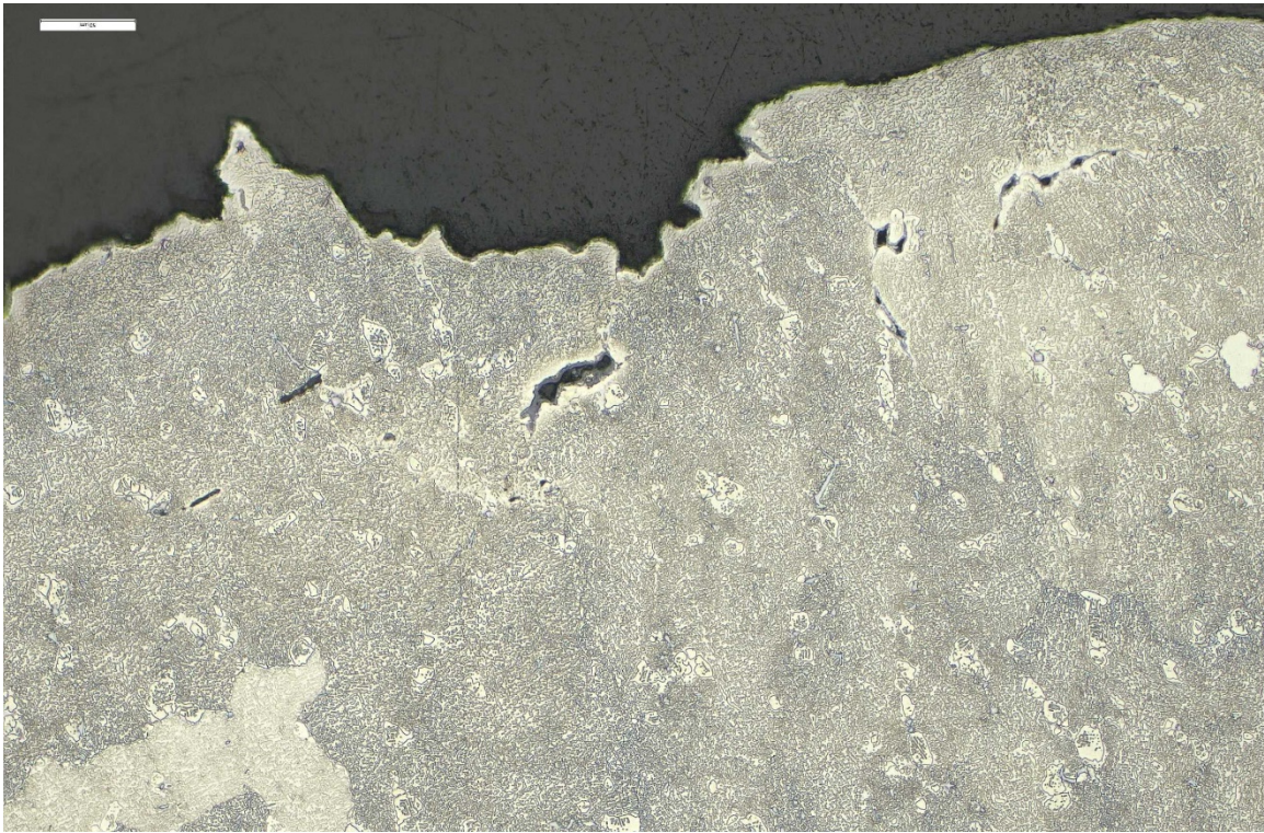
Figure 31 – Bright field (BF) micrograph of the microstructure at a cross section through the Blade 25 fracture surface (~200X, etched Marble's Reagent).
