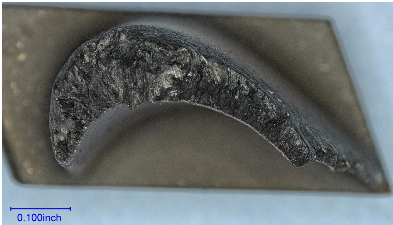
Figure 11 – The fracture surface of Blade 25.
