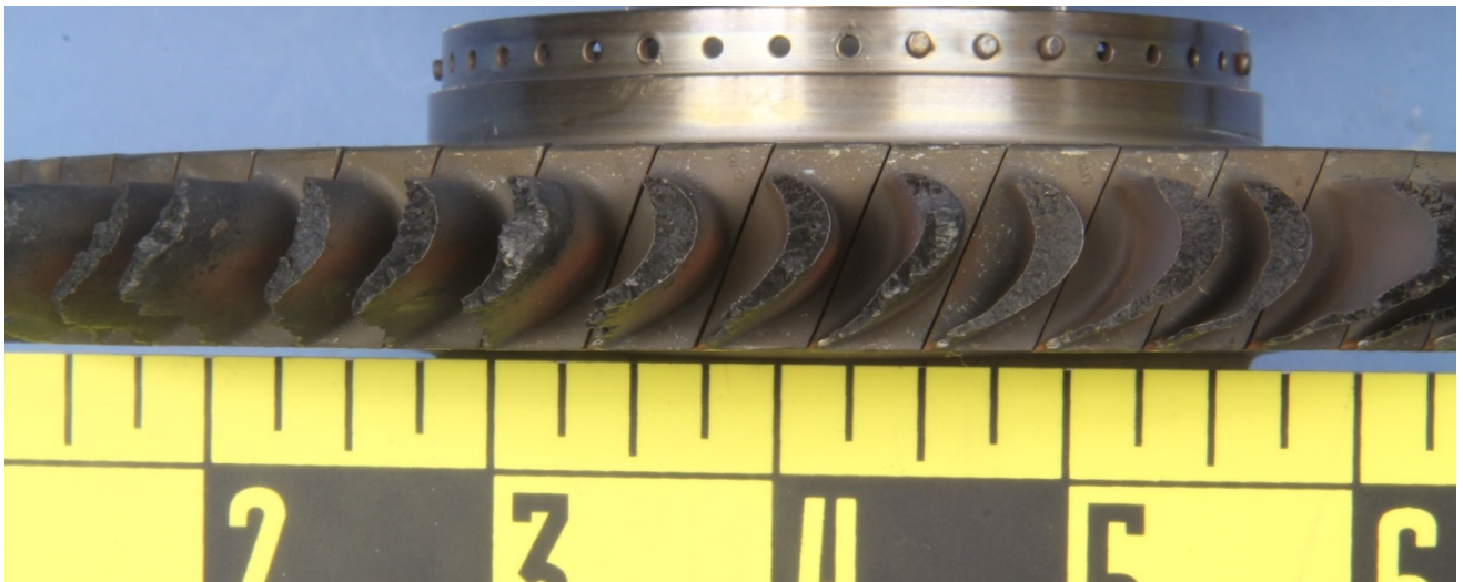
Figure A-8: The turbine wheel, as received, positioned to show the blade fracture surfaces.
