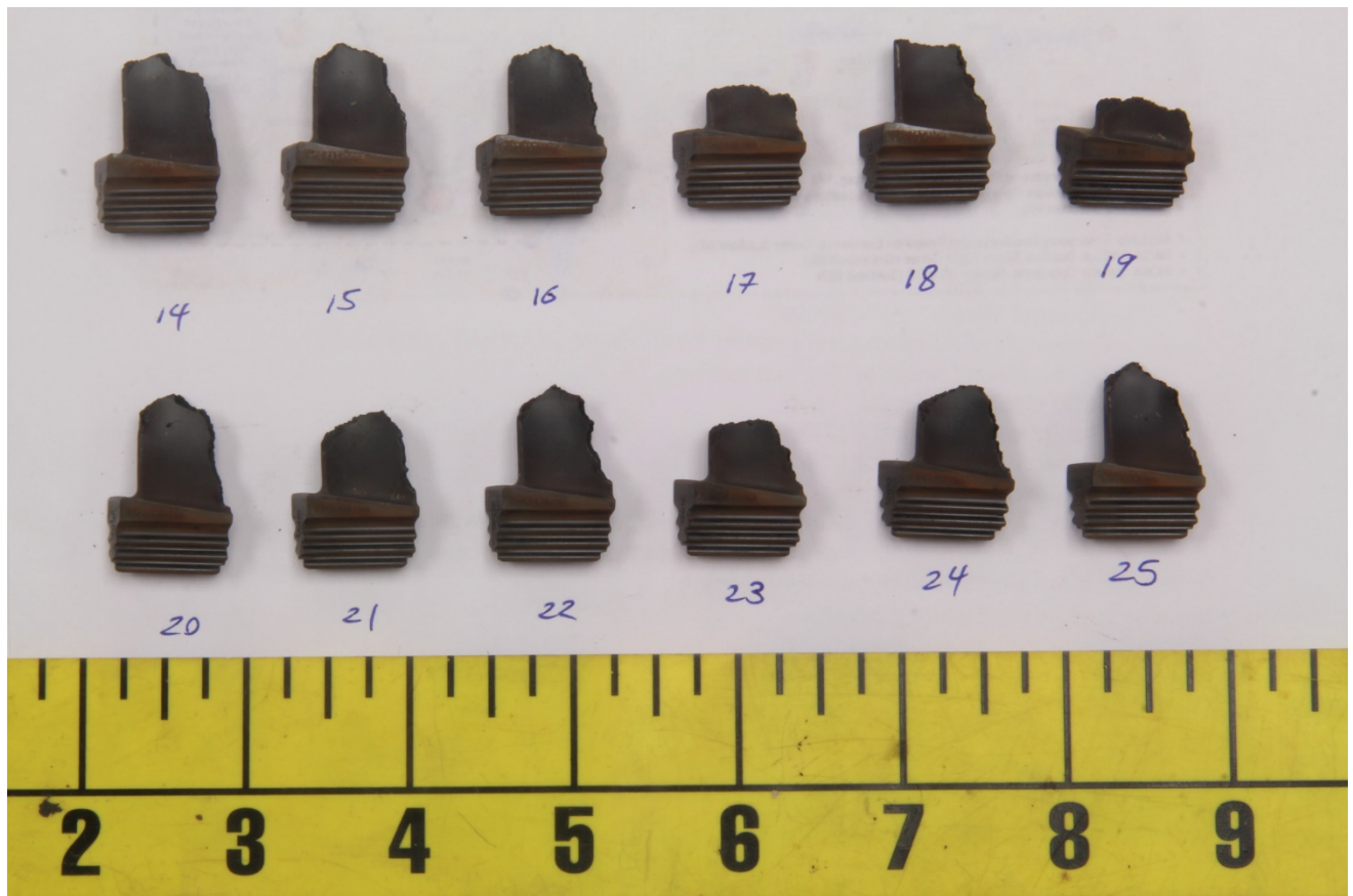
Figure B-8 – Fractured turbine blades 14 through 25, viewed from the concave side.
