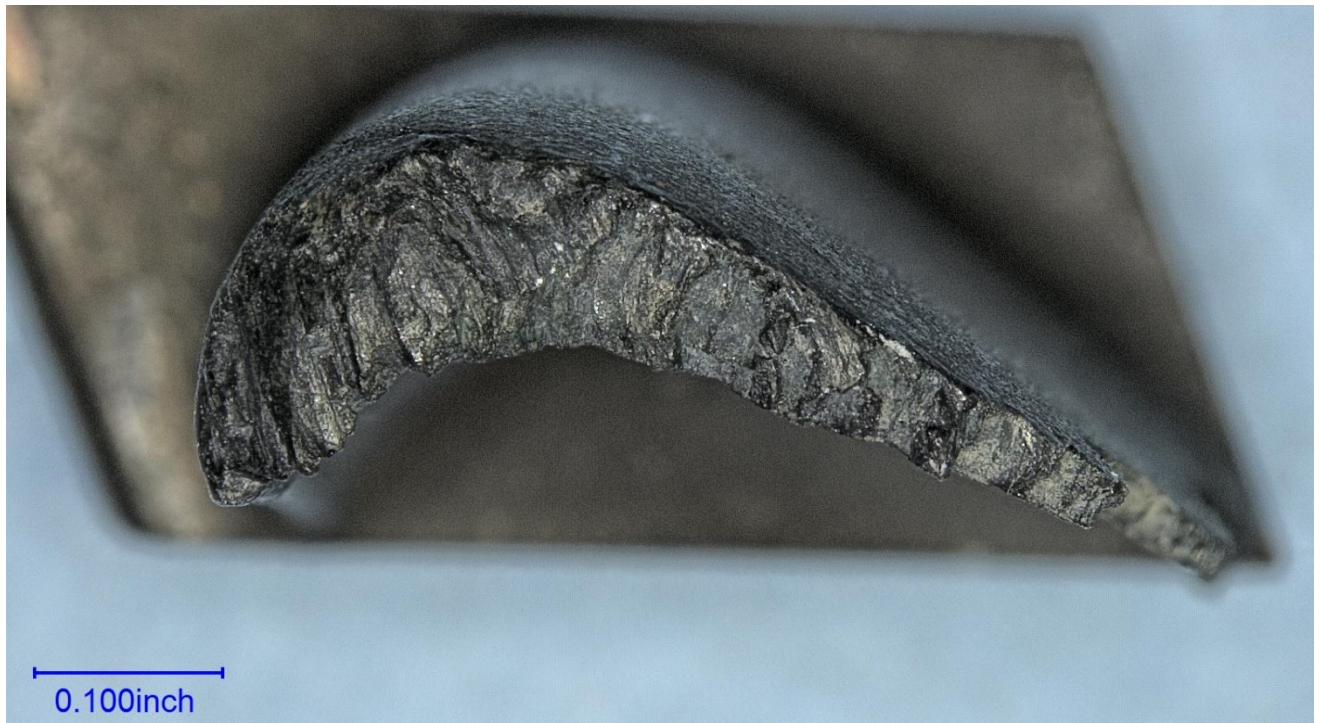
Figure 9 – The fracture surface of Blade 1.
