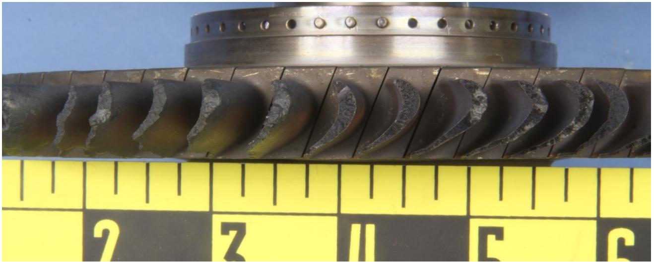
Figure A-11: The turbine wheel, as received, positioned to show the blade fracture surfaces.
