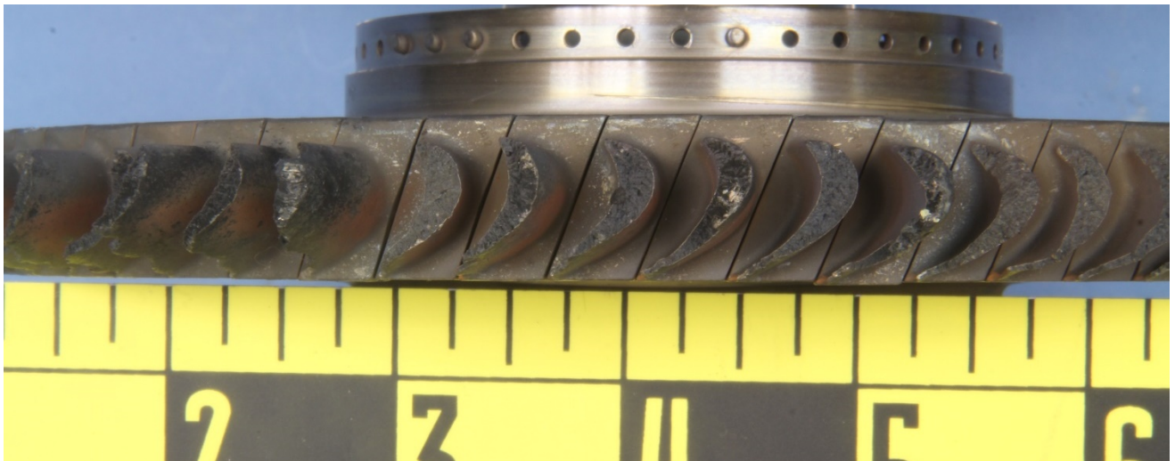
Figure A-6: The turbine wheel, as received, positioned to show the blade fracture surfaces.
