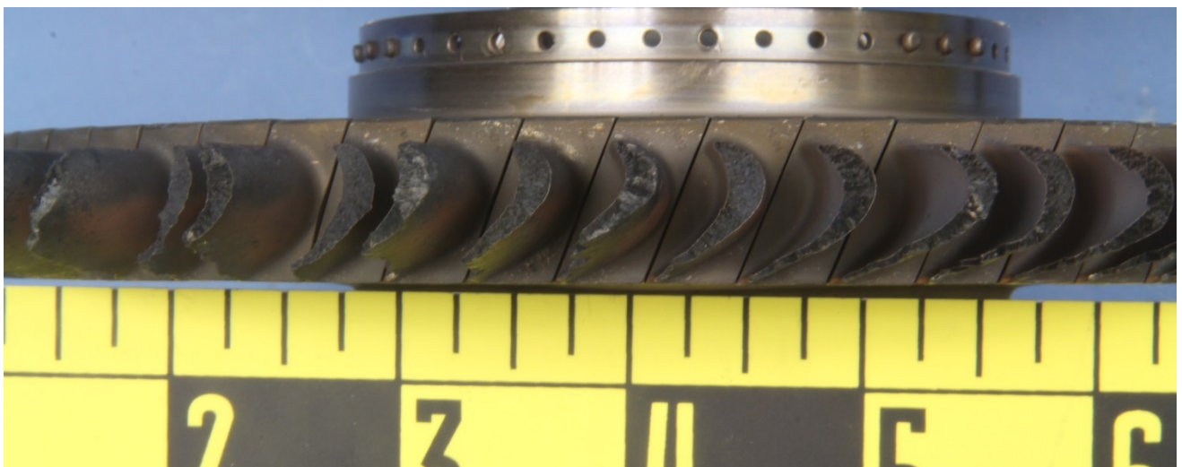
Figure A-9: The turbine wheel, as received, positioned to show the blade fracture surfaces.
