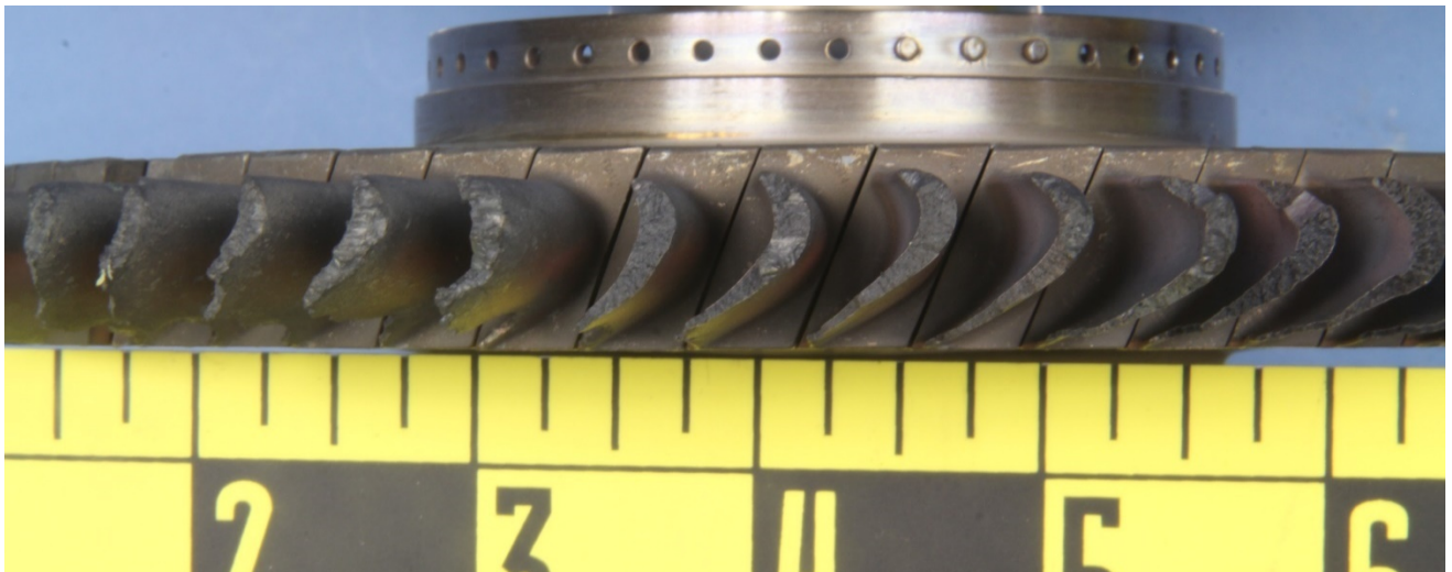
Figure A-12: The turbine wheel, as received, positioned to show the blade fracture surfaces.
