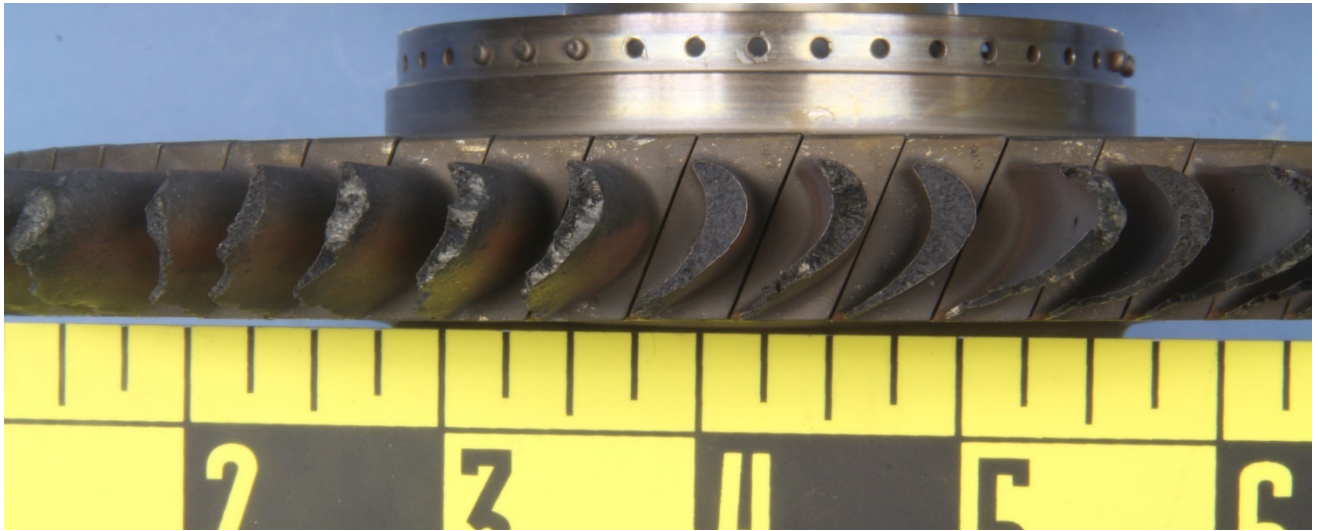
Figure A-10: The turbine wheel, as received, positioned to show the blade fracture surfaces.
