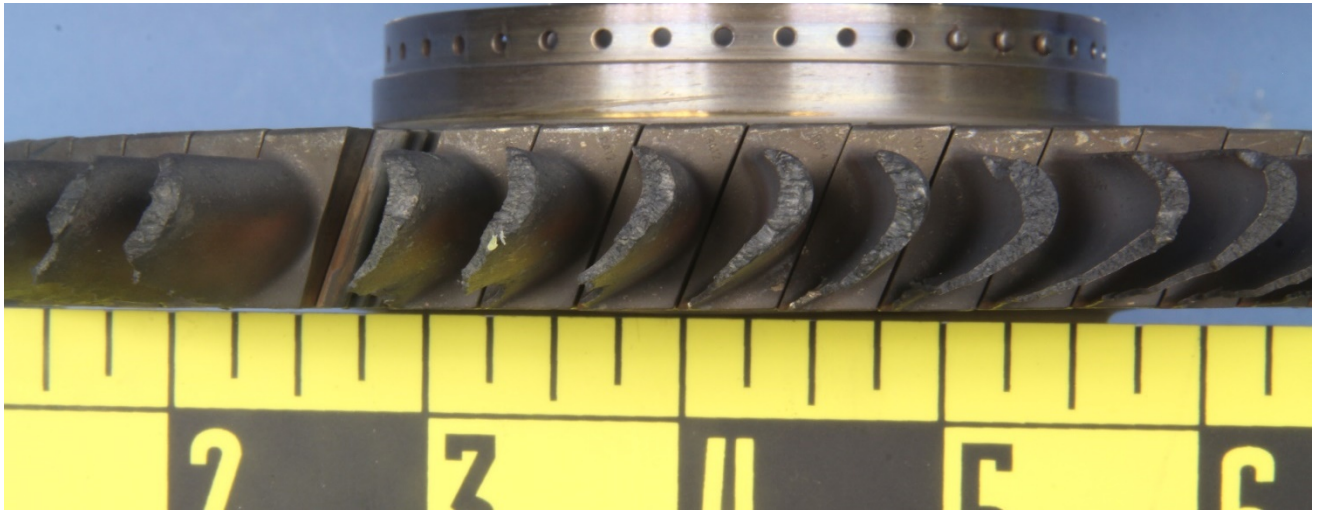
Figure A-13: The turbine wheel, as received, positioned to show the blade fracture surfaces.
