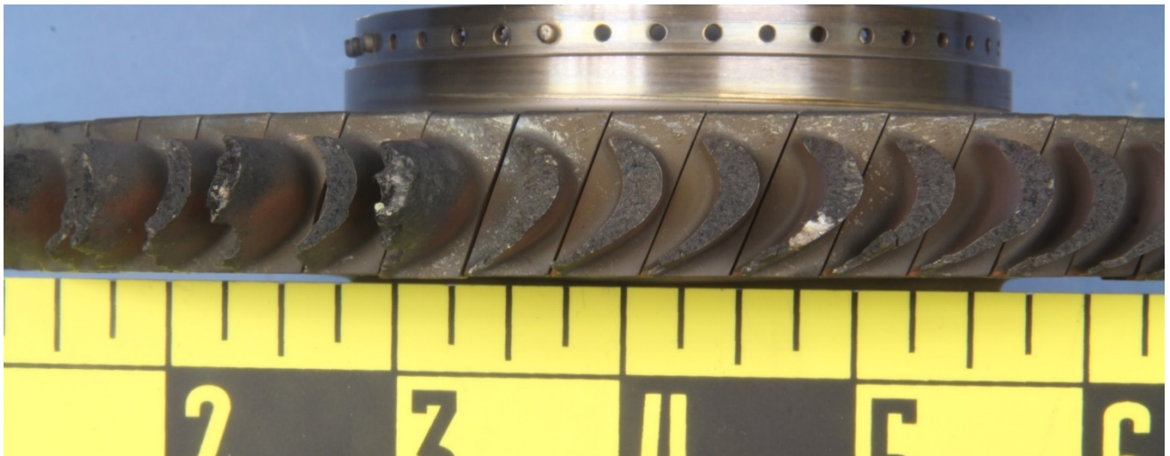
Figure A-5: The turbine wheel, as received, positioned to show the blade fracture surfaces.
