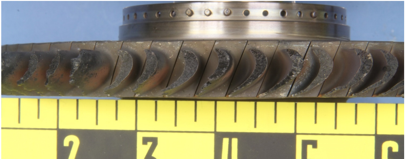
Figure A-7: The turbine wheel, as received, positioned to show the blade fracture surfaces.
