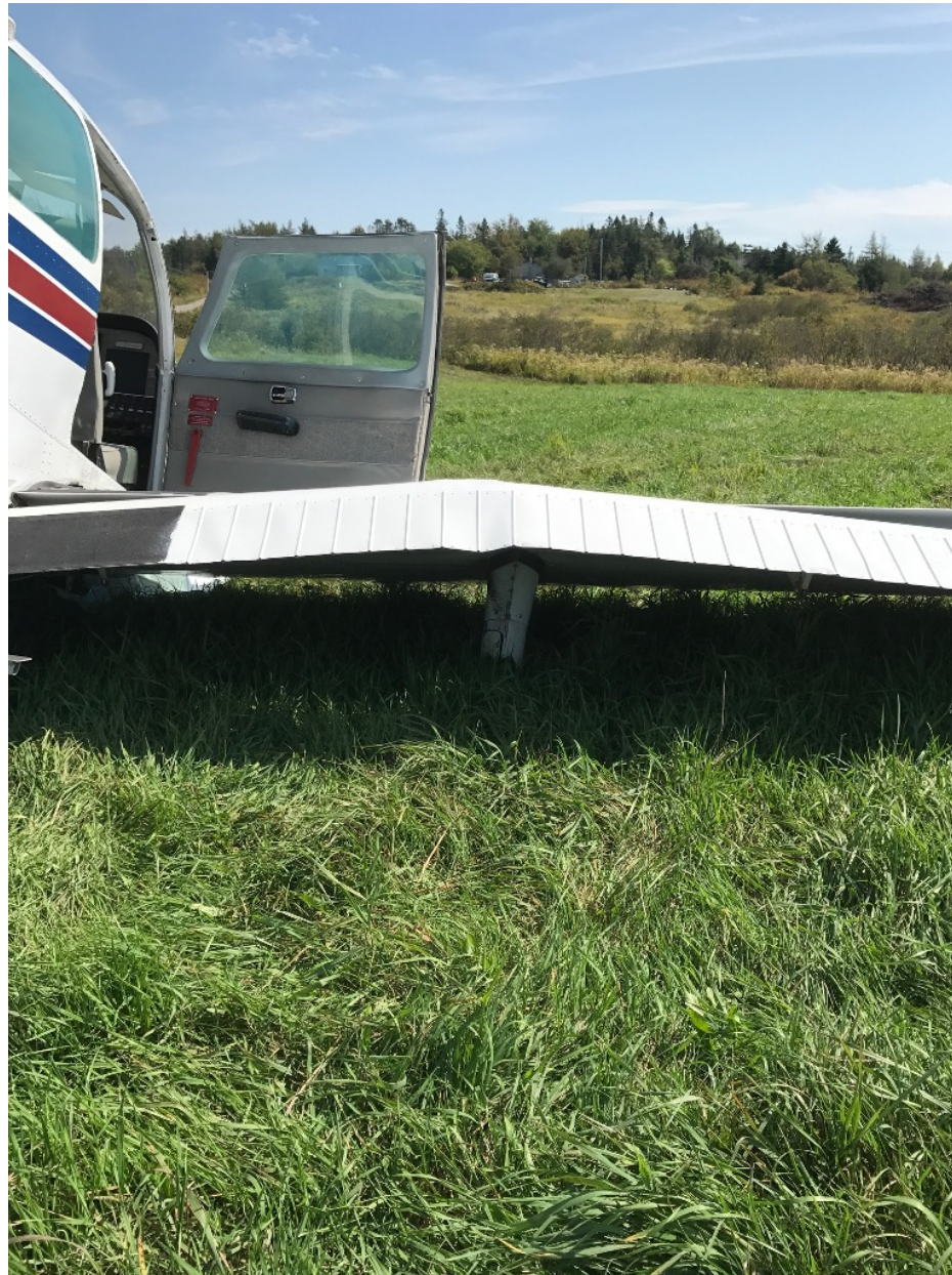
Photo 2 – Right Wing Damage (Photo Courtesy of FAA)
