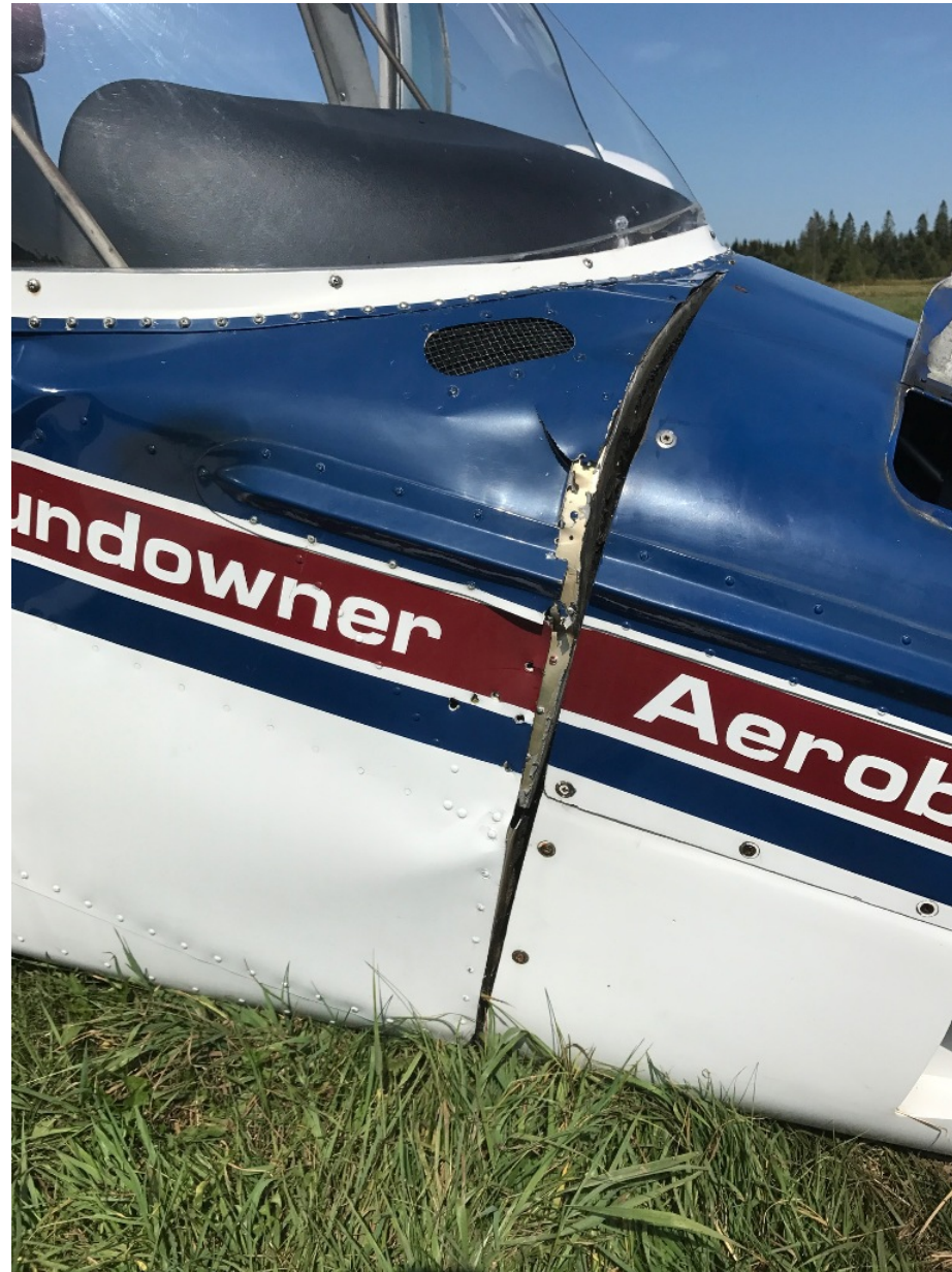
Photo 3 – Fuselage Damage (Photo Courtesy of FAA)
