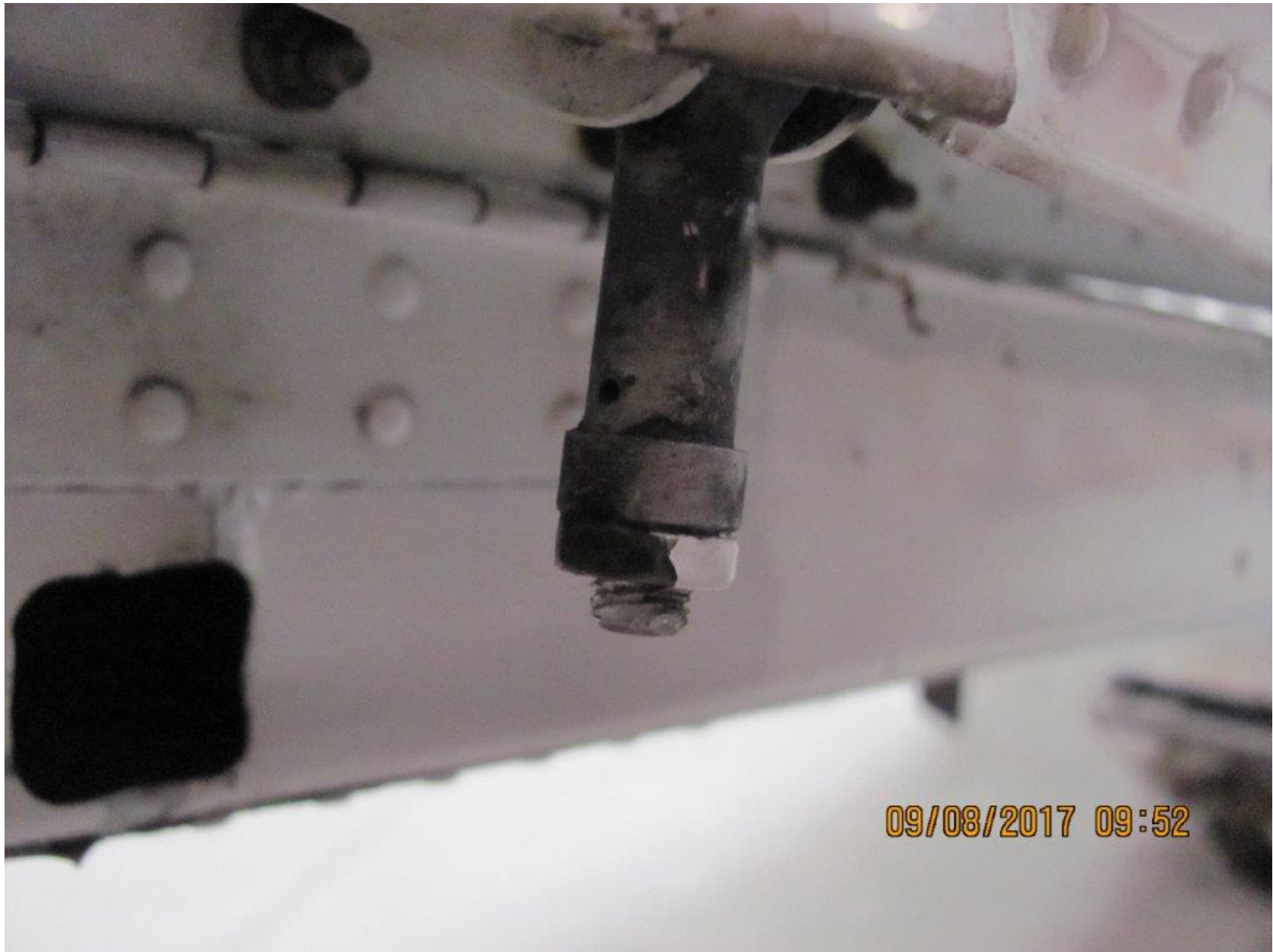
Photo 2 – View of Fractured Aileron Control Rod (State of Vermont)
