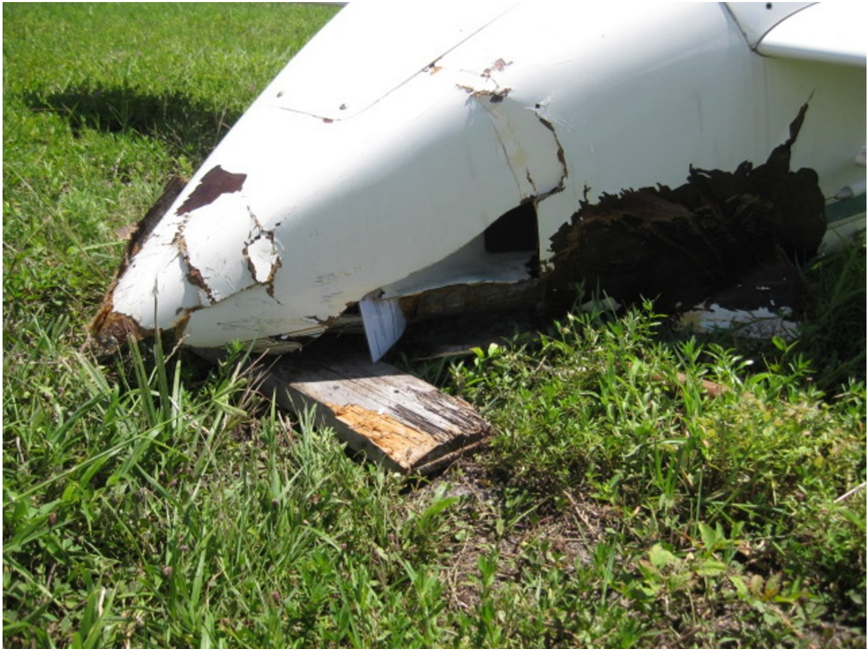
Photo 2 – Damage to the forward fuselage area
