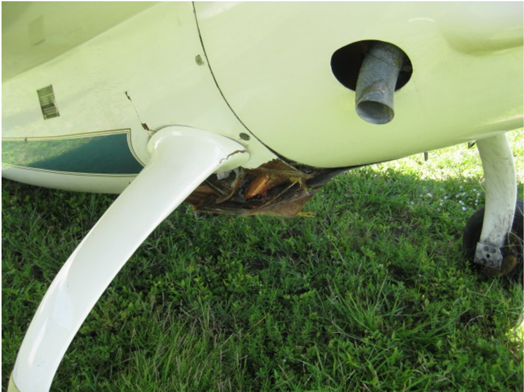
Photo 4 – Damage to lower fuselage
