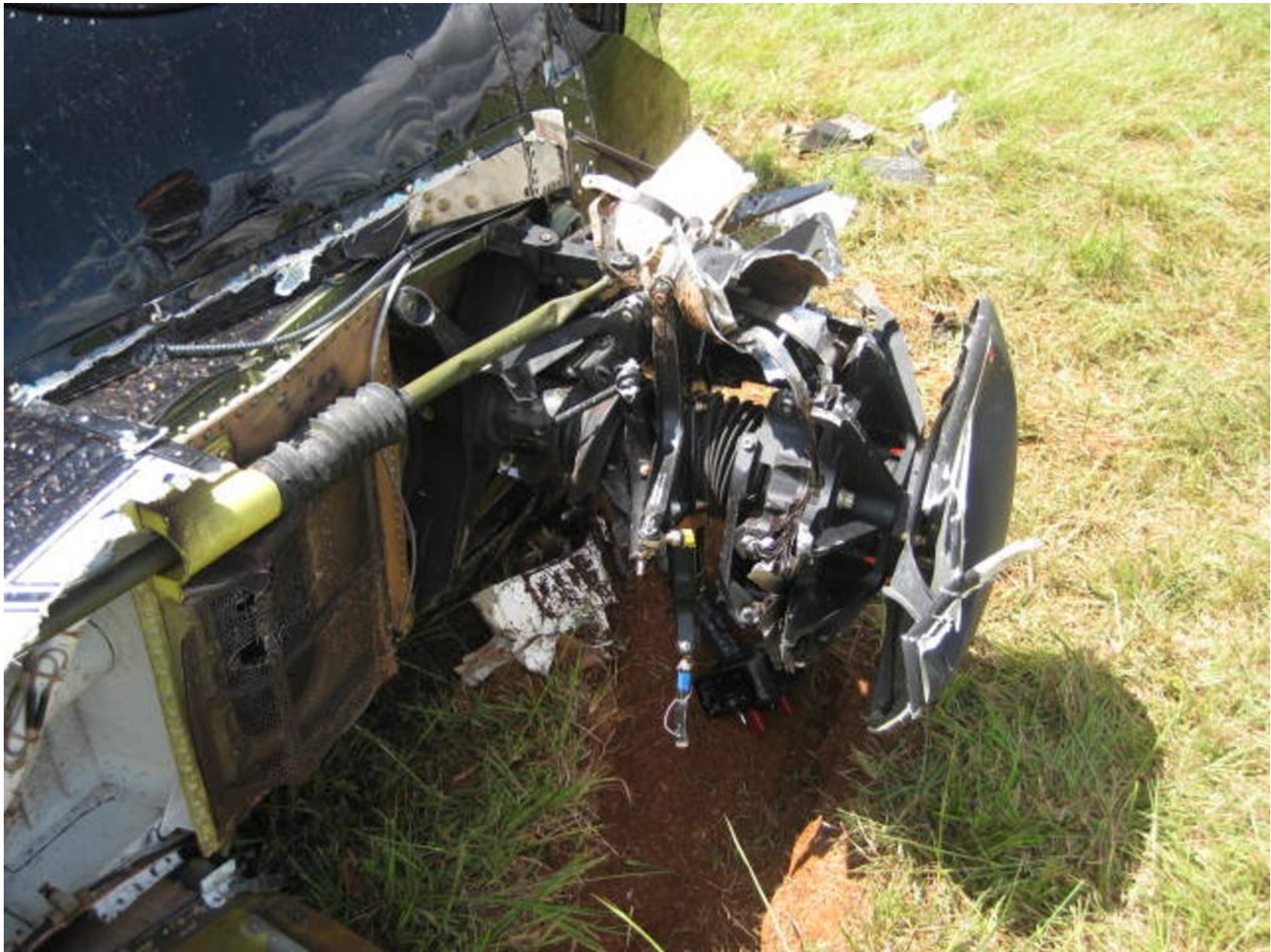
Photo 4 – Main Rotor Hub (FAA Photo)
