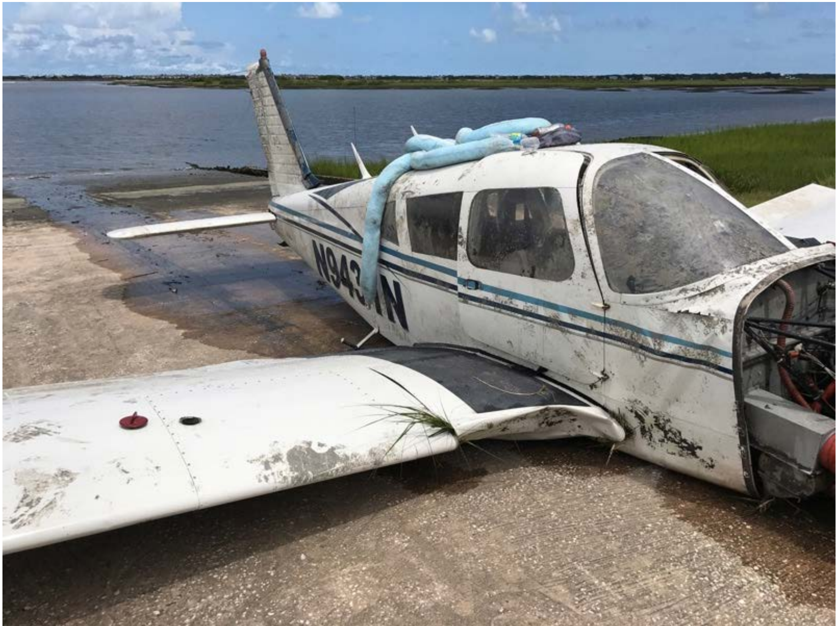
Photo 4 – View of right wing showing inboard buckling of leading edge and airframe (courtesy of FAA)
