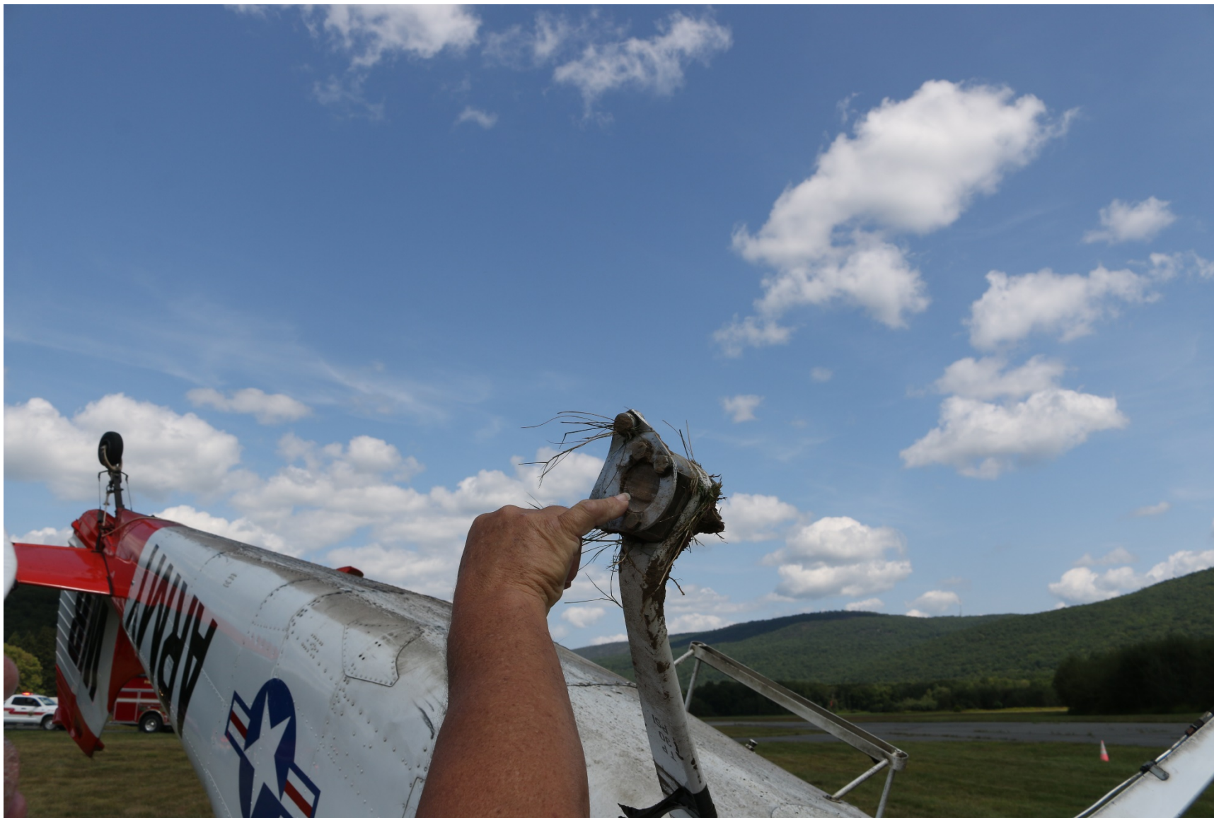
Photo 3 – View of Fractured Axle (Courtesy of FAA)
