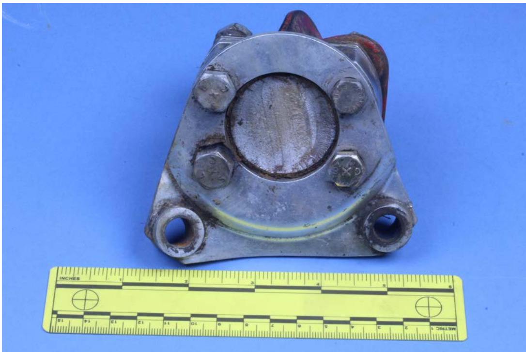
Figure 2: Portion of fractured axle shaft.
