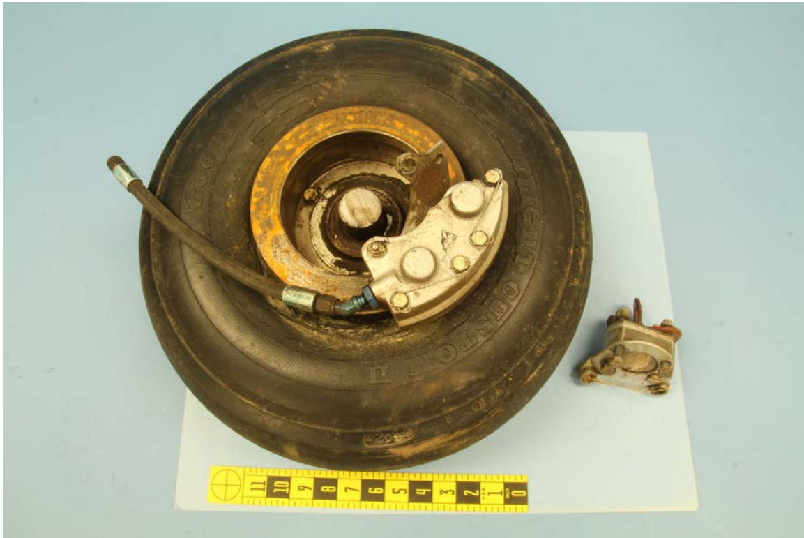
Figure 1: Left main landing gear wheel and axle assembly as received.
