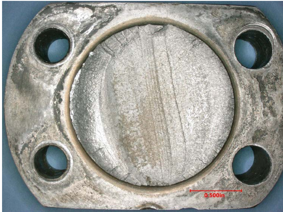
Figure 3: Axle shaft fracture surface exhibiting ratchet marks on the periphery and crack arrest fronts towards the middle.
